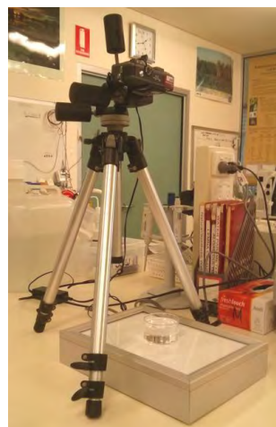
Figure A2 Set up of camera, tripod and light box for capturing surface area images
