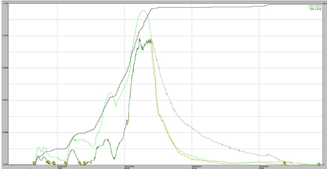
**Figure A1-16** Stage traces for EP1 and EP2 runoff events from 16-01-2014. Some 66 mm of rainfall occurred during the runoff periods and a total of 82 mm rain occurred in the 24-hour period before the end of rainfall.
