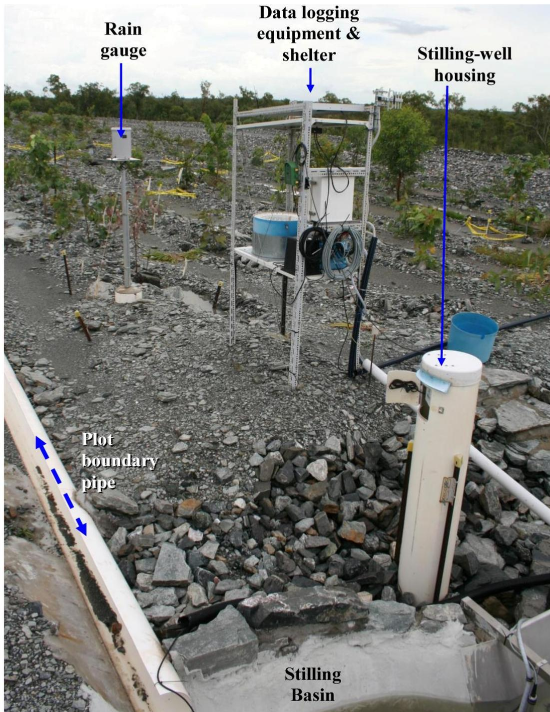
**Figure 4.** The location of the EP1 raingauge just right of the downstream plot boundary and in relation to other EP1 monitoring equipment: Data-logger and shelter; runoff stilling-basin; and stilling-well housing for the shaft encoder. Photo taken 19-01-2011.
