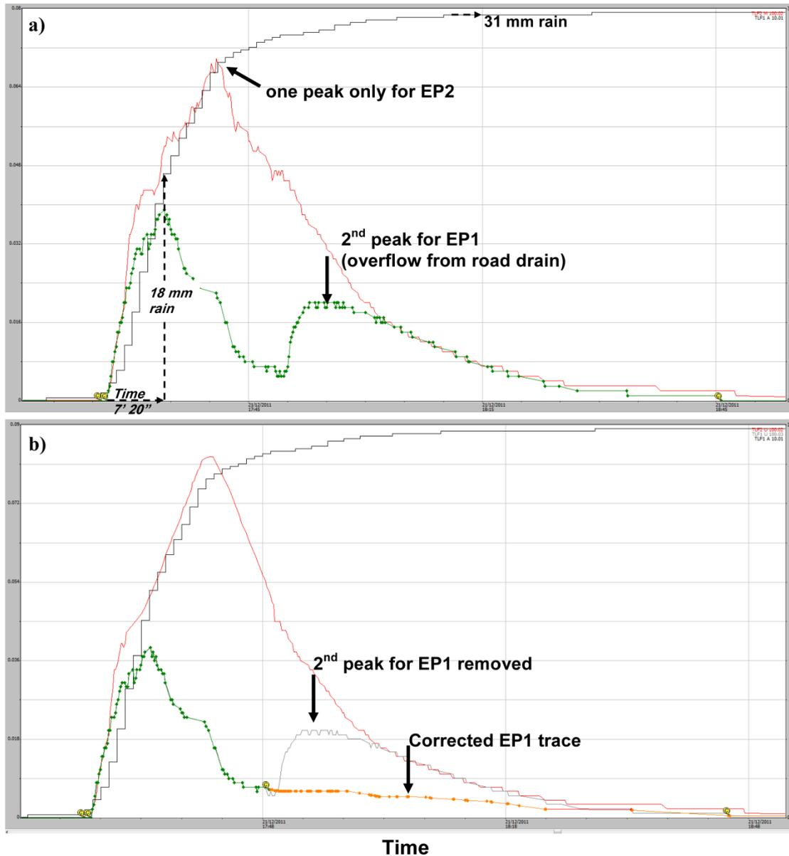
**Figure 6** Evidence and correction of roadside drain overflow event where: **a)** overflow is indicated by a 2<sup>nd</sup> peak in the EP1 trace after a brief yet intense 31 mm rain event on the 21<sup>st</sup> December 2011; and **b)** correction applied to abnormal records by manual editing (orange line).
