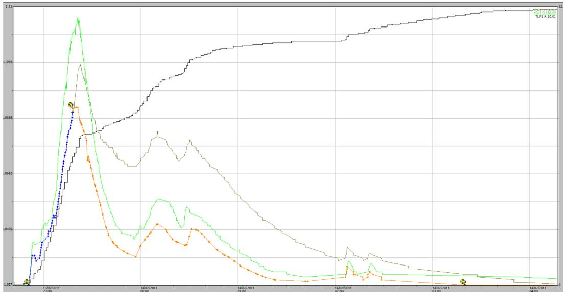
**Figure A1-4** Stage traces for an EP1 and EP2 runoff event on 14-02-2011. Some 63 mm of rainfall occurred during the runoff period and a total of 127 mm occurred in a 24-hour period from the end of rainfall.
