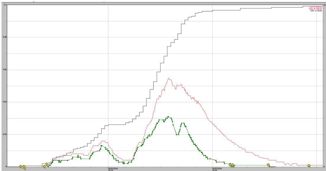
**Figure A1-47** 05/03/2014 (Plot1/2): 33 mm rain event (black) EP1 shaft encoder (green trace) EP2 shaft encoder (red trace). No boundary overflow problem indicated.
