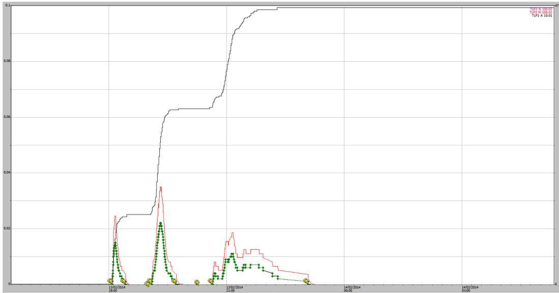
**Figure A1-44** 13/02/2014 (Plot1/2): 48 mm rain (black) over three runoff events. EP1 shaft encoder (green trace) EP2 shaft encoder (red trace). No overflow problem indicated.
