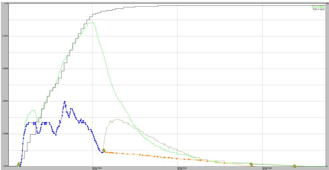
**Figure A1-9** Stage traces for an EP1 and EP2 runoff event on 08-02-2012. Some 40 mm of rainfall occurred during the runoff period and a total of 41 mm of rain occurred in the 24-hour period before the end of rainfall.
