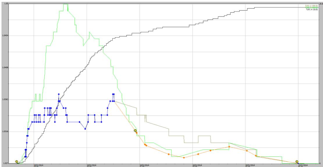
**Figure A1-17** Stage traces for EP1 and EP2 runoff events from 18-01-2014. Some 30 mm of rainfall occurred during the runoff periods and a total of 58 mm rain occurred in the 24-hour period before the end of rainfall.
