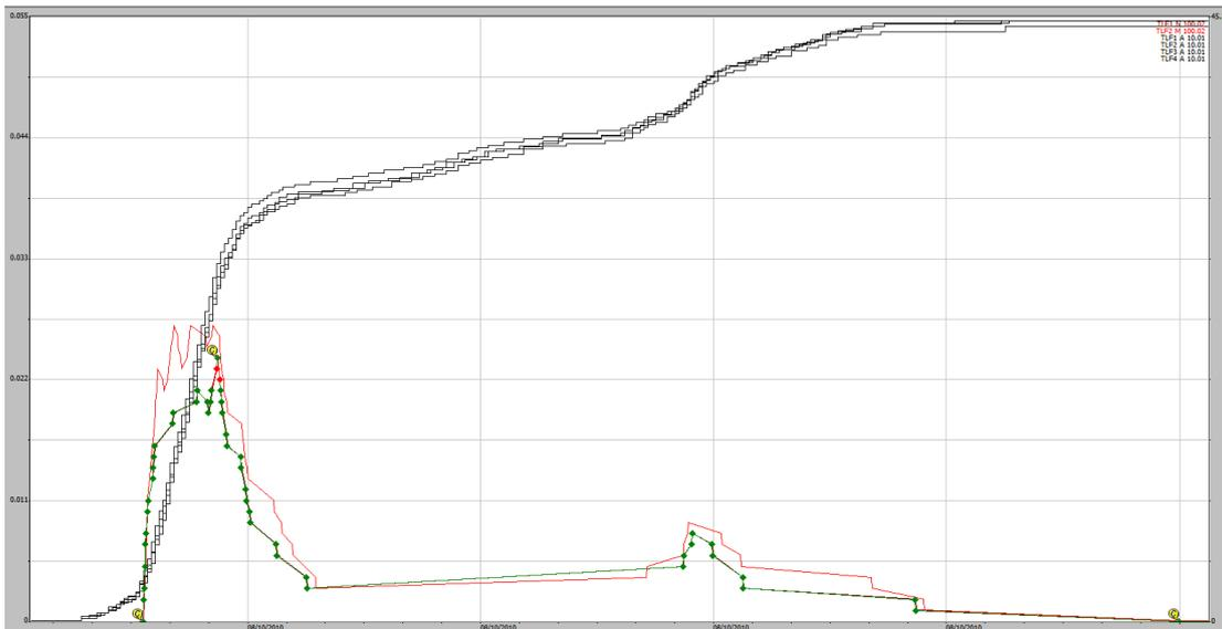
**Figure A1-29** 08/10/2010, 45 mm rain event (black traces for plots 1 to 4) EP1 shaft encoder (green trace) EP2 shaft encoder (red trace). No overflow problem indicated.
