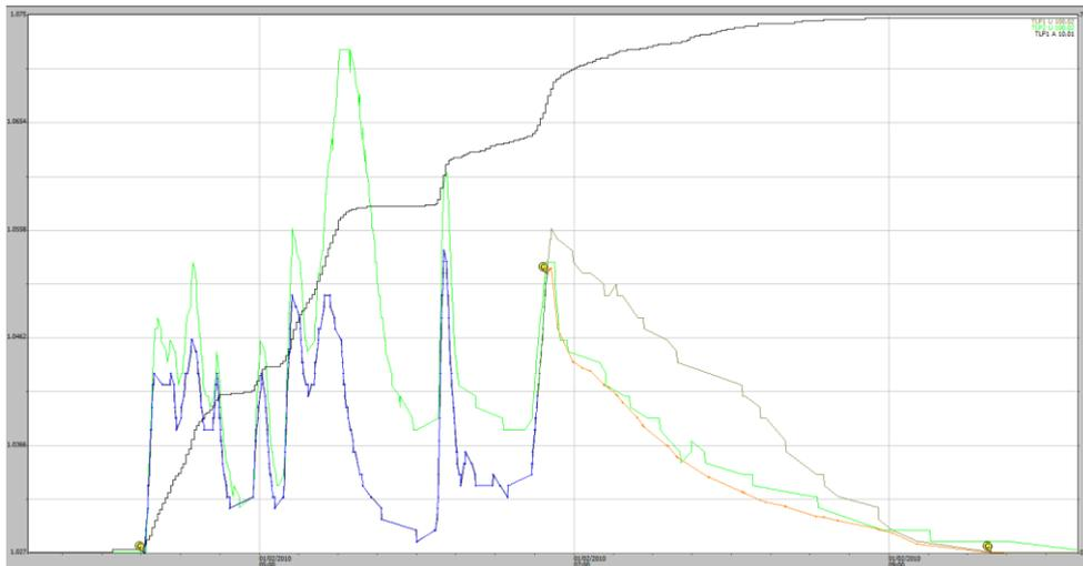
**Figure A1-1** Stage traces for an EP1 and EP2 runoff event on 01-02-2010 where some 76 mm of rainfall occurred during the runoff period this being the total amount occurring in a 24-hr period from the end of rainfall.
