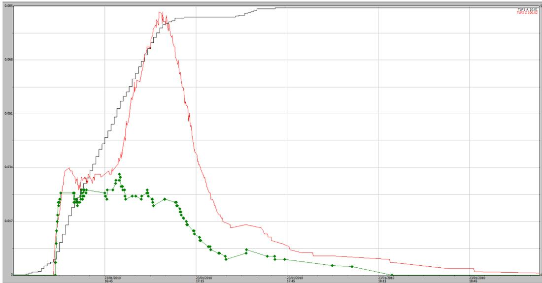
**Figure A1-24** 23/01/2010, 58 mm rain event (black trace) EP1 shaft encoder (green trace) EP2 shaft encoder (red trace). No overflow problem indicated.
