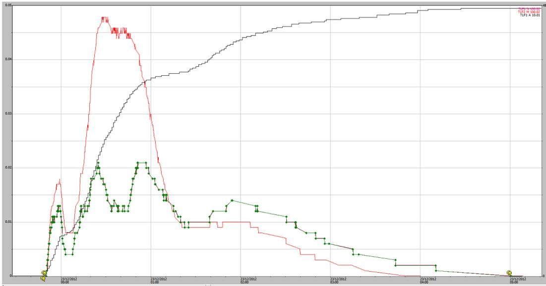
**Figure A1-38** 23/12/2012, 48 mm rain event (black) EP1 shaft encoder (green trace) EP2 shaft encoder (red trace). No overflow problem indicated.
