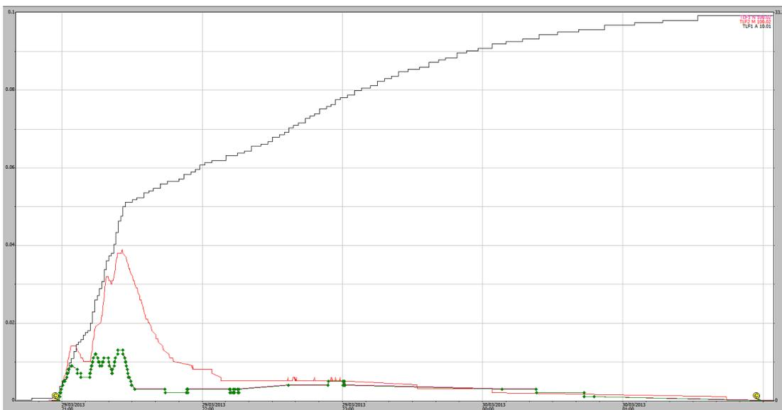
**Figure A1-39** 29/03/2013, 33 mm rain event (black) EP1 shaft encoder (green trace) EP2 shaft encoder (red trace). No overflow problem indicated.
