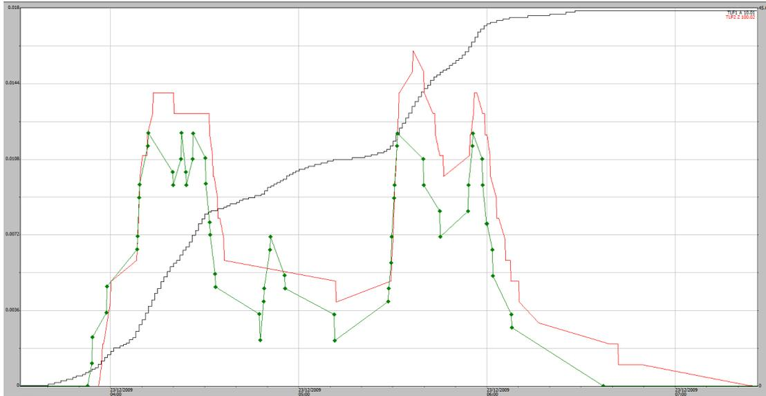
**Figure A1-22** 23/12/2009, 46 mm rain event in about 2 ½ hours (black trace) EP1 shaft encoder (green trace) EP2 shaft encoder (red trace). No overflow problem indicated.
