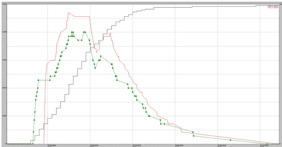
**Figure A1-25** 27/01/2010, 30 mm rain event (black trace) EP1 shaft encoder (green trace) EP2 shaft encoder (red trace). No overflow problem indicated.
