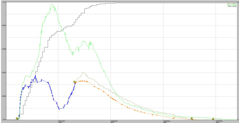
**Figure A1-2** Stage traces for an EP1 and EP2 runoff event on 13-02-2011 where some 48 mm of rainfall occurred during the runoff period with 64 mm occurring in a 24-hr period from the end of rainfall.
