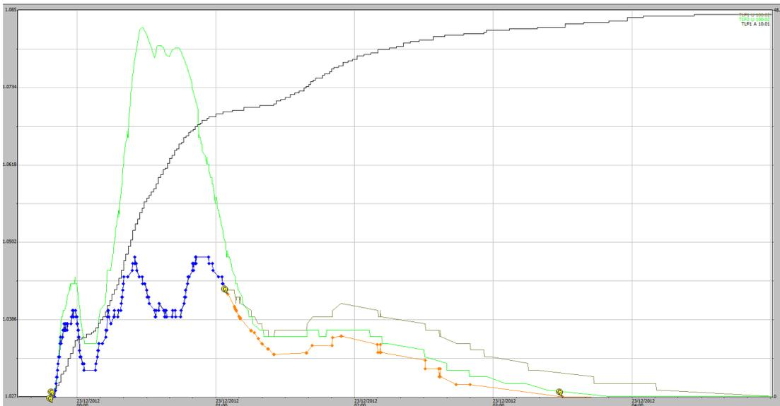
**Figure A1-11** Stage traces for an EP1 and EP2 runoff event on 23-12-2012. Some 48 mm of rainfall occurred during the runoff period and a total of 77 mm of rain occurred in the 24-hour period before the end of rainfall.
