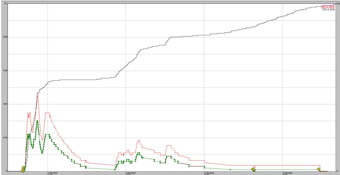
**Figure A1-46** 18/02/2014 (Plot1/2): 37 mm rain event (black) EP1 shaft encoder (green trace) EP2 shaft encoder (red trace). No boundary overflow problem indicated.
