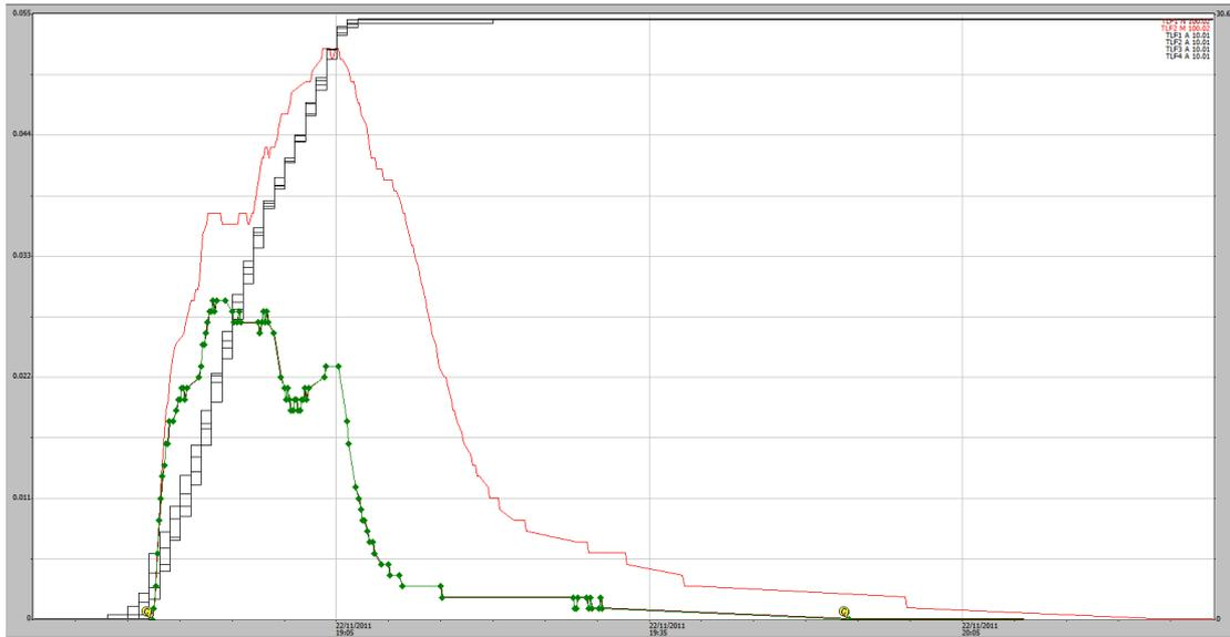
**Figure A1-32** 22/11/2011, 30 mm rain event (black traces for plots 1 to 4). EP1 shaft encoder (green trace) EP2 shaft encoder (red trace). No overflow problem indicated.
