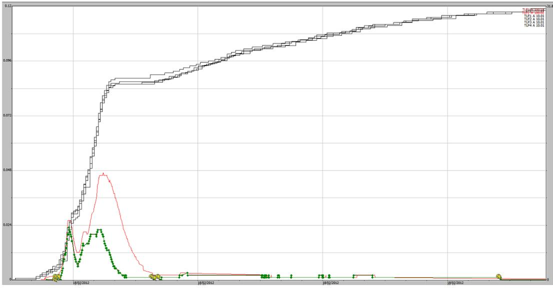
**Figure A1-35** 18/02/2012, 32 mm rain event (rising black traces, plots 1 to 4) EP1 shaft encoder (green trace) EP2 shaft encoder (red trace). No overflow problem indicated.
