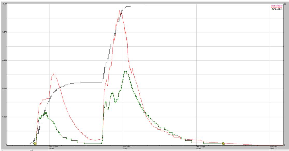
**Figure A1-37** 18/12/2012, 56 mm rain (black) over two runoff events. EP1 shaft encoder (green trace) EP2 shaft encoder (red trace). No overflow problem indicated.
