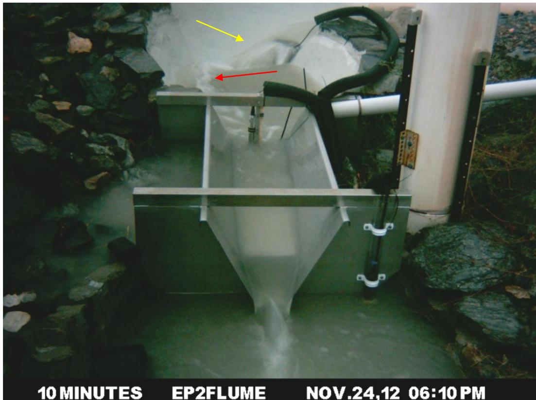
**Figure 5** Example of water-level disturbance in the upstream stilling basin at EP2 during the peak of a high-flow event. The flow can be seen deflecting off the cage (yellow arrow) and can be seen rising up around the outside of the basin (red arrow).
