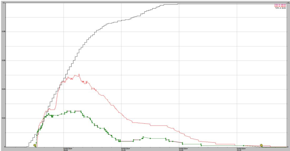
**Figure A1-50** 03/05/2014, 46 mm rain event (black) EP1 shaft encoder (green trace) EP2 shaft encoder (red trace). No boundary overflow problem indicated.
