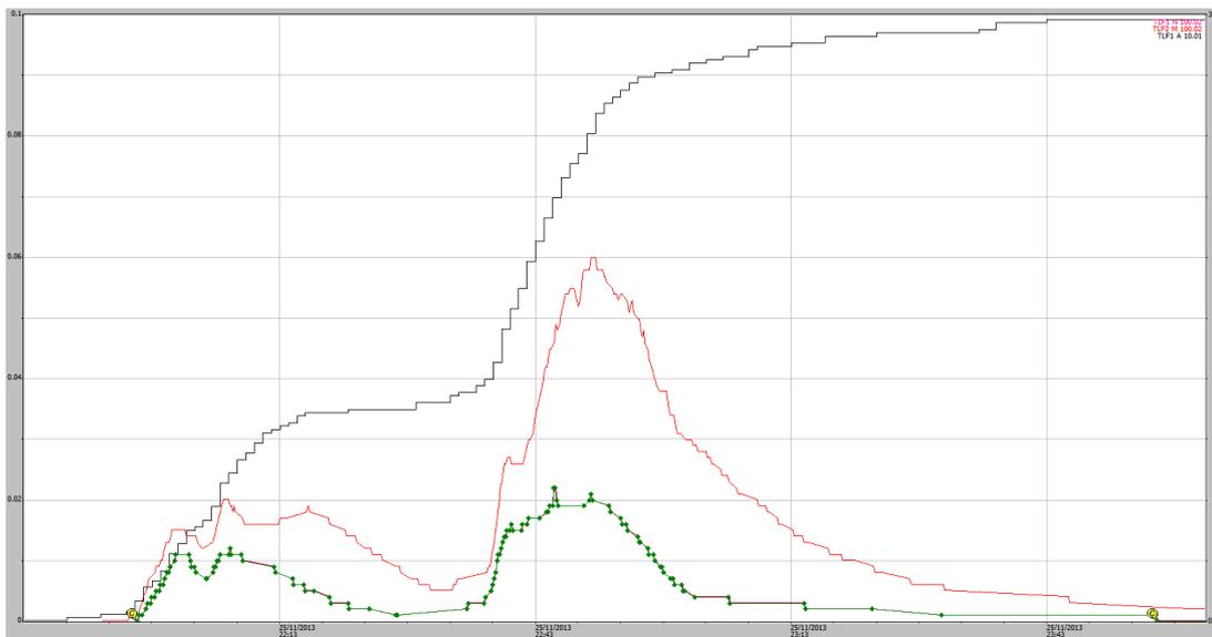
**Figure A1-41** 25/11/2013, 36 mm rain event (black) EP1 shaft encoder (green trace) EP2 shaft encoder (red trace). No overflow problem indicated.
