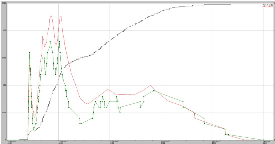
**Figure A1-31** 27/03/2011, 53 mm rain event (black) EP1 shaft encoder (green trace) EP2 shaft encoder (red trace). Marginal overflow problem indicated on recession but no correction applied.
