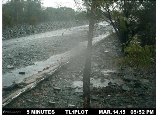
**Figure A2-7** EP1 stage trace for a 1.6 mm rain event from 5:22 to 5:26 PM on the 14-03-2015 and photo of the adjacent roadside drain showing peak runoff at 5:26 PM with no plot boundary overflow.
