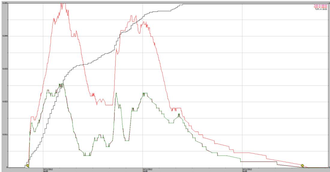
**Figure A1-36** 23/11/2012, 55 mm rain event (black) EP1 shaft encoder (green trace) EP2 shaft encoder (red trace). No overflow problem indicated.
