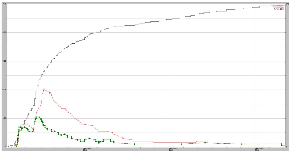
**Figure A1-43** 26/01/2014, 39 mm rain event (black) EP1 shaft encoder (green trace) EP2 shaft encoder (red trace). No overflow problem indicated.
