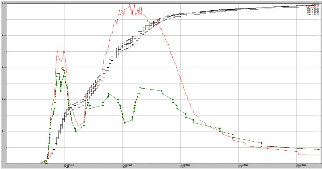
**Figure A1-30** 09/10/2010, 69 mm rain (black traces for plots 1 to 4). EP1 shaft encoder (green trace) EP2 shaft encoder (red trace). Marginal overflow detected at end of recession period. Perhaps could be corrected but has been left at this stage. The multimodal peaks on the EP1 stage trace correspond to changes in rain intensity.
