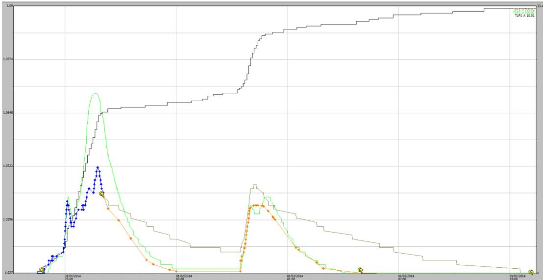
**Figure A1-20** Stage traces for EP1 and EP2 runoff events from 31-01-2014. Some 33 mm of rainfall occurred during the runoff periods and a total of 83 mm rain occurred in the 24-hour period before the end of rainfall.
