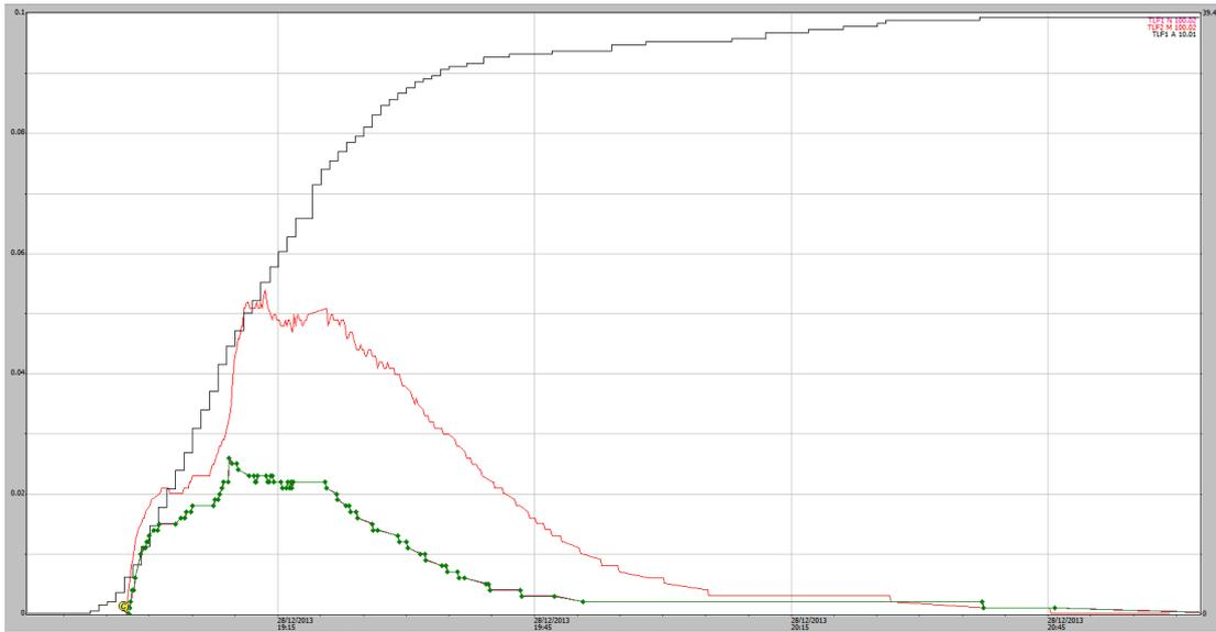
**Figure A1-42** 28/12/2013, 39 mm rain event (black) EP1 shaft encoder (green trace) EP2 shaft encoder (red trace). No overflow problem indicated.
