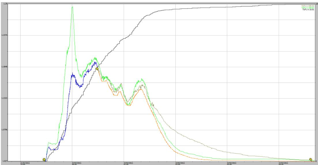
**Figure A1-5** Stage traces for an EP1 and EP2 runoff event on 22-02-2011. Some 180 mm of rainfall occurred during the runoff period and a total of 195 mm occurred in a 24-hour period from the end of rainfall.
