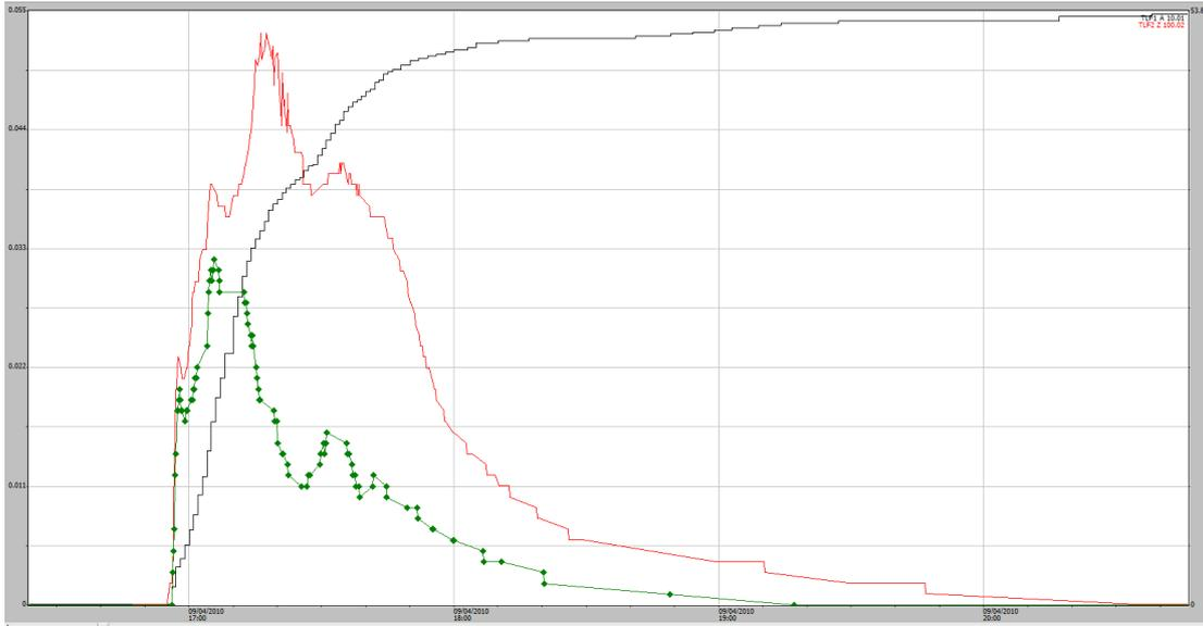
**Figure A1-26** 09/04/2010, 53 mm rain event (black trace) EP1 shaft encoder (green trace) EP2 shaft encoder (red trace). No overflow problem indicated.
