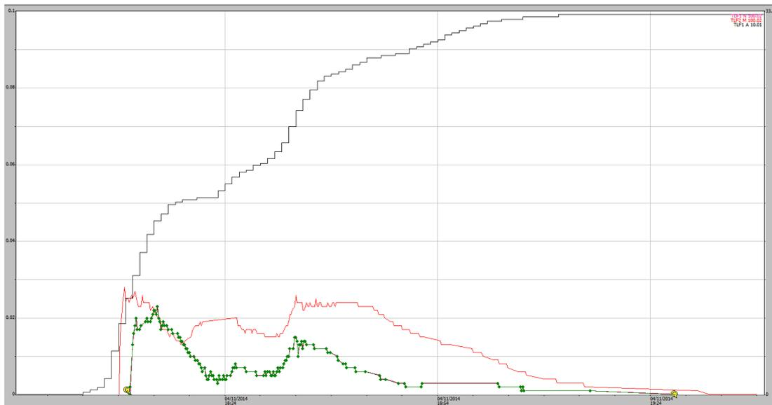
**Figure A1-51** 04/11/2014, 33 mm rain event (black) EP1 shaft encoder (green trace) EP2 shaft encoder (red trace). No boundary overflow problem indicated.
