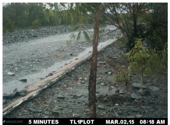
**Figure A2-5** EP1 stage trace for a 2.6 mm rain event from 6:20 to 9:51 am on the 02-03-2015 and photo of the adjacent roadside drain showing peak runoff at 8:18 am with no plot boundary overflow.
