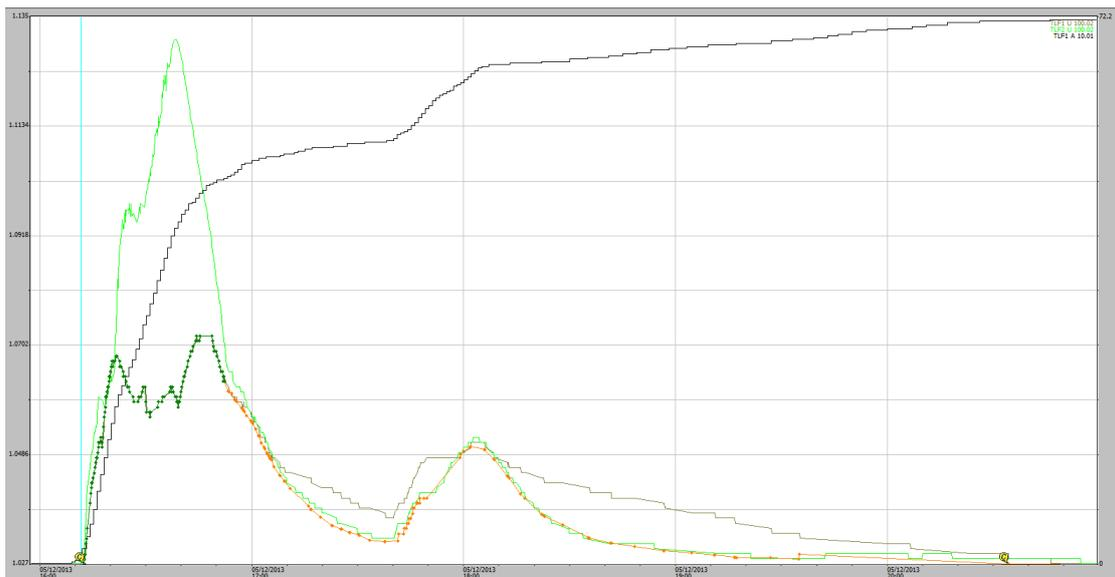
**Figure A1-15** Stage traces for EP1 and EP2 runoff events from 05-12-2013. Some 72 mm of rainfall occurred during the runoff periods and a total of 77 mm rain occurred in the 24-hour period before the end of rainfall.
