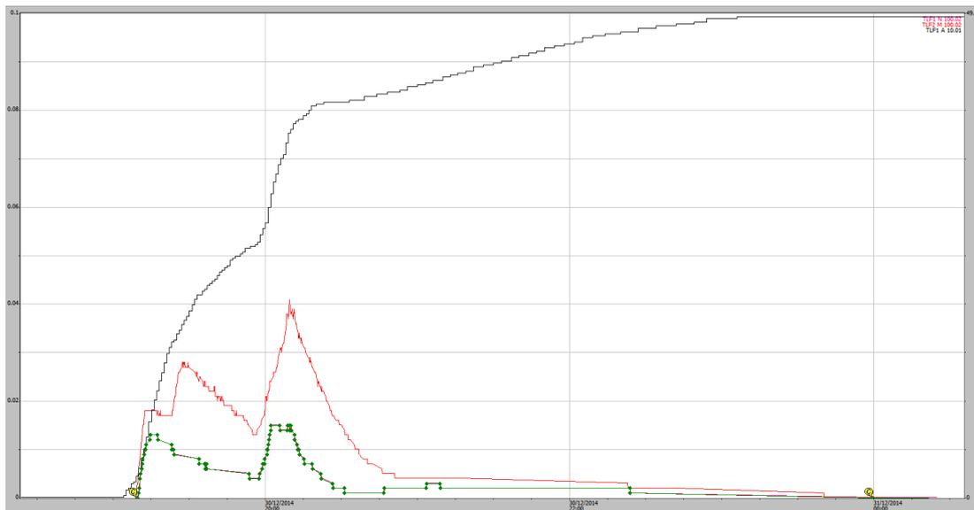
**Figure A1-53.** 30/12/2014, 50 mm rain event (black) EP1 shaft encoder (green trace) EP2 shaft encoder (red trace). No boundary overflow problem indicated.
