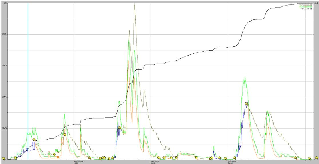
**Figure A1-14** Stage traces for EP1 and EP2 runoff events from 30-03-2013. Some 170 mm of rainfall occurred during the runoff periods and a total of 187 mm rain occurred in the 24-hour period before the end of rainfall.
