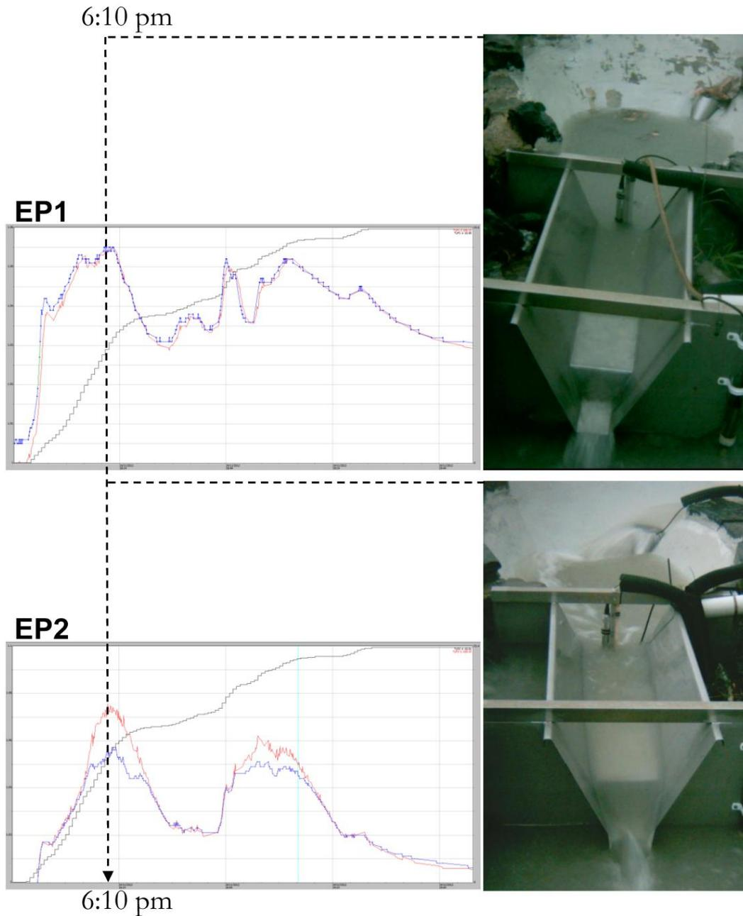
**Figure 15** EP1 (Blue) and EP2 (red) stage traces and corresponding time-lapse photos at peak of runoff event during some 54 mm of rainfall over 1 ½ hours on 24/11/2012.
