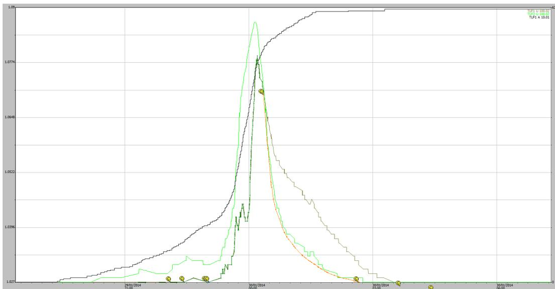
**Figure A1-19** Stage traces for EP1 and EP2 runoff events from 29-01-2014. Some 63 mm of rainfall occurred during the runoff periods and a total of 75 mm rain occurred in the 24-hour period before the end of rainfall.
