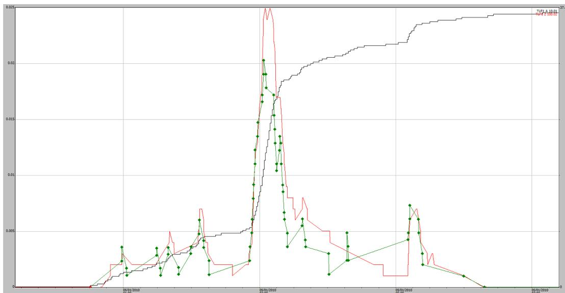
**Figure A1-23** 05/01/2010, 37 mm rain event (black trace) EP1 shaft encoder (green trace) EP2 shaft encoder (red trace). No overflow problem indicated.
