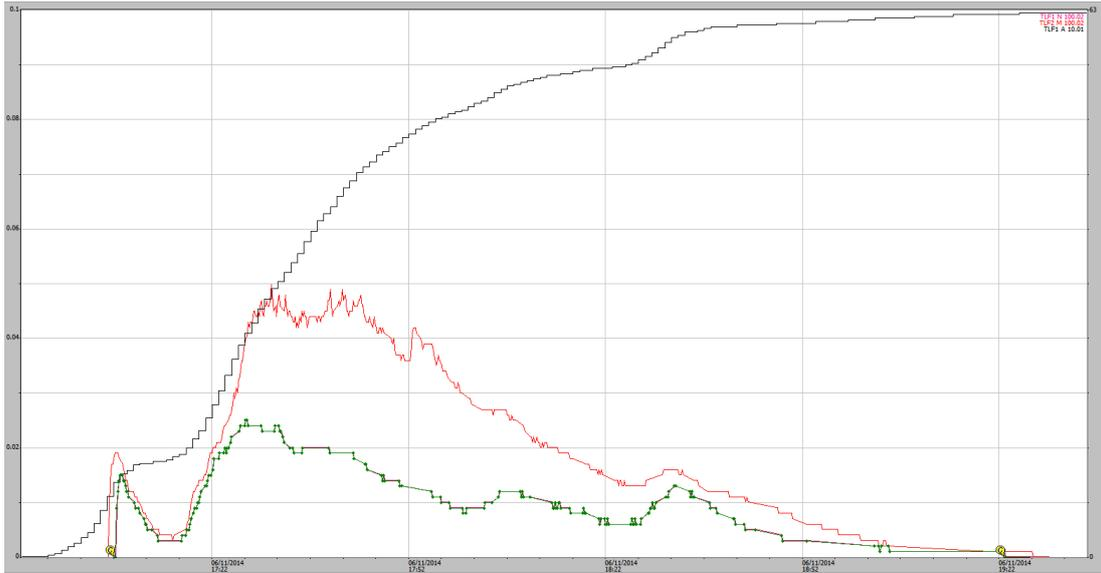
**Figure A1-52** 06/11/2014, 63 mm rain event (black) EP1 shaft encoder (green trace) EP2 shaft encoder (red trace). No boundary overflow problem indicated.
