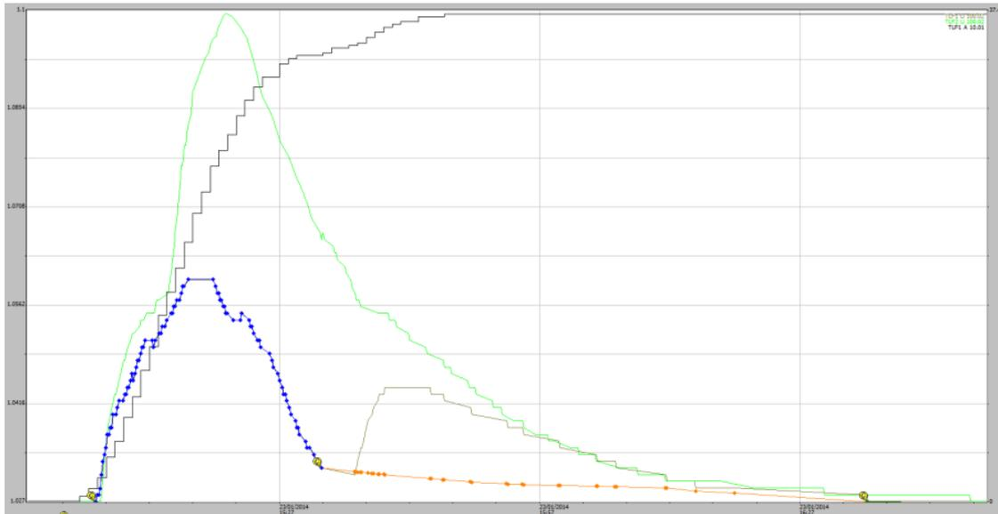
**Figure A1-18** Stage traces for EP1 and EP2 runoff events from 23-01-2014. Some 37 mm of rainfall occurred during the runoff periods and a total of 60 mm rain occurred in the 24-hour period before the end of rainfall.
