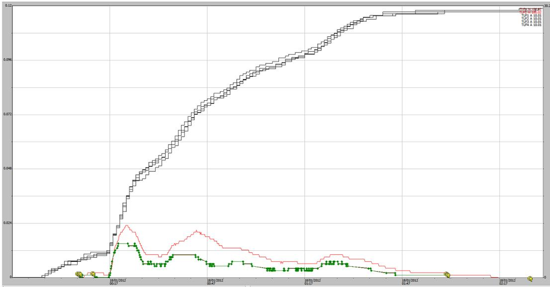
**Figure A1-34** 18/12/2011: 30 mm rain event (rising black traces, plots 1 to 4) EP1 shaft encoder (green trace) EP2 shaft encoder (red trace). No overflow problem indicated.
