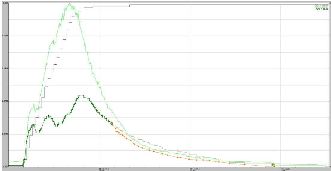
**Figure A1-10** Stage traces for an EP1 and EP2 runoff event on 18-12-2012. Some 31 mm of rainfall occurred during the runoff period and a total of 56 mm of rain occurred in the 24-hour period before the end of rainfall.
