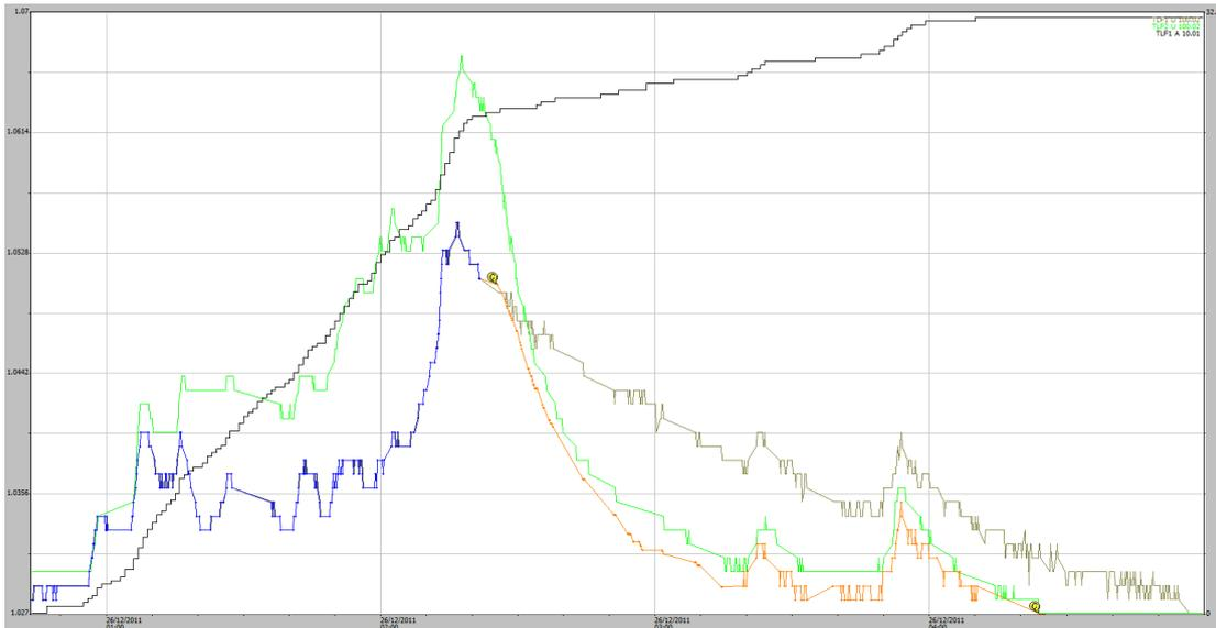
**Figure A1-8** Stage traces for an EP1 and EP2 runoff event on 26-12-2011. Some 58 mm of rainfall occurred during the runoff period and a total of 68 mm of rain occurred in the 24-hour period before the end of rainfall.
