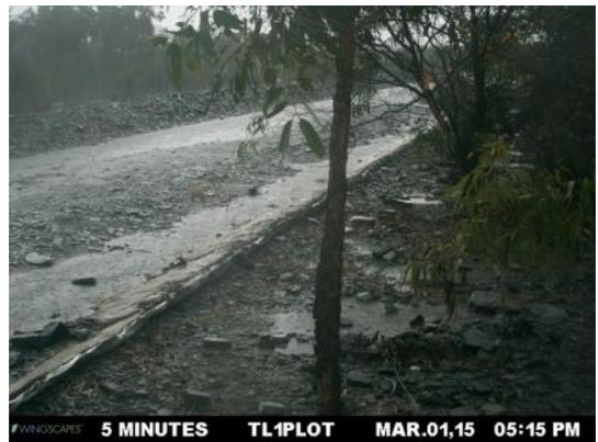
**Figure A2-4** EP1 stage trace for a 22 mm rain event from 4:51 to 5:25 pm on the 01-03-2015 and photo of the adjacent roadside drain showing peak runoff at 5:15 pm with no plot boundary overflow. These events are also illustrated in Figures 16 and 17 of the results as the largest rainfall runoff event captured by camera.
