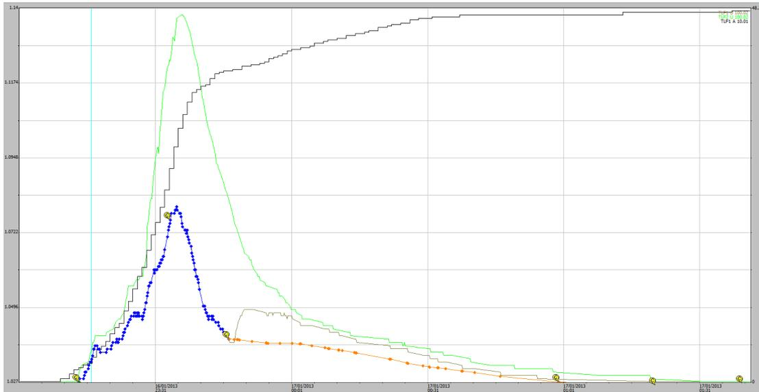
**Figure A1-12** Stage traces for an EP1 and EP2 runoff event on 16-01-2013. Some 48 mm of rainfall occurred during the runoff period and this was also the total rain that had occurred in the 24-hour period before the end of rainfall.
