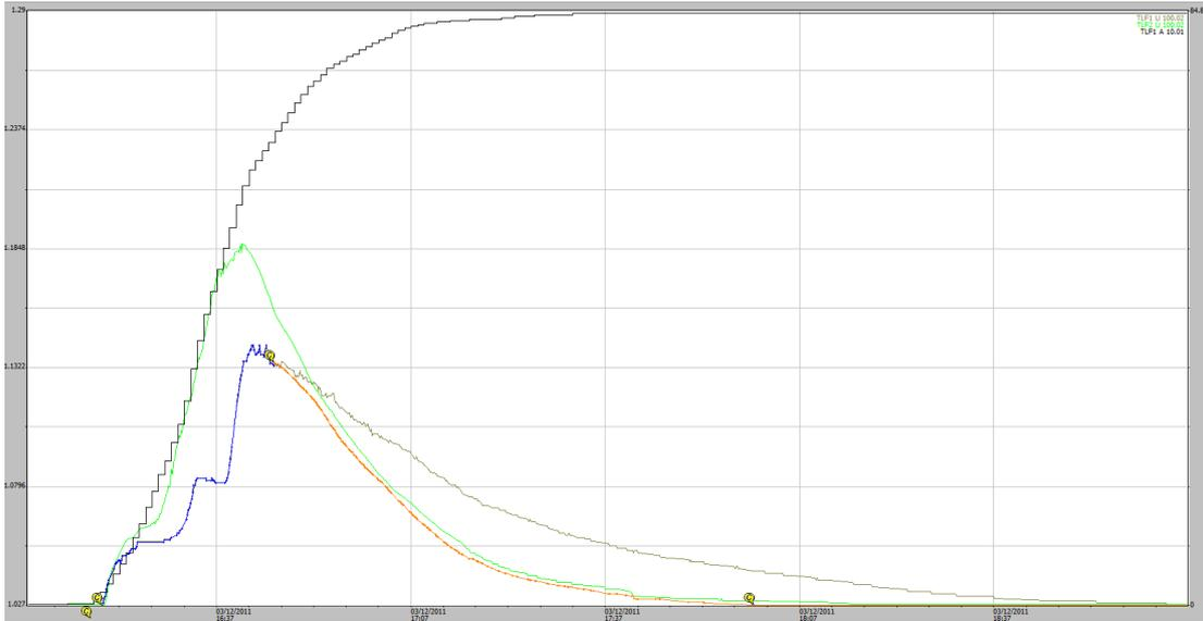
**Figure A1-6** Stage traces for an EP1 and EP2 runoff event on 03-12-2011. Some 84 mm of rainfall occurred during the runoff period this also being the total rain that occurred in the 24-hour period the end of rainfall.
