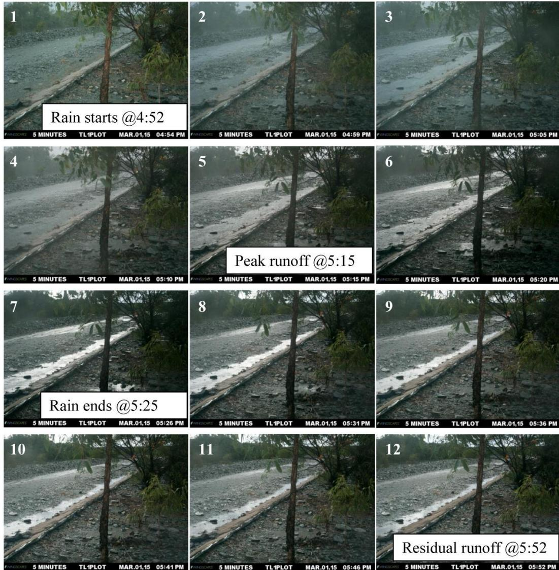
**Figure 16** Five-minute interval photo sequence (1 to 12) showing flow along the roadside drain (to left of EP1) during a 22 mm rain event on 1-03-2015. Rain start and stop times are taken from the EP1 raingauge record illustrated in Figure 17.
