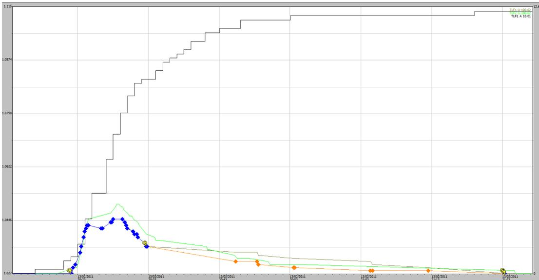
**Figure A1-3** Stage traces for an EP1 and EP2 runoff event on 14-02-2011. Only 13 mm of rainfall occurred during the runoff period but 76 mm occurred in a 24-hour period prior to the end of rainfall.
