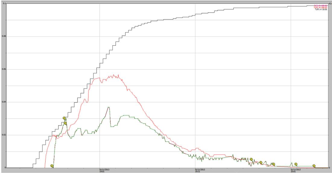
**Figure A1-40** 01/11/2013 (Plot1/2): 43 mm rain event (black) EP1 shaft encoder (green trace) EP2 shaft encoder (red trace). No overflow problem indicated.
