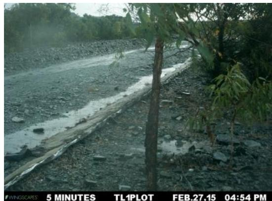
**Figure A2-2** EP1 stage trace for a 5.9 mm rain event from 4:40 to 4:56 pm on the 27-02-2015 and photo of the adjacent roadside drain showing peak runoff at 4:54 pm with no plot boundary overflow.
