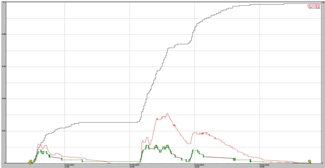
**Figure A1-54** 01/01/2015, 50 mm rain event (black) EP1 shaft encoder (green trace) EP2 shaft encoder (red trace). No boundary overflow problem indicated.
