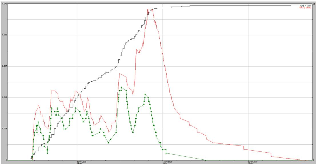
**Figure A1-27** 12/04/2010, 51 mm rain event (black trace) EP1 shaft encoder (green trace) EP2 shaft encoder (red trace). No overflow problem indicated.
