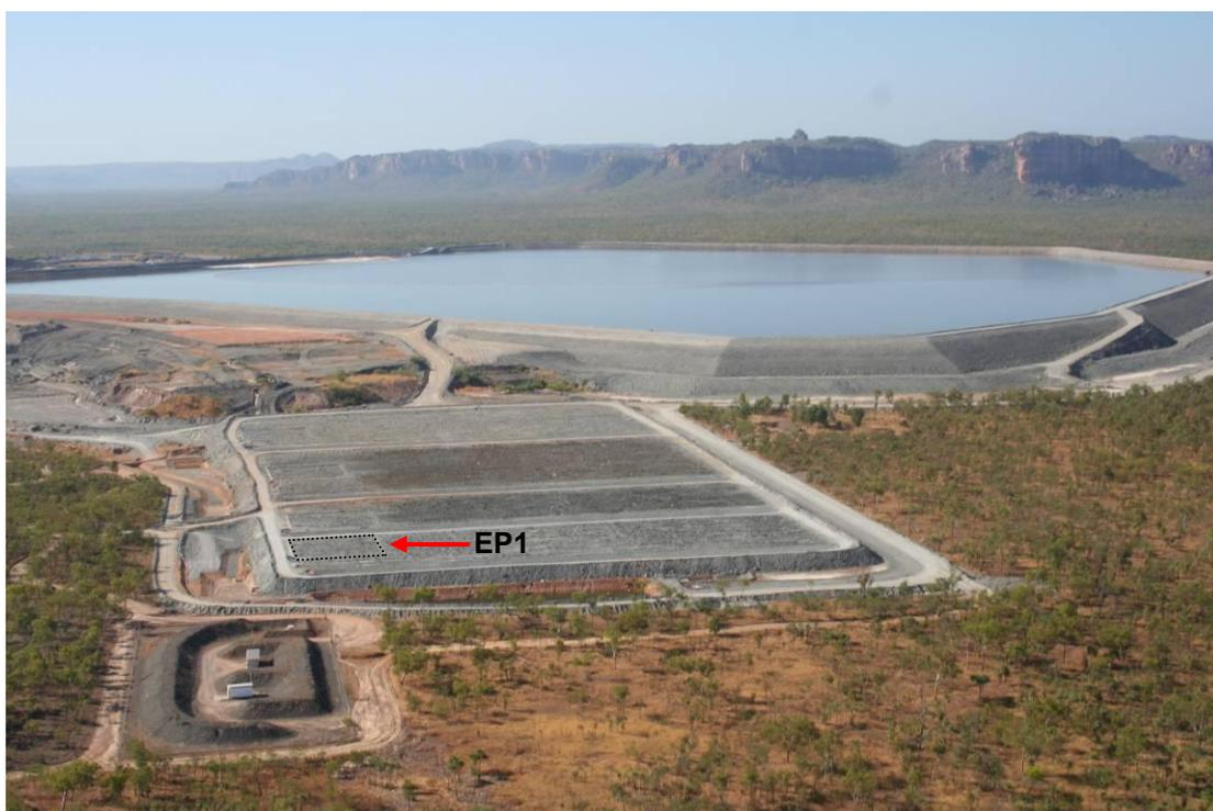
**Figure 2.** Aerial view of the completed Trial Landform located next to the Ranger mine Tailings Storage Facility. Erosion Plot 1 (EP1) is indicated by red arrow and black dotted outline.
