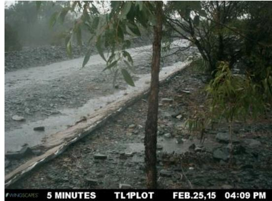
**Figure A2-1** EP1 stage trace for a 5.6mm rain event from 4:06 to 4:07 pm on the 25-02-2015 and photo of the adjacent roadside drain showing peak runoff at 4:09 pm with no plot boundary overflow.
