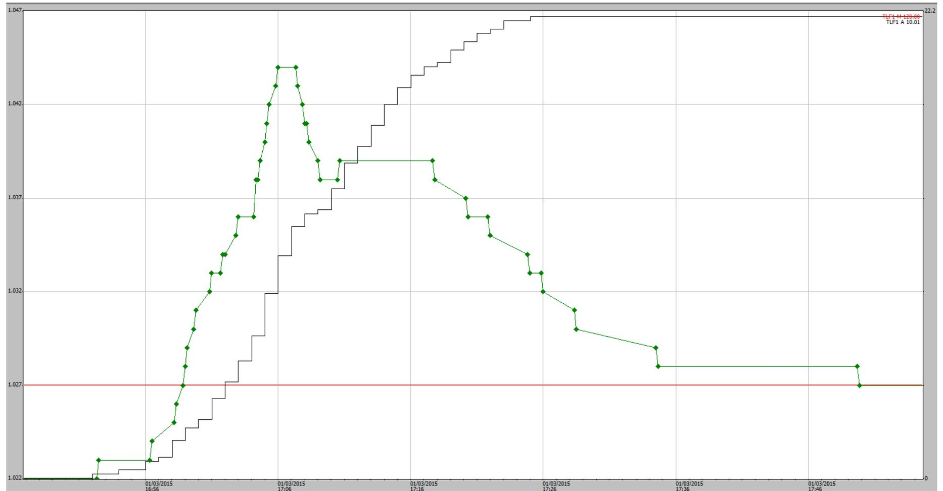
**Figure 17** Shaft-encoder stage trace for EP1 (green line) during the 22 mm rain event (black line) over which roadside drain runoff was also captured on camera (i.e. Figure 16 above). The CTF line is indicated in red.
