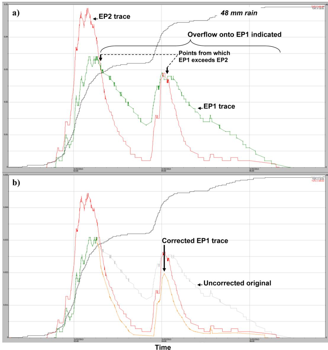
**Figure 7** Evidence and correction of roadside drain overflow event where: **a)** overflow was indicated by the exceedance of the EP1 stage trace in relation to EP2; and **b)** correction applied to abnormal records by manual editing (orange line).
