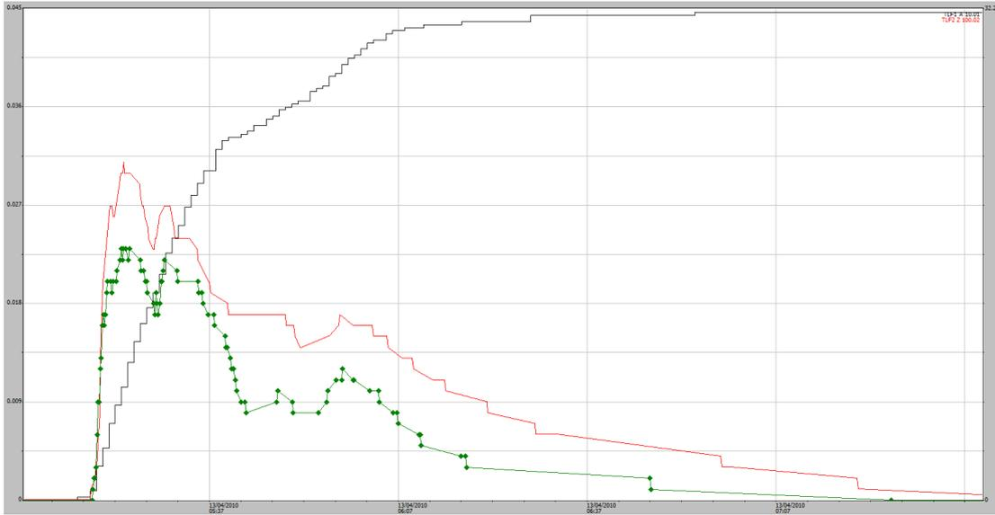
**Figure A1-28** 13/04/2010, 32 mm rain event (black trace) EP1 shaft encoder (green trace) EP2 shaft encoder (red trace). No overflow problem indicated.
