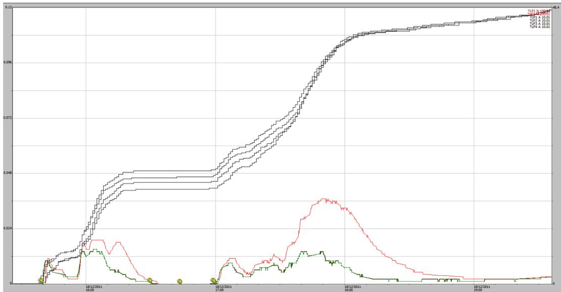
**Figure A1-33** 18/12/2011: 45 mm rain event over two events (rising black traces, plots 1 to 4) EP1 shaft encoder (green trace) EP2 shaft encoder (red trace). No overflow problem indicated.
