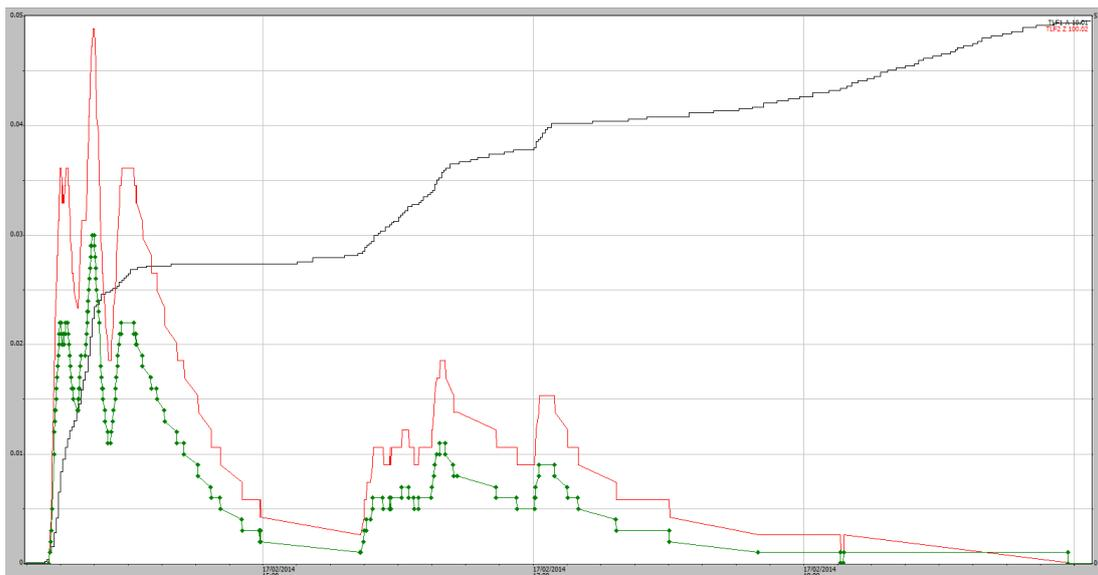
**Figure A1-45** 17/02/2014 (Plot1/2): 53 mm rain event (black) EP1 shaft encoder (green trace) EP2 shaft encoder (red trace). No overflow problem indicated.
