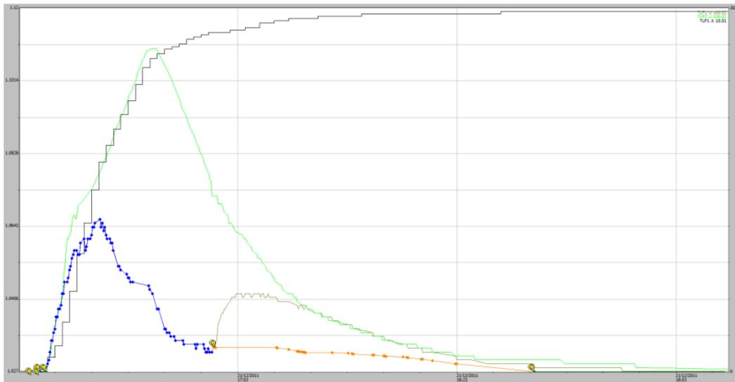
**Figure A1-7** Stage traces for an EP1 and EP2 runoff event on 21-12-2011. Some 30 mm of rainfall occurred during the runoff period and a total of 57 mm of rain occurred in the 24-hour period before the end of rainfall.
