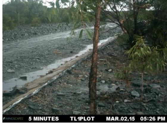
**Figure A2-6** EP1 stage trace for a 1.6 mm rain event from 5:22 to 5:26 PM on the 02-03-2015 and photo of the adjacent roadside drain showing peak runoff at 5:26 PM with no plot boundary overflow.
