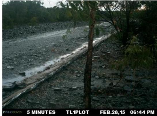
**Figure A2-3** EP1 stage trace for a 2.6 mm rain event from 6:13 to 6:46 pm on the 28-02-2015 and photo of the adjacent roadside drain showing peak runoff at 6:44 pm with no plot boundary overflow.
