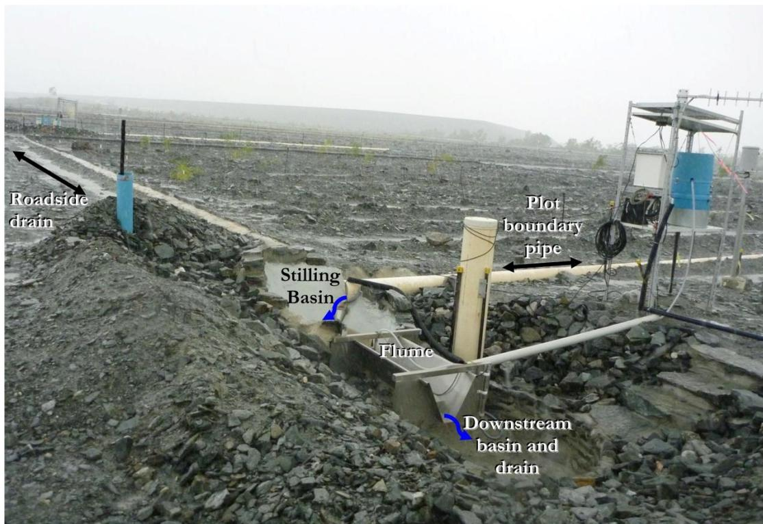
**Figure 3.** Erosion Plot 1 showing the boundary pipe, stilling basin, flume and downstream basin drain. The adjacent roadside drain (top left) is also shown. Photo taken 09-Dec-2009
