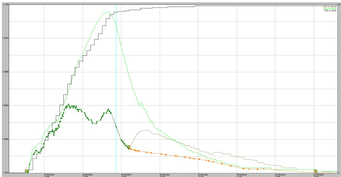
**Figure A1-21** Stage traces for EP1 and EP2 runoff events from 07-03-2014. Some 33 mm of rainfall occurred during the runoff periods and a total of 83 mm rain occurred in the 24-hour period before the end of rainfall.
