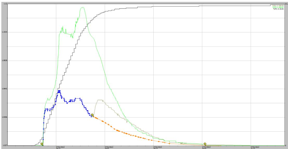
**Figure A1-13** Stage traces for an EP1 and EP2 runoff event on 27-01-2013. Some 53 mm of rainfall occurred during the runoff period and this was also the total rain that had occurred in the 24-hour period before the end of rainfall.
