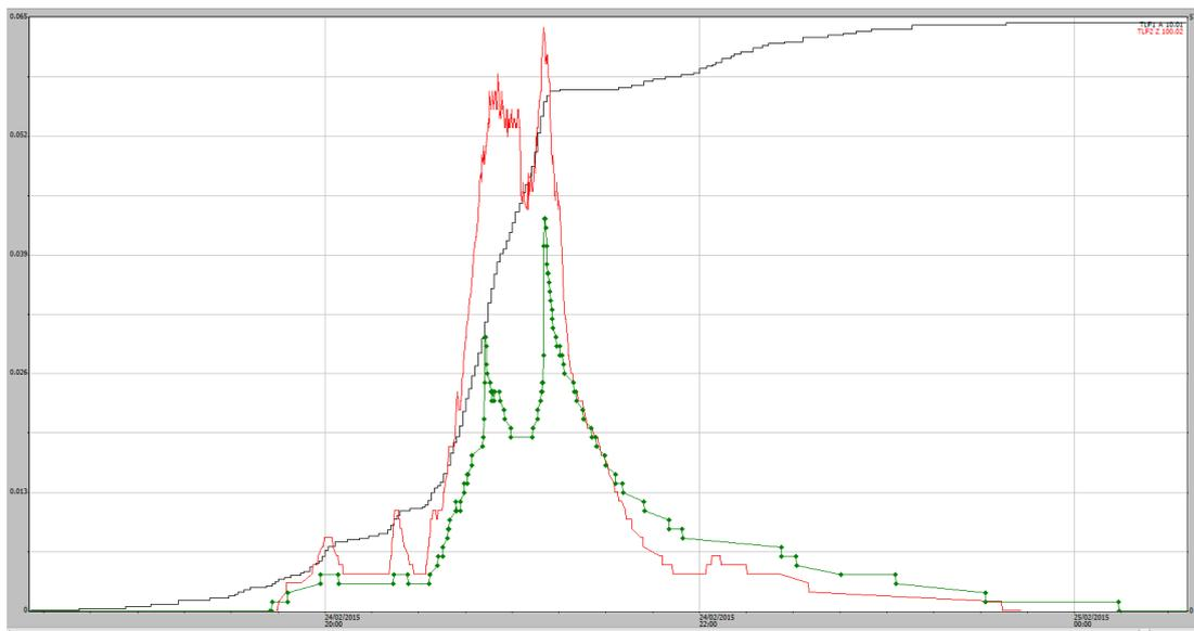
**Figure A1-55** 24/02/2015, 56 mm rain event (black) EP1 shaft encoder (green trace) EP2 shaft encoder (red trace). Marginal boundary overflow indicated on recession but no correction applied.
