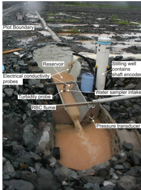
Figure 3 Instrumentation installed on individual erosion plots
