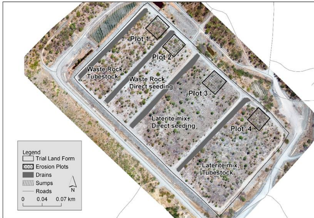
Figure 2 Layout and location of erosion plots on the Ranger trial landform.
