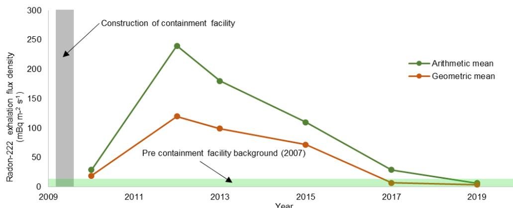
**Figure 3** Mean radon-222 exhalation flux density changes on the containment since construction
