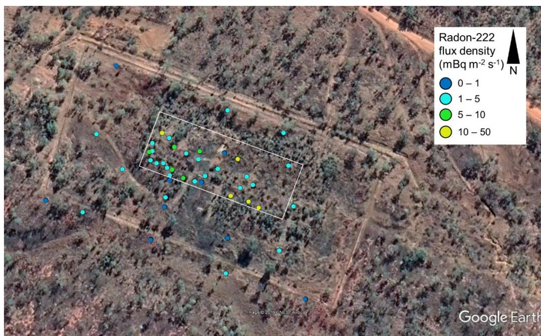
**Figure 1** Radon-222 exhalation flux densities measured at the measured at the South Alligator Containment Facility in May/June 2019 (the white rectangular outline indicates the location of the containment).
