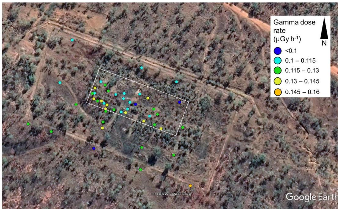
**Figure 2** Gamma dose rates measured South Alligator Containment Facility in May 2019 (the white rectangular outline indicates the location of the containment).
