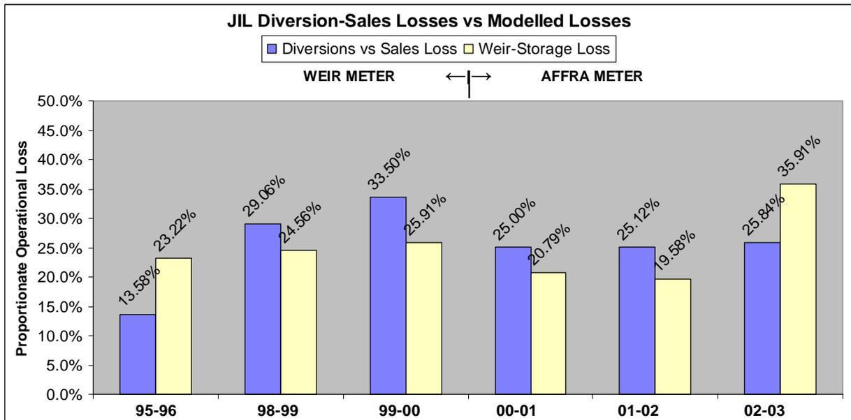
Figure 7, Historic Water Balance Losses versus Preliminary Weir-storage losses
