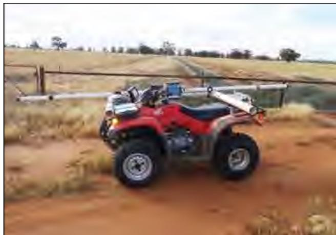
**Figure 10:** Geonics EM31-MK2 and Trimble® EZ-Guide™ dGPS equipment fitted to the 4-wheel motorbike used in the assessment
