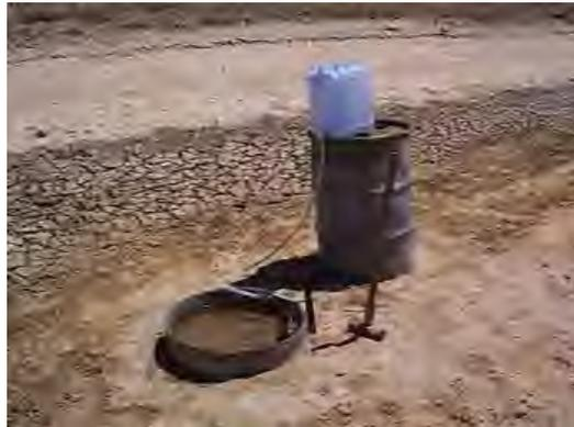
**Figure 14:** Ring infiltrometer (ANCID, 2004) similar to the one used in the initial (failed) ring infiltrometer trials in this study
