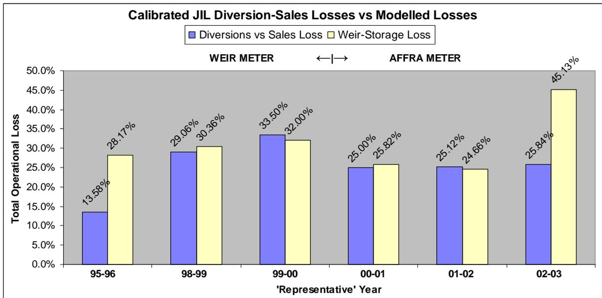
Figure 8, Historic Water Balance Losses versus Calibrated Weir-storage losses.
