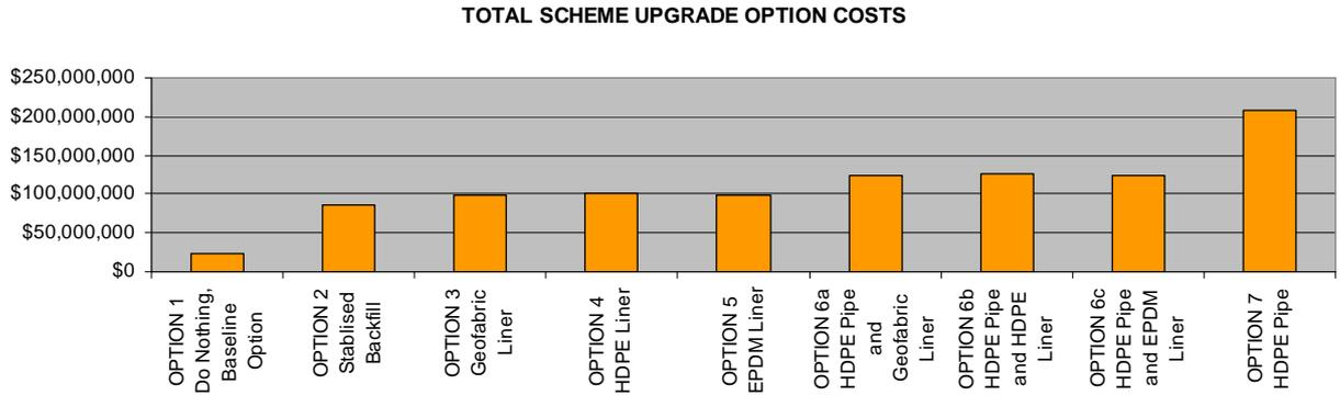
Figure 14, option upgrade total cost comparison
