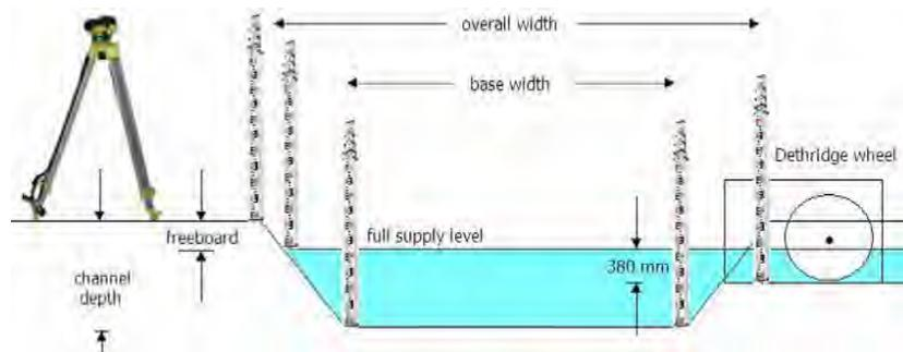
**Figure 9:** Diagrammatic representation of measurements made in the cross-sectional survey
