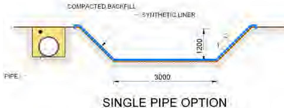
Figure 10, HDPE Pressure Pipe concept
