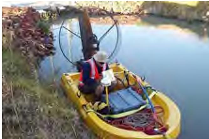
**Figure 12:** Boat-mounted electrical resistivity survey equipment similar to that used in this assessment (©Groundwater Imaging)
