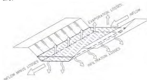
Figure 5, Elements of open-channel losses
