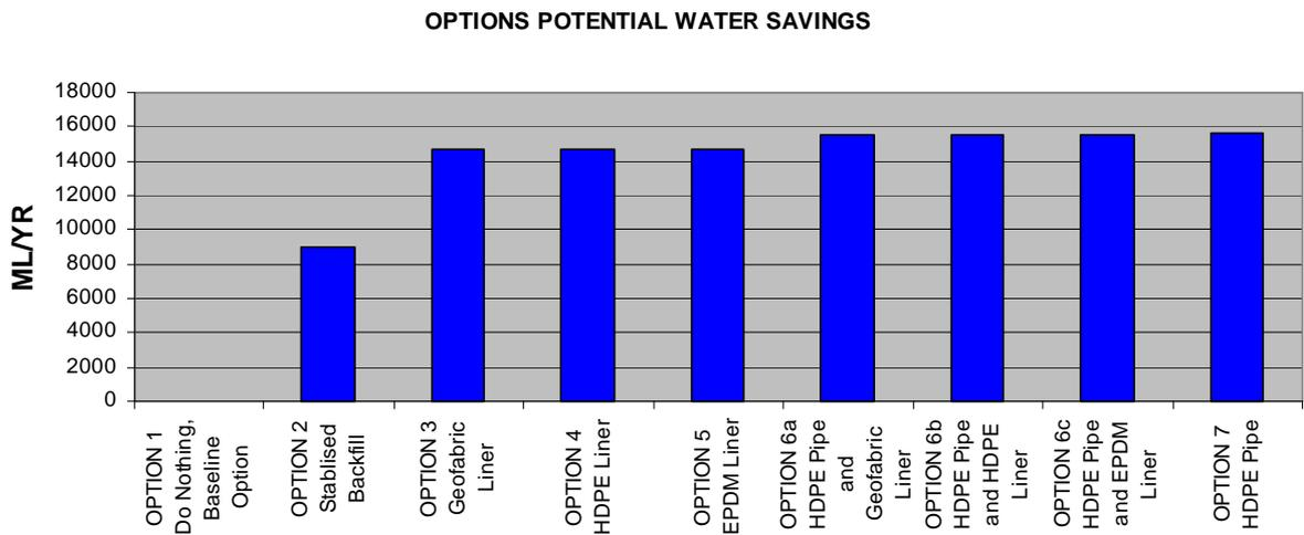
Figure 15, option upgrade total potential water savings
