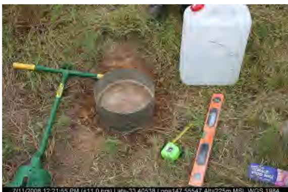
Image 11, Indicative infiltration testing carried out using an single ring infiltrometer source B&P
