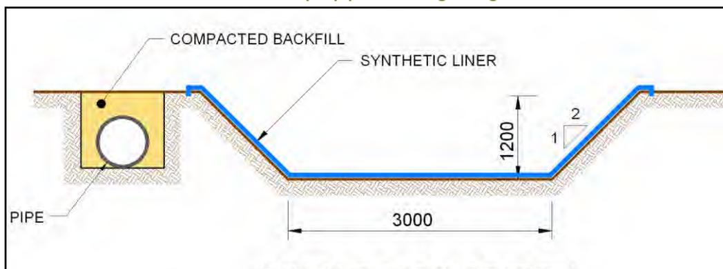
In this option, Division 2 may be lined with any of the synthetic liners if felt appropriate.
