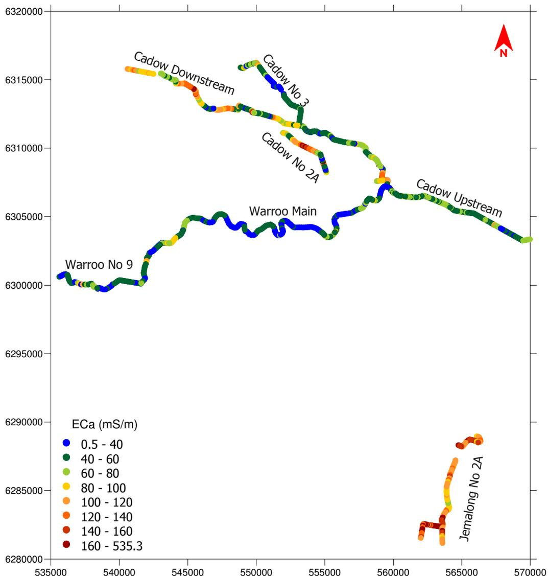
Figure 18: Plot of  $EC_a$  values in EM31 surveyed channels
