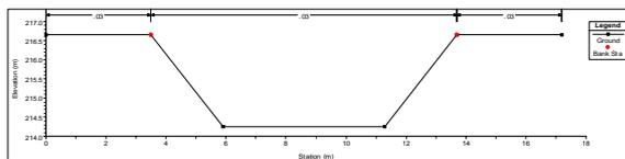
Figure 2, Typical cross section of the Jemalong Irrigation delivery system.
