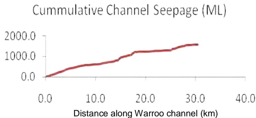
**Figure 18** Annual estimates of cumulative channel seepage using Idaho seepage metre test results carried out after every 200 metres or more frequently along the Warroo main supply channel.
