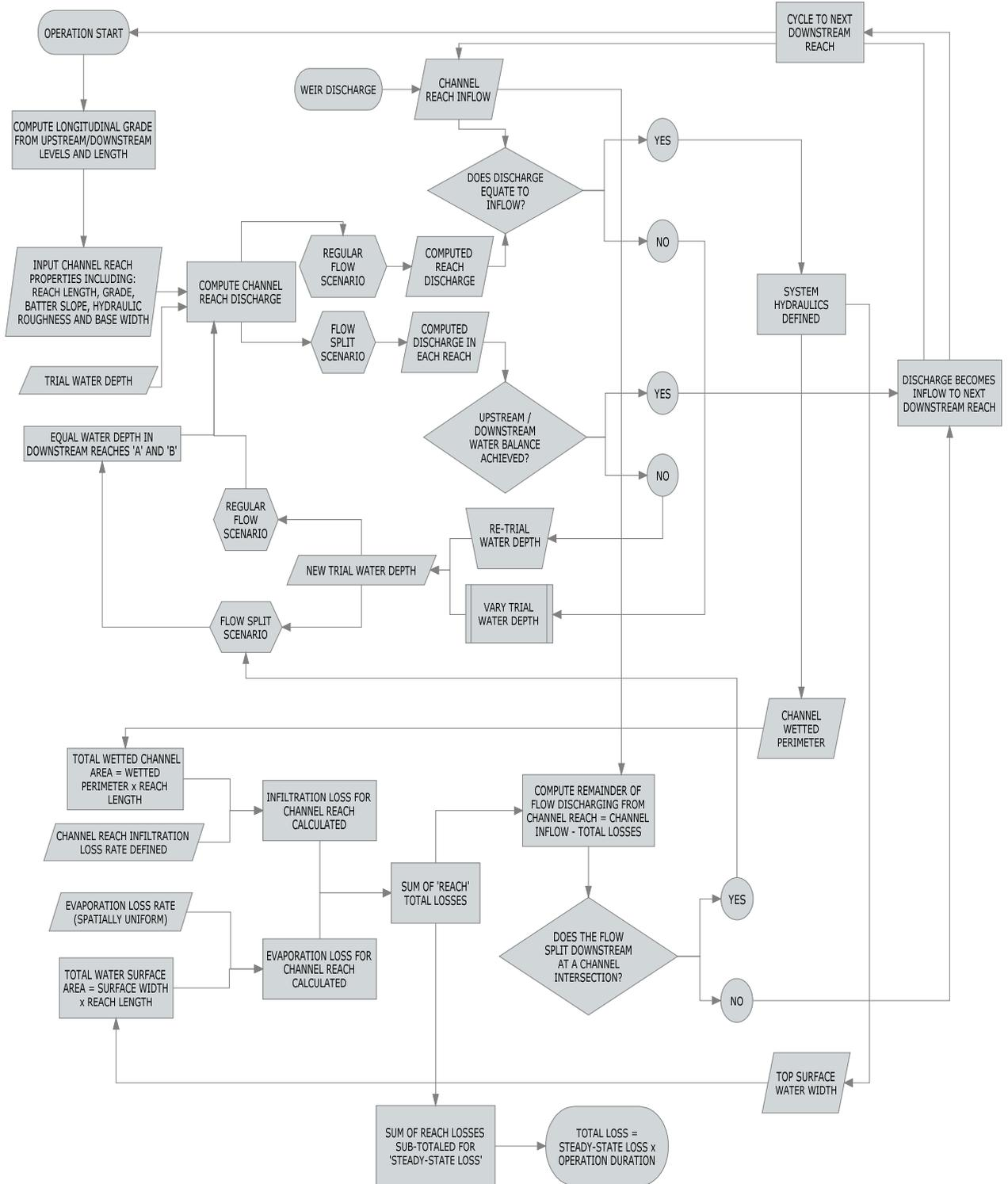
Figure 17, Summary of the operations of the Mass Balance Loss Model
