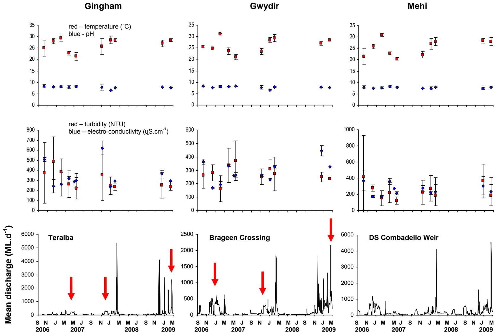
**Fig. 7.6a.** Mean pH, water temperature, electro-conductivity, turbidity and discharge within the three study watercourses, October 2006 to February 2009. The discharge hydrograph is shown for each watercourse, with ECA releases indicated by red arrows.
