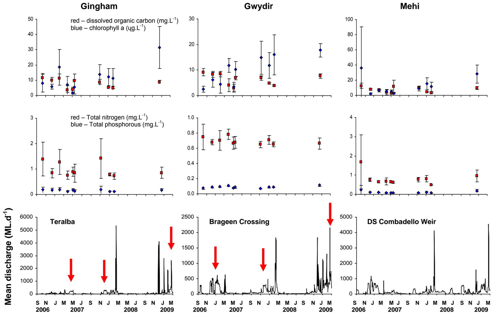
**Fig. 7.6b.** Mean concentration of dissolved organic carbon, chlorophyll a (phaeophytin corrected), total nitrogen, total phosphorous and discharge within the three study watercourses, October 2006 to February 2009. The discharge hydrograph is shown for each watercourse, with ECA releases indicated by red arrows.
