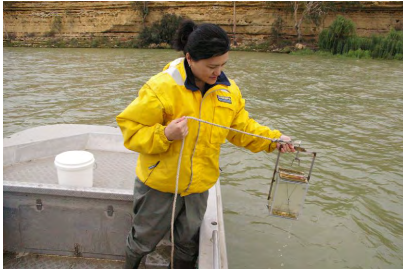
Figure G1. Perspex Haney trap used for sampling zooplankton assemblage in the main channel of the Lower Murray River.
