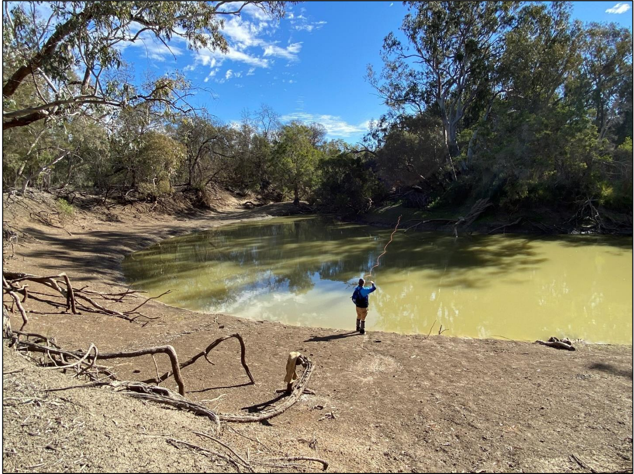
Figure 30. Staff measuring the depth of a refuge pool using a portable depth sounder. 3.4 km upstream of the Macintyre-Gnoura Gnoura Creek confluence, in the Boomi Management Reach, 21/7/2020. Flow rate was 51 ML/day.
