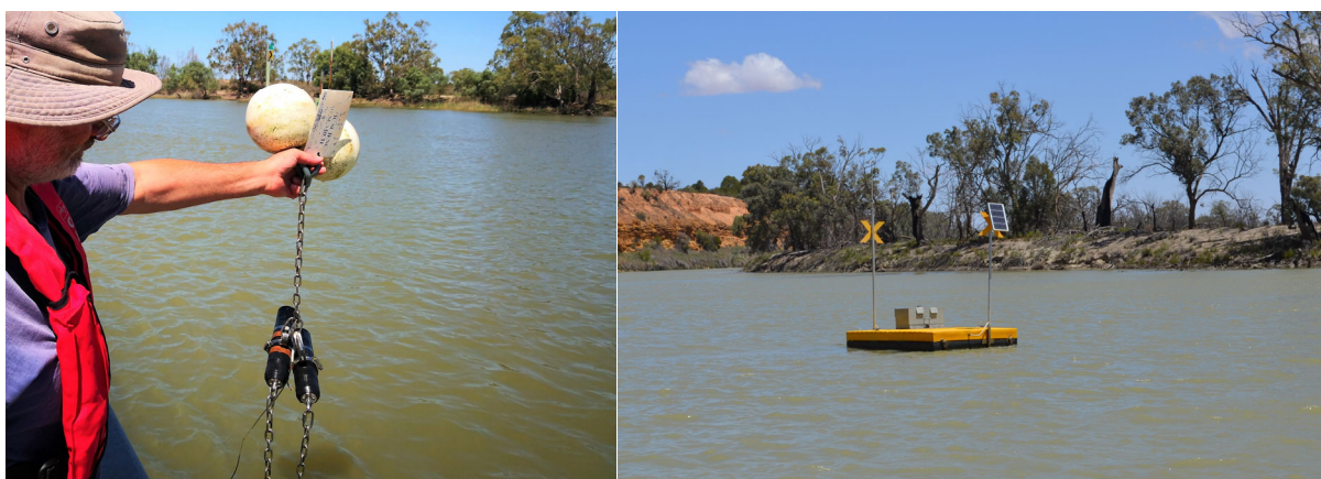
Figure 6. Loggers that are deployed in the Lower Murray to measure dissolved oxygen concentrations (left) and the typical mooring station (right) (photos: SARDI).
