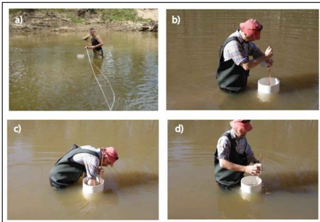
Figure 2-6. The method for field sampling of fine-grained sediment in the bed: a) sampling area measurement from bank for random sampling site selection, b) disturbance of bed sediments within cylinder, c) suspended sample collection, and d) collected sample to be transferred to combined 1L sample for subsequent analysis.
