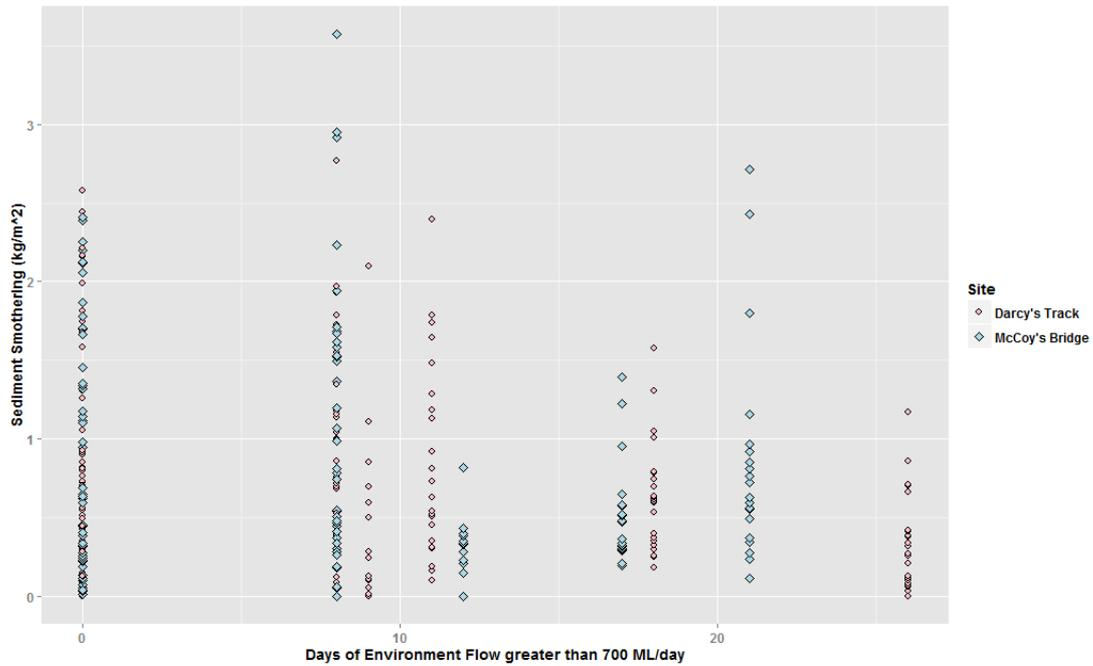
Figure 2-15. Sediment smothering ( $\text{kg/m}^2$ ) relative to the number of days where environmental flows are provided for freshes. Data are plotted for environmental flows  $> 700 \text{ ML/d}$ , since flows of this magnitude were commonly contributed for the purposes of freshes (rather than baseflows).
