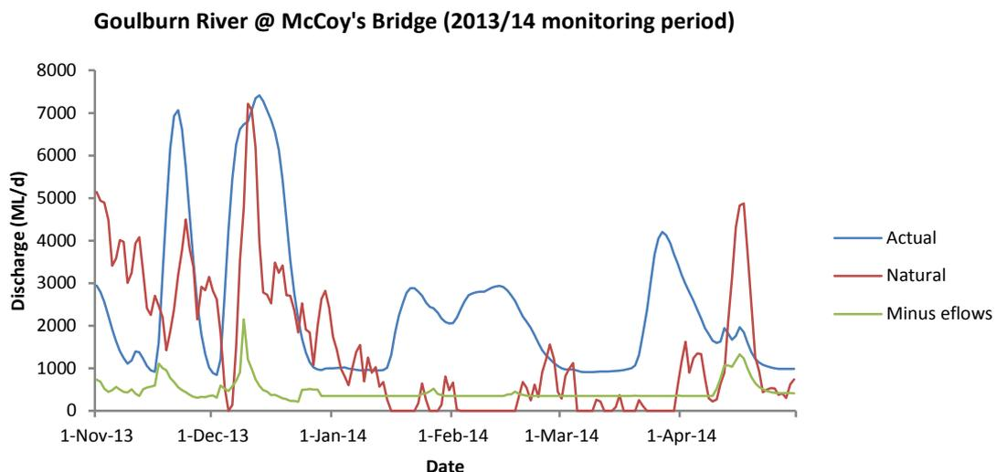
Figure 1-3. Environmental flow delivery in the lower Goulburn River. Graph covers 1/11/13 – 30/4/14, the approximate period of the monitoring program. Lines depict actual discharges, modelled natural discharges without regulation, and discharge minus environmental flow amounts, as depicted in the key.
