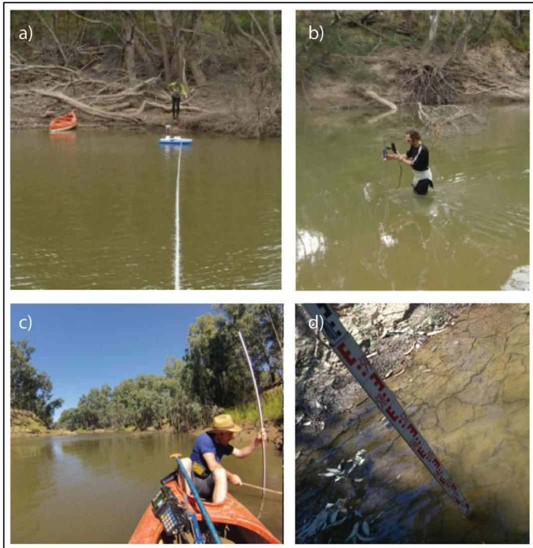
Figure 2-5. a) using the ADCP to assess field hydraulics along transects, b) use of a handheld ADV to test velocity across transects, c) measurement of extent of pool depth along a transect, and d) measuring depth in slackwaters.
