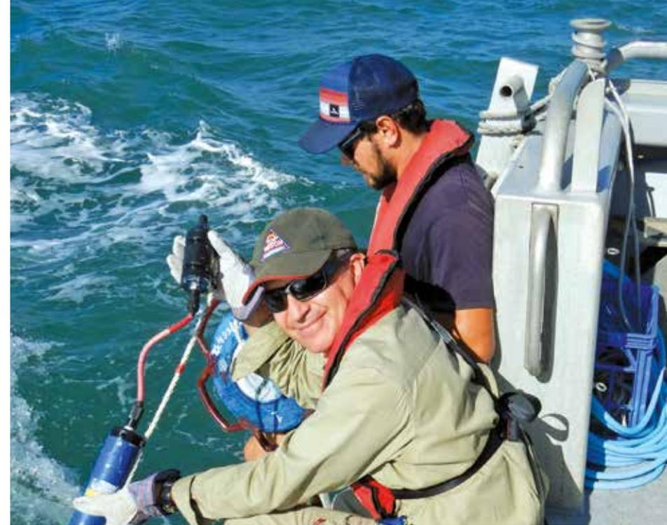
*Underwater acoustic sensors were deployed in groups for up to sixty days through Torres Strait making it possible to provide a more accurate estimate of overall annual vessel movements.*
