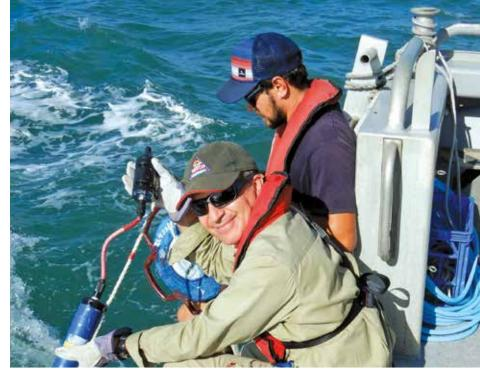
Underwater accoustic sensors were deployed in groups for up to sixty days throught Torres Strait making it possible to provide a more accurate estimate of overall annual vessel movements.
