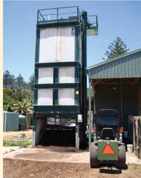
Figure 4.6: The vertical composting unit on Lord Howe Island.
