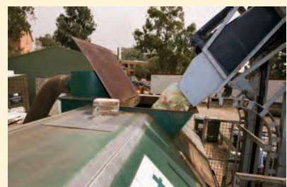
3. Feedstock emptying into the HotRot
