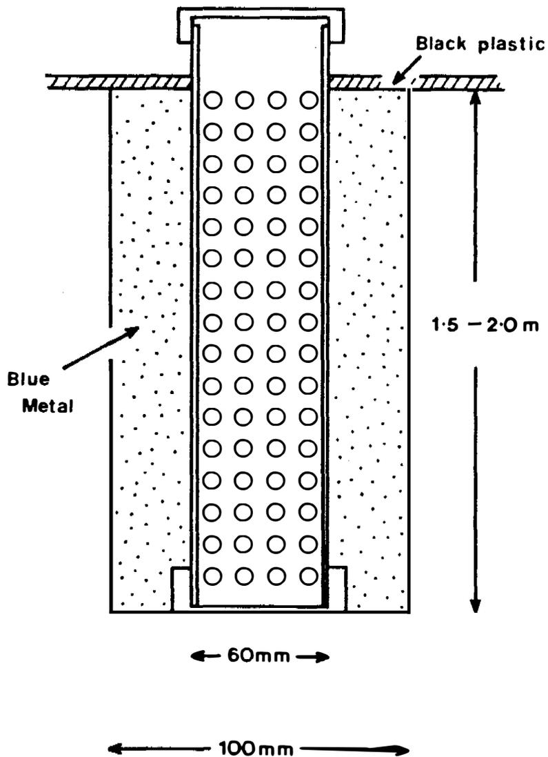
Fig. 3.1-2<sup>a</sup> Detail of construction of the bore used for sampling groundwater at Jabiluka.
