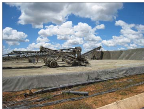
Figure 5.3 Stockpiling of ore on the heap leach pad at Caetite uranium mine, Bahia, Brazil
