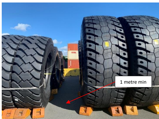
Figure 2 Tyre presentation using chocks – minimum spacing
