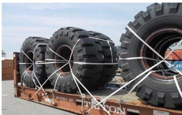
Figure 5 Tyre presentation using chocks, straps and flat rack
