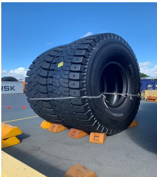
Figure 2 Tyre presentation using chocks – minimum spacing
