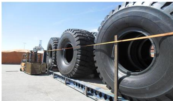
Figure 4 Tyre presentation using chocks and steel bracing
