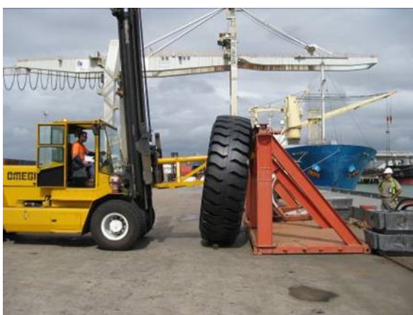
Figure 7 Tyre presentation using inspection stand
