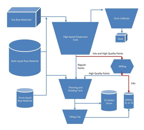
Figure 1: Generic process flow diagram for paint and ink manufacturing.
