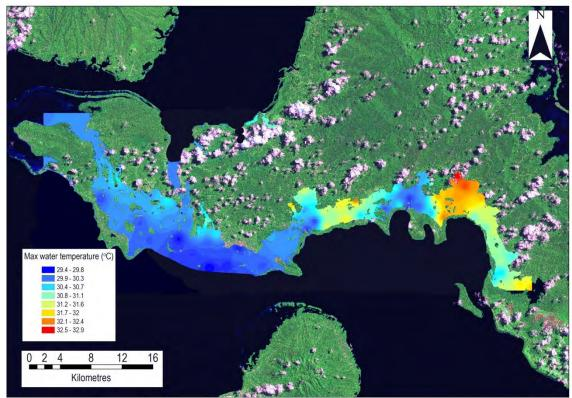
Figure 90 Large scale variability in maximum water temperature observed during July 2010 baseline water quality assessment.
