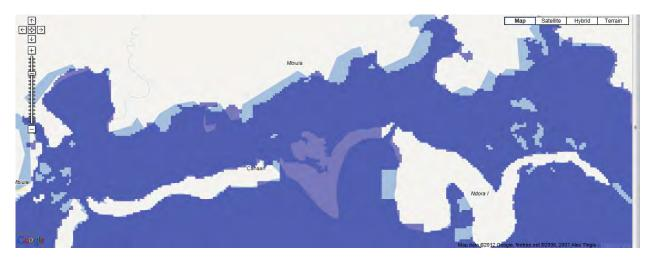
Figure 23 Example of modelled 1 m sea level rise in Roviana Lagoon from SRTM based inundation tool.
