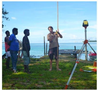
Figure 36 Training RCF zone co-ordinators in the use of laser level survey equipment
