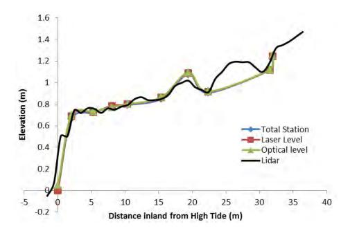
Figure 26 Comparison of elevation data from High tide to 1.2 m inland using LiDAR, Total Station, Laser and Optical level
