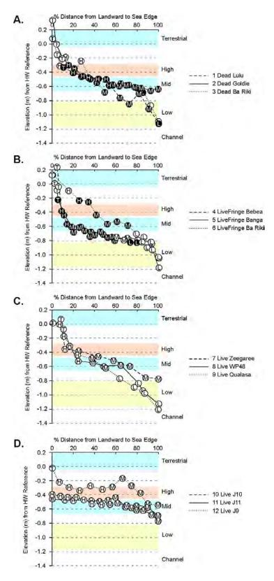
Figure 86 Representations of the 12 transects showing: relative elevation and shape of profiles (elevation in metres, zero reference at high water on first day – 21 March 2011); zonal position marked by vegetation assemblages (High = H; Mid = M; Low = L; Terrestrial = T); and dieback state (dieback = solid black circles; no dieback = white circles). Transect lengths were standardised (%) from distances listed in Table 29. Zones positioned from non dieback transects, see Table 31.
