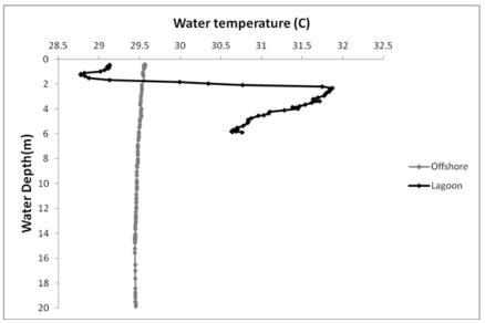
Figure 91 Rapid changes in water temperature profiles at lagoon sites versus relatively uniform profile from offshore site.
