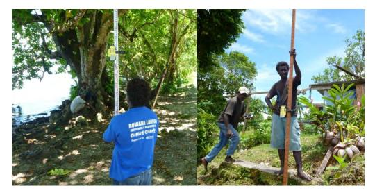
Figure 29 Laser detector attached to 4 m staff (left) and locally created staff (right)
