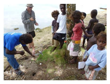
Figure 27 Establishing estimated HAT and marking with survey peg
