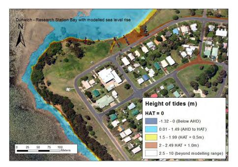
Figure 24 Inundation map of Dunwich, North Stradbroke island, Australia-based on LiDAR data
