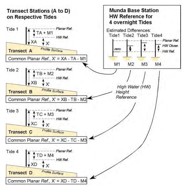
Figure 85 The method used in this investigation for transferring a standardised reference across all transects measured during different days across the study area. Three replicate High Water Measuring Bottles were deployed each day at the Munda Base Station and respective transect locations.
