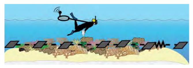
Figure 38: Conceptual diagram of georeferenced photo transects, where a snorkeler is taking photos of benthos at regular intervals while a GPS is tracking its position at the surface.
