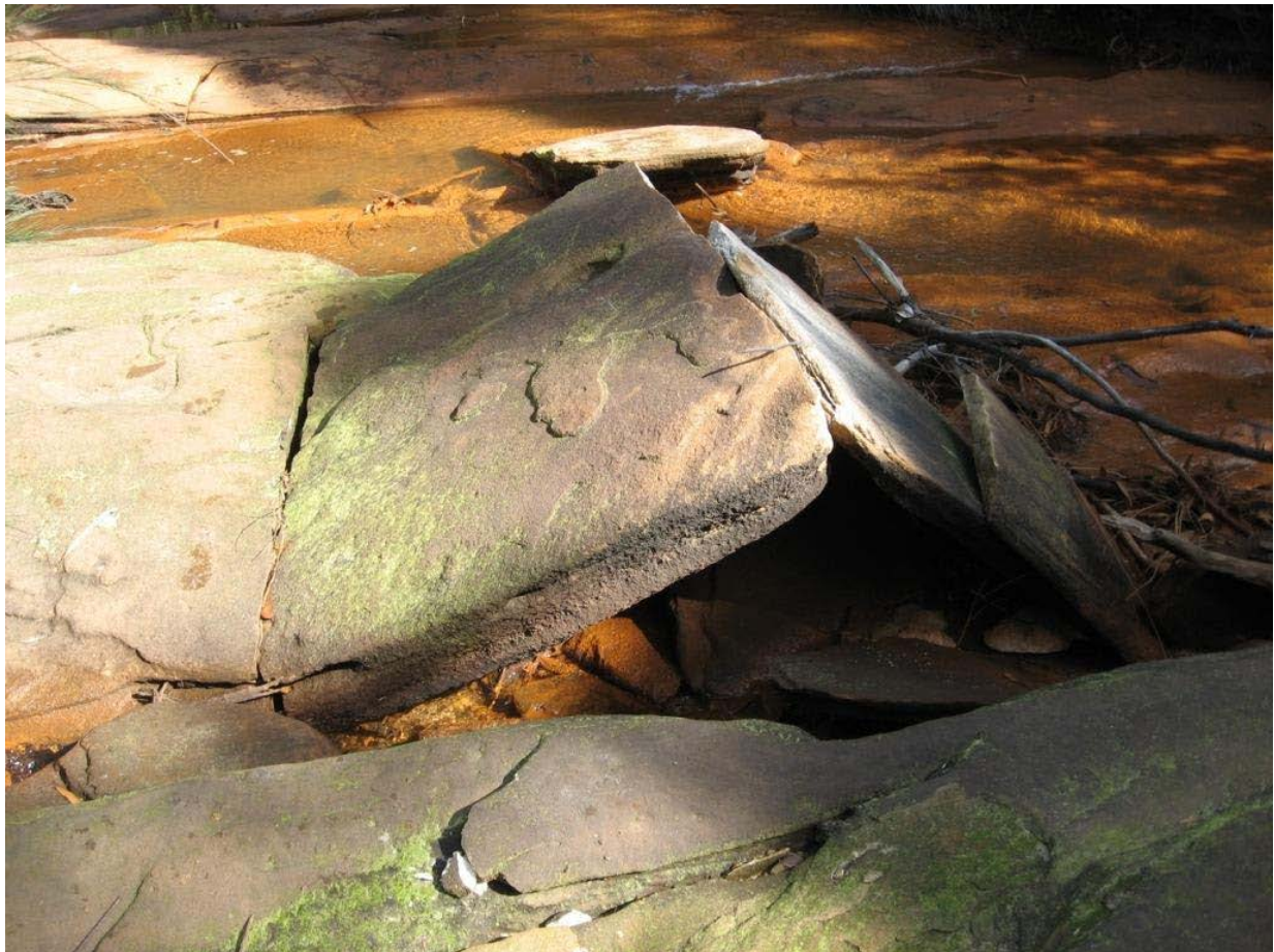
Figure 3.5 Buckling of near surface, Waratah Rivulet (Southern Coalfield), late 2004.
