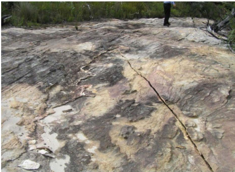
Figure 8.7 Tensile crack and horizontal shear movement (on left) in zone of upsidence in the floor of the valley subject to valley closure movements.
