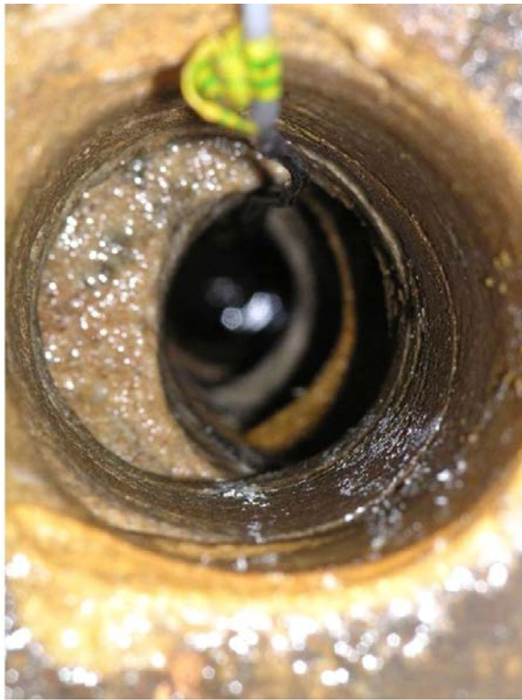
Figure 8.5 Example of shear movements in a vertical borehole drilled in a sandstone rockbar subject to valley closure movements.
