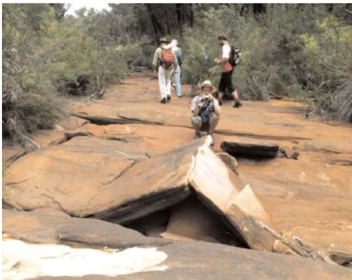
Figure 8.6 Example of upward buckling of restrained surface strata as a result of valley closure movements concentrated in the floor of the valley.
