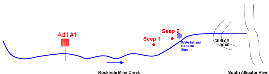
Figure 3.20 Schematic (not to scale) of Rockhole Mine Creek showing the location of Adit 1 and two downstream seeps
