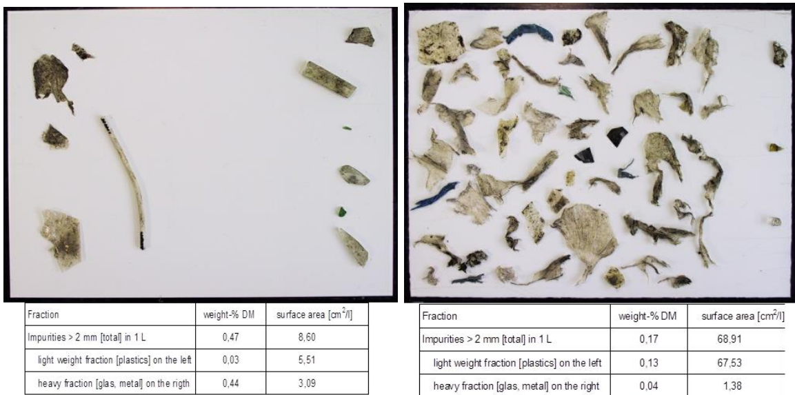
Figure 3: Physical impurities (> 2 mm) in compost expressed on the basis of weight and surface area, dominated by heavy particles (left) or lightweight particles (right) [Source: Thelen-Jüngling 2008]
