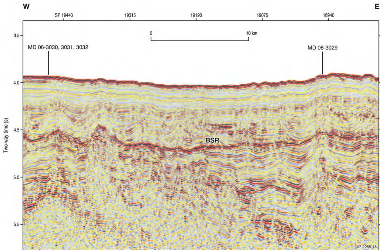
Figure 3.58. Seismic profile at eastern flank of central Fairway Basin, showing the distinctive bottom simulating reflector (BSR) and location of cores. GA line 177/LHRNR-BA, Location in Figure 3.54. Colwell et al., (2006)
