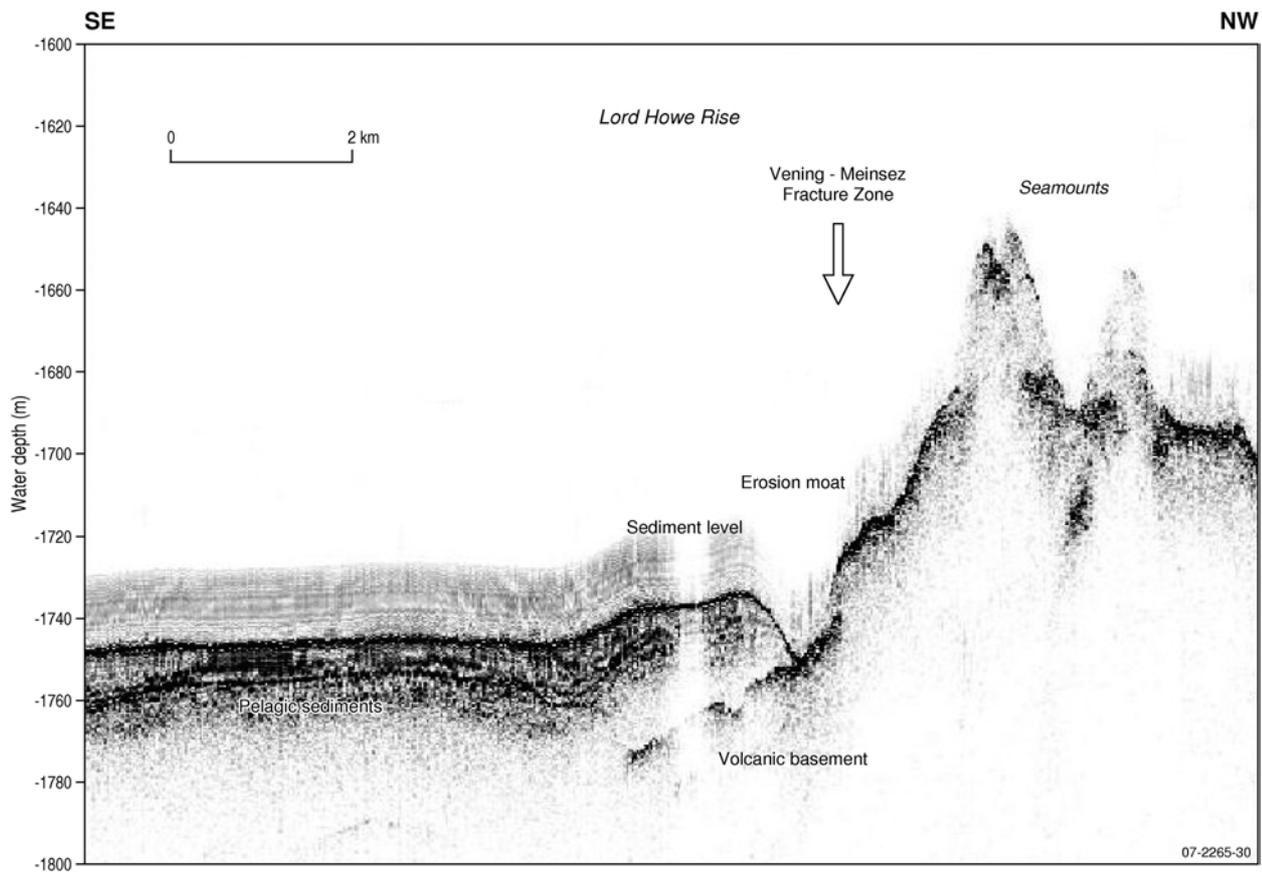
Figure 3.42. Seismic profile across the Vening-Meinesz Fracture Zone on the Lord Howe Rise showing erosion by bottom currents at the base of volcanic ridges. Location on Figure 3.39. Colwell et al., (2006).
