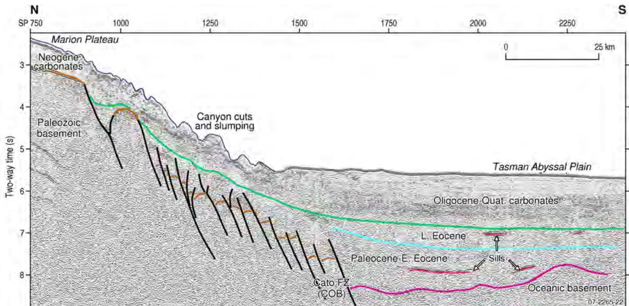
Figure 3.35. Seismic profile showing sediment slumping from the Marion Plateau and relatively shallow turbidites forming the abyssal plain, north Tasman Basin. Note the location of the Cato Fracture Zone separating oceanic crust from continental crust. Location is on Figure 3.1. Line 1. Exon et al., (2005).
