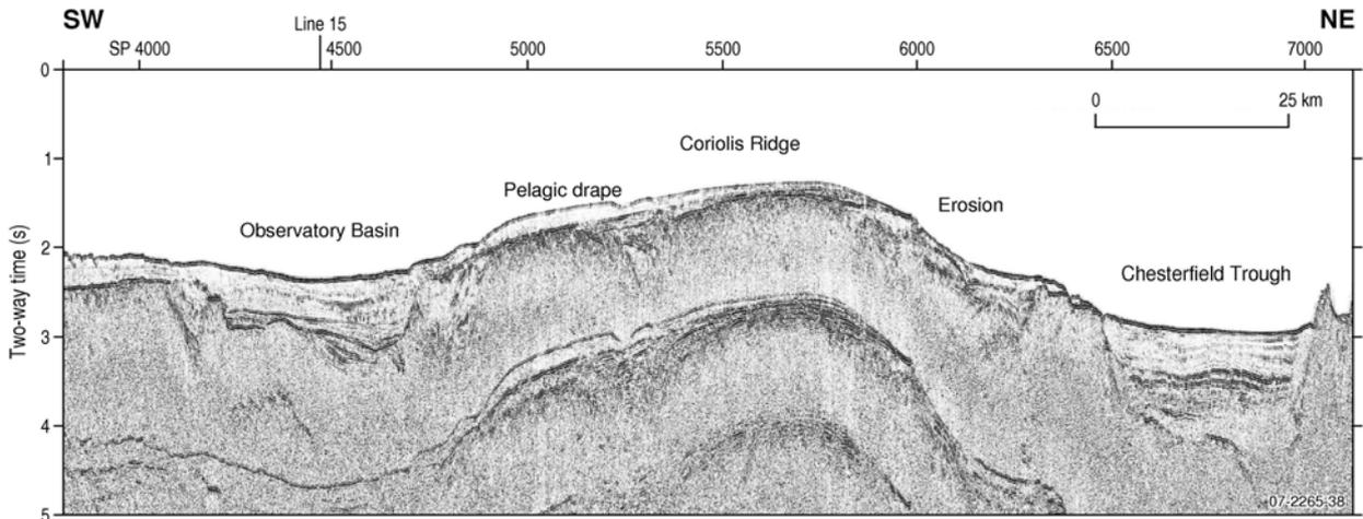
Figure 3.48. Seismic profile across the Observatory Basin, Coriolis Ridge and Chesterfield Trough showing general drape of pelagic sediments. Line 270-3. Location in Figure 3.44. Exon *et al.*, (2005).
