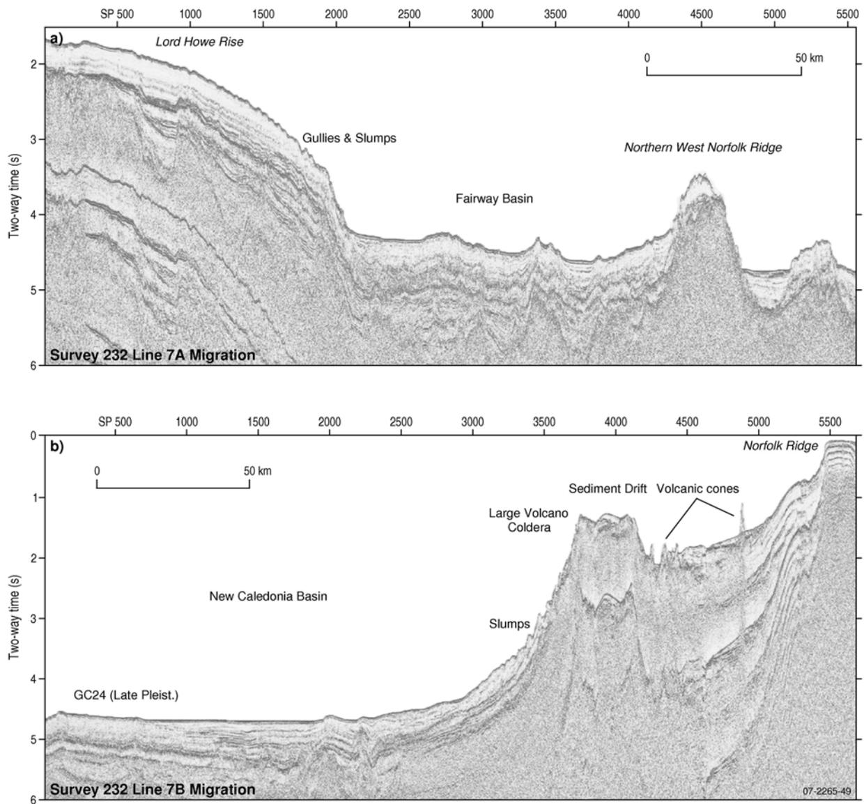
Figure 3.56. a) Seismic profile from Lord Howe Rise across the South Fairway Basin to the Northern West Norfolk Ridge showing hills in the basin and steep ridges and b) Seismic profile from the New Caledonia Basin to Norfolk Ridge showing volcanic cones, sediment drifts and slumping. Lines 232-7A and 7B, Exon et al., (2004b).
