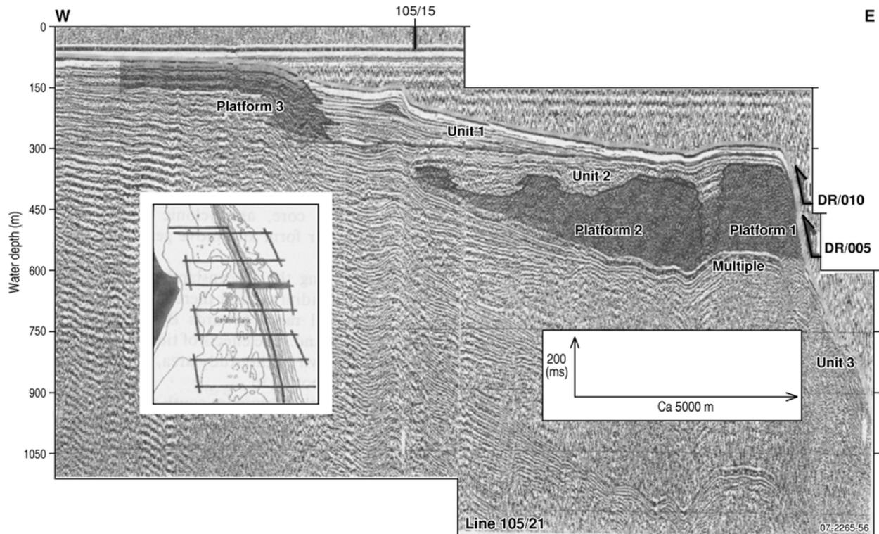
Figure 3.15. Seismic profile showing the carbonate platforms and sedimentary units on the outer shelf and upper slope offshore of Fraser Island (Marshall et al., 1998).
