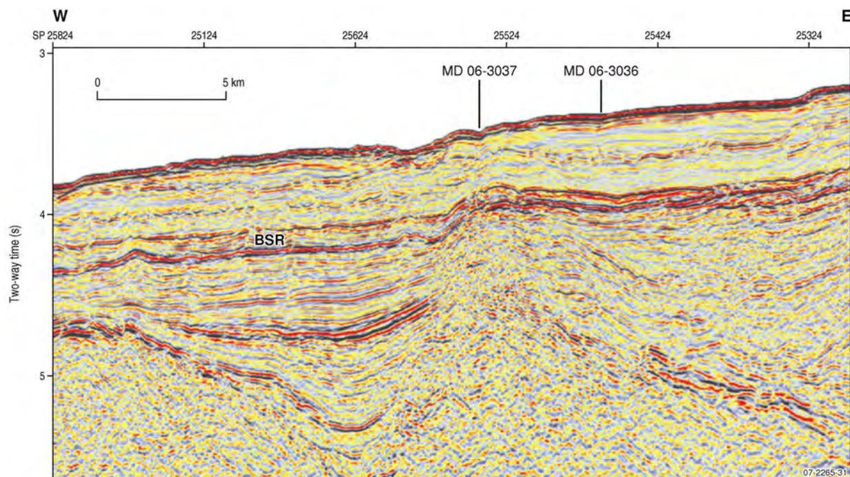
Figure 3.43. Seismic profile showing bottom simulating reflector (BSR) in Capel Basin, western flank of Lord Howe Rise and location of cores. Note the seafloor is irregular above subsurface domes. Location on Figure 3.39. GA line 206/04, Colwell et al., (2006).
