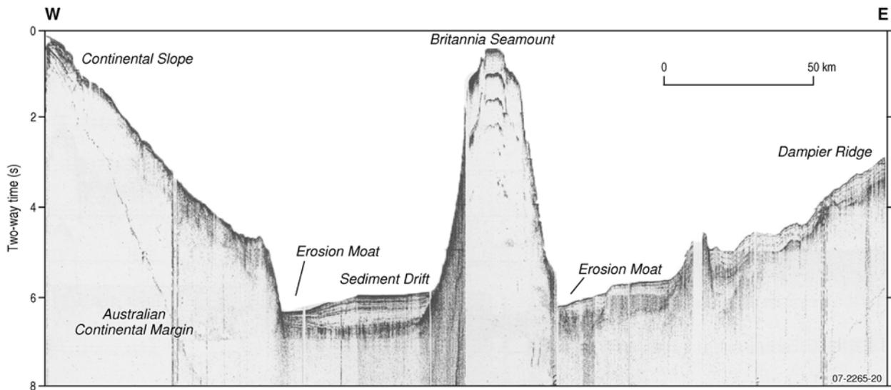
Figure 3.33. Seismic profile in the north Tasman Basin from east of Tweed Heads to the Dampier Ridge passing over Britannia Seamount. Note the wide mid-slope and steep lower slope with erosion moat at its base in the abyssal plain. Deposition by bottom currents has formed a sediment drift and apron at the base of seamount. There is an erosion moat on the east side of Britannia Seamount. Location is on Figure 3.1. Eltanin Line 29.
