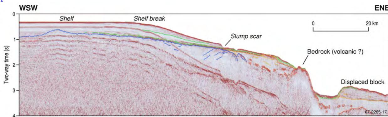
Figure 3.30. Seismic profile across the slope illustrated in Figure 3.29. Note the upper slope sediment wedge, slide scar, older rift sediment basin in the mid slope with a volcanic ridge exposed on the down slope side. Location on Figure 3.11. Line 007, Glenn et al., (2007).
