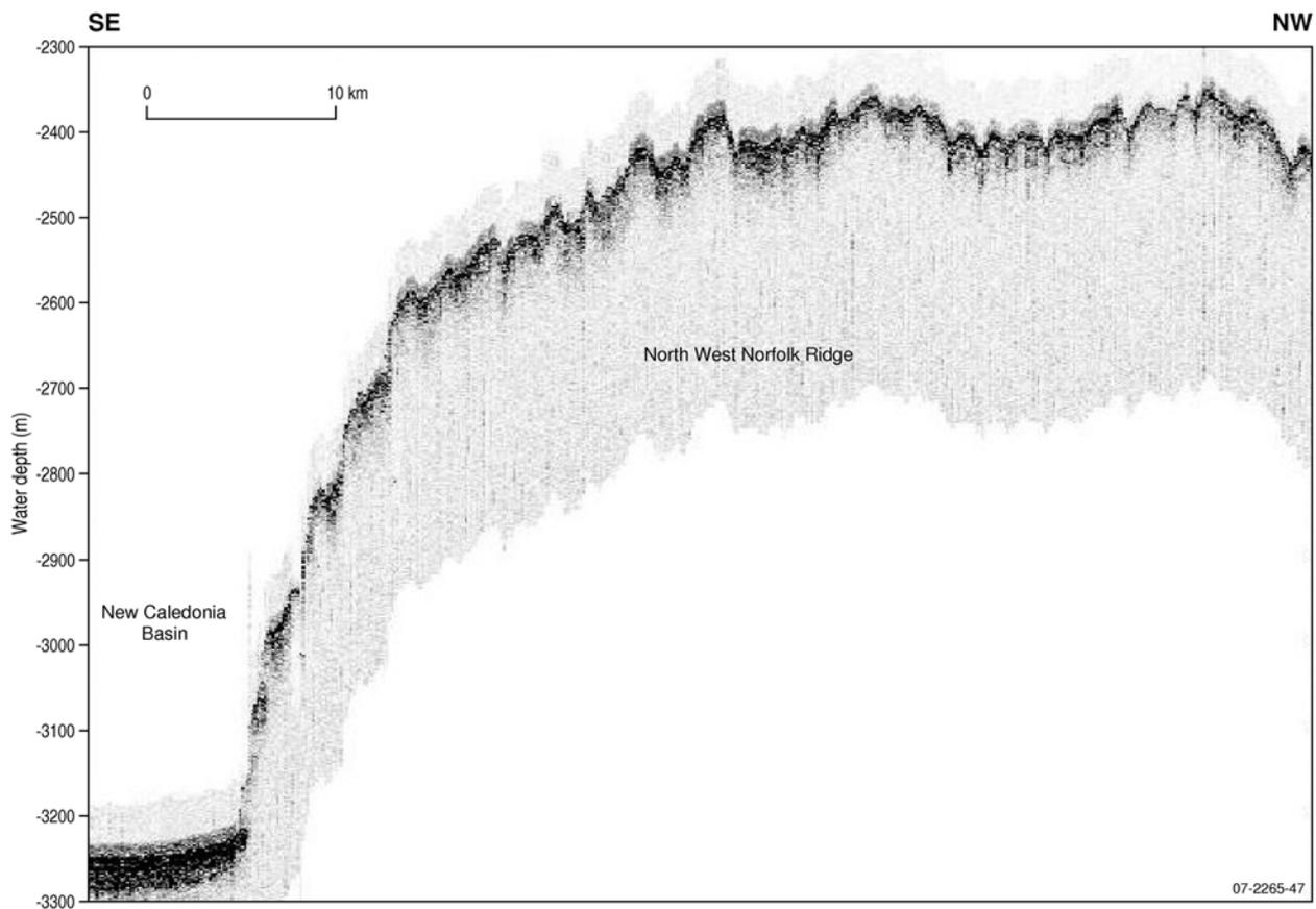
Figure 3.57. Profile of North West Norfolk Ridge showing rough topography on ridge, steep lower slope and flat floor of the Fairway Basin. Location in Figure 3.54. Colwell, (2006).
