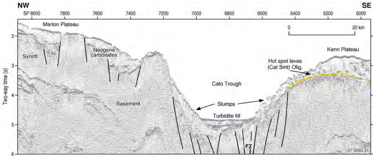
Figure 3.47. Seismic profile across the Cato Trough showing erosion, exposure of bedrock, sediment slumps on the slopes and turbidites in floor of trough. Line 11. Location in Figure 3.44. Exon *et al.*, (2005).
