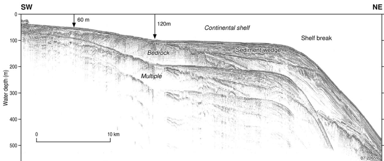
Figure 3.14. Seismic profile of the continental shelf and upper slope offshore of Barranjoey Head, Broken Bay, NSW, showing the relatively steep inner to mid shelf with rock outcrop and the outer shelf plain forming the top of the prograding sediment wedge. The location of the 60 m and 120 m isobaths are marked to show the location of the midshelf mud deposit. The shelf-break is gradual along this part of the coast at ~150 m. Location on Figure 3.11. Line 9A, (Heggie et al., 1992).
