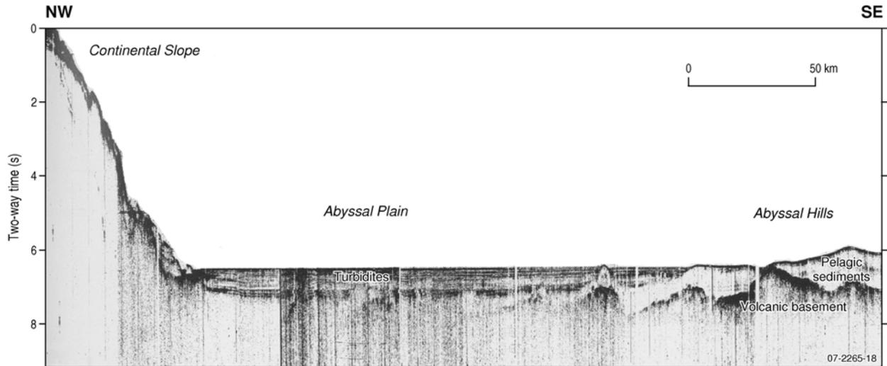
Figure 3.31. Seismic profile to the south-east of Newcastle showing the flat, near horizontal abyssal plain formed by turbidites and the sharp contact with the abyssal hills draped with pelagic sediments of the deep ocean floor region. Basaltic basement outcrops as small seamounts or where sediment is eroded. Location is on Figure 3.1. Eltanin Line 54.
