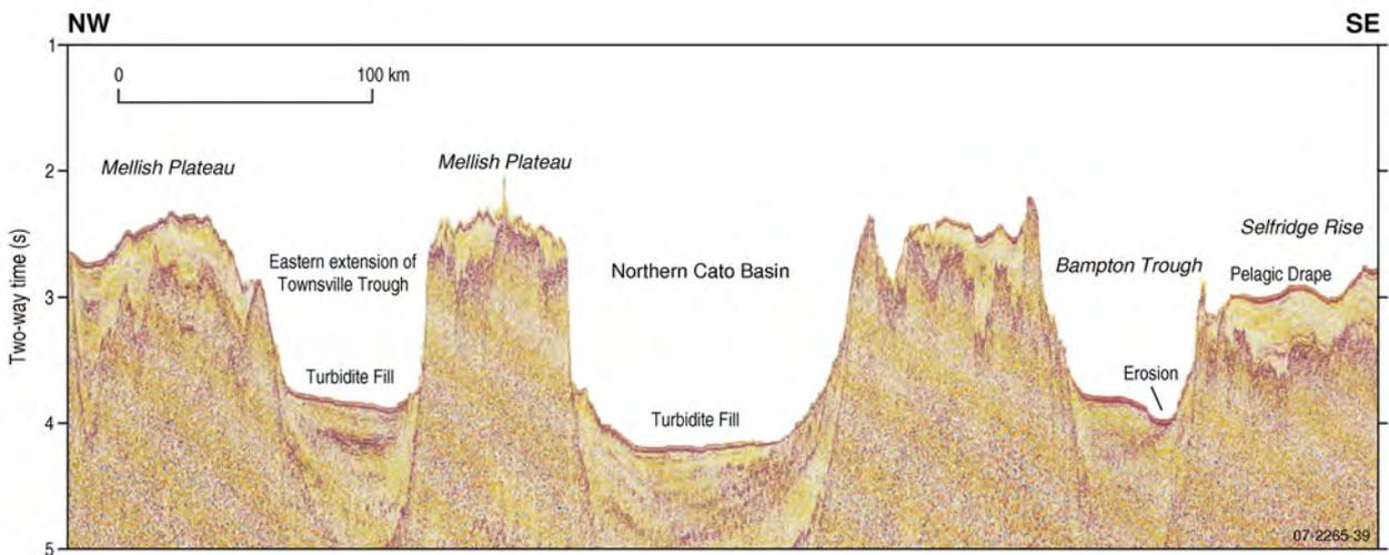
Figure 3.49. Seismic profile from Selridge Rise to Mellish Rise showing the trough and ridge topography typical in this area. Line GA274/01. Location in Figures 3.44 and 3.45. Exon *et al.*, (2006a).
