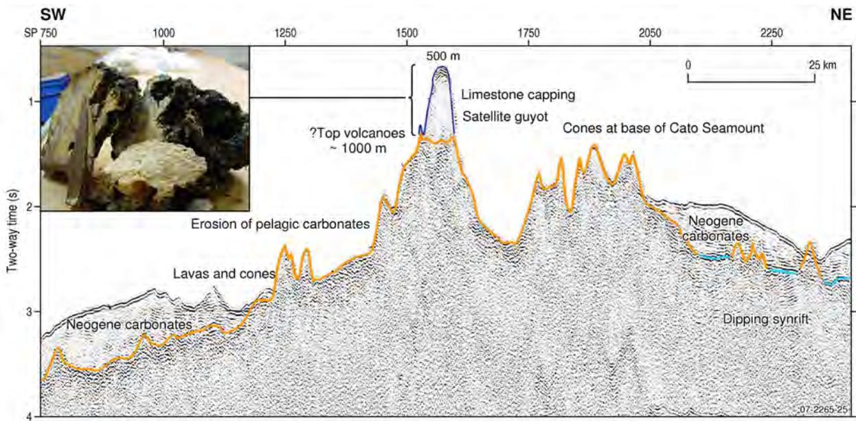
Figure 3.38. Seismic profile across Cato Seamount showing erosion, exposure of bedrock, sediment drifts and carbonate reef as a cap on the volcanic peak. Location on Figure 3.1. Line 3, Exon *et al.*, (2005).
