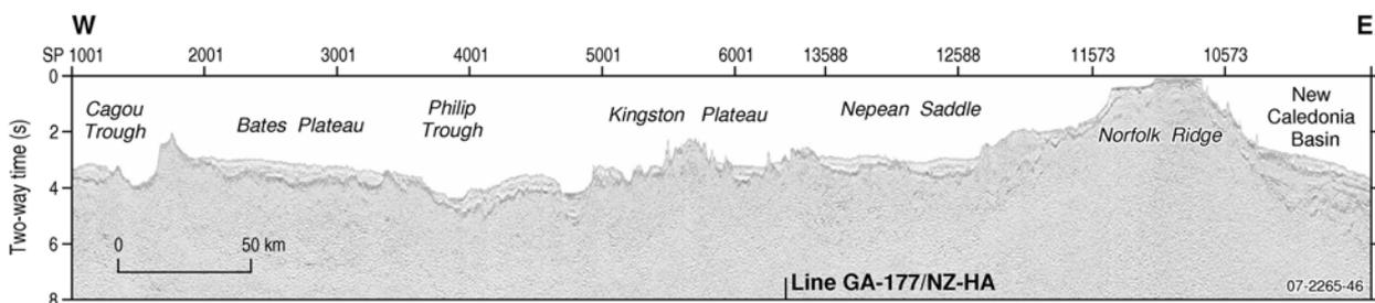
Figure 3.55. Seismic profile from the Norfolk Ridge to the eastern margin of the EMR showing the slope up from the New Caledonia Basin and the rugged topography of the ridges, troughs and plateaus. Location in Figure 3.54. Alcock *et al.*, (2006).
