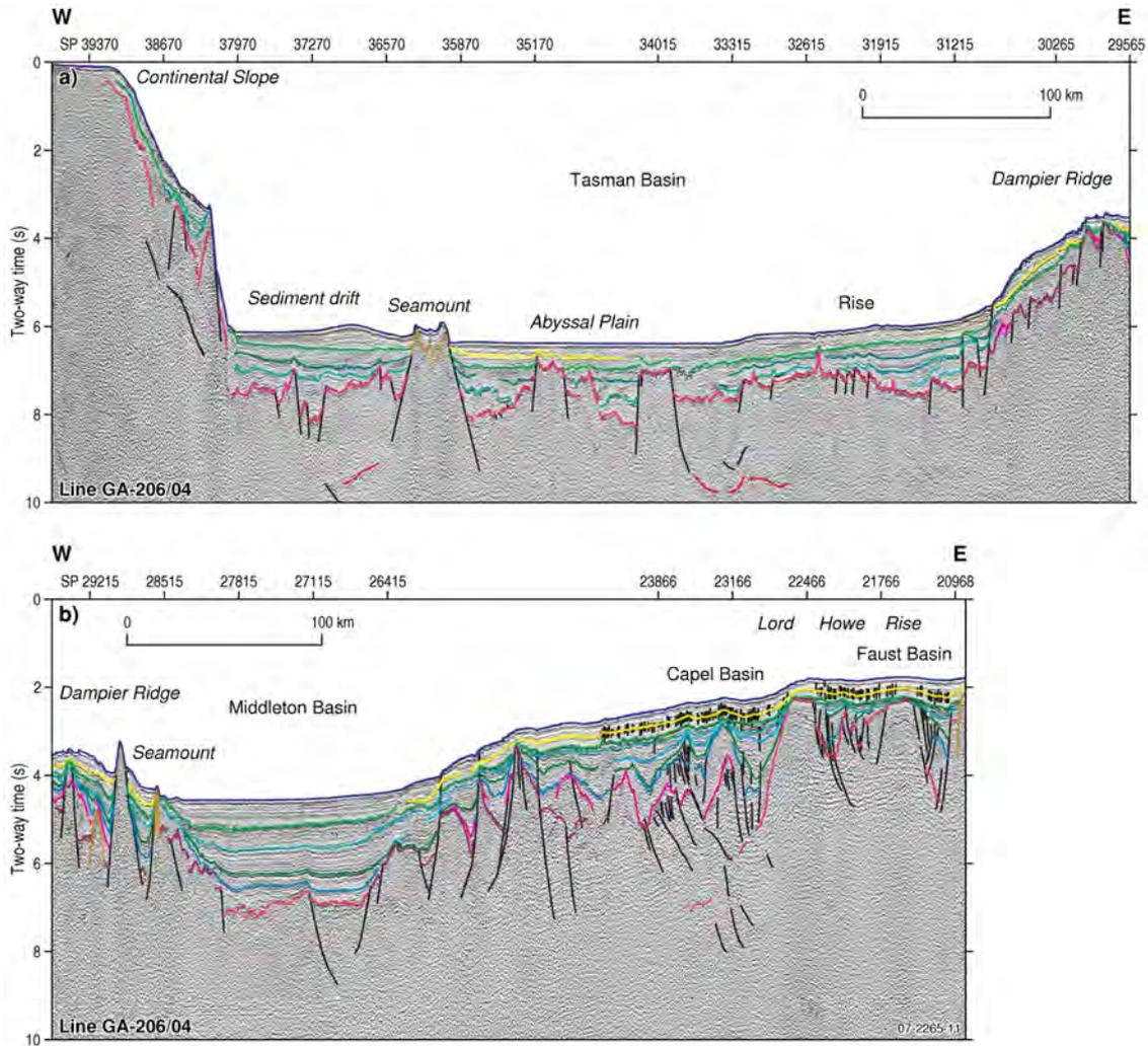
Figure 3.23. Seismic profile from Yamba, NSW, across the Tasman Basin to the Dampier Ridge. It shows the wide slope, lack of rise, abyssal plain and the rise at the foot of the Dampier Ridge. Note the drift deposit on the abyssal plain/deep ocean floor and the basement seamount. Location on Figure 3.1. (Van der Beuque et al., 2003).
