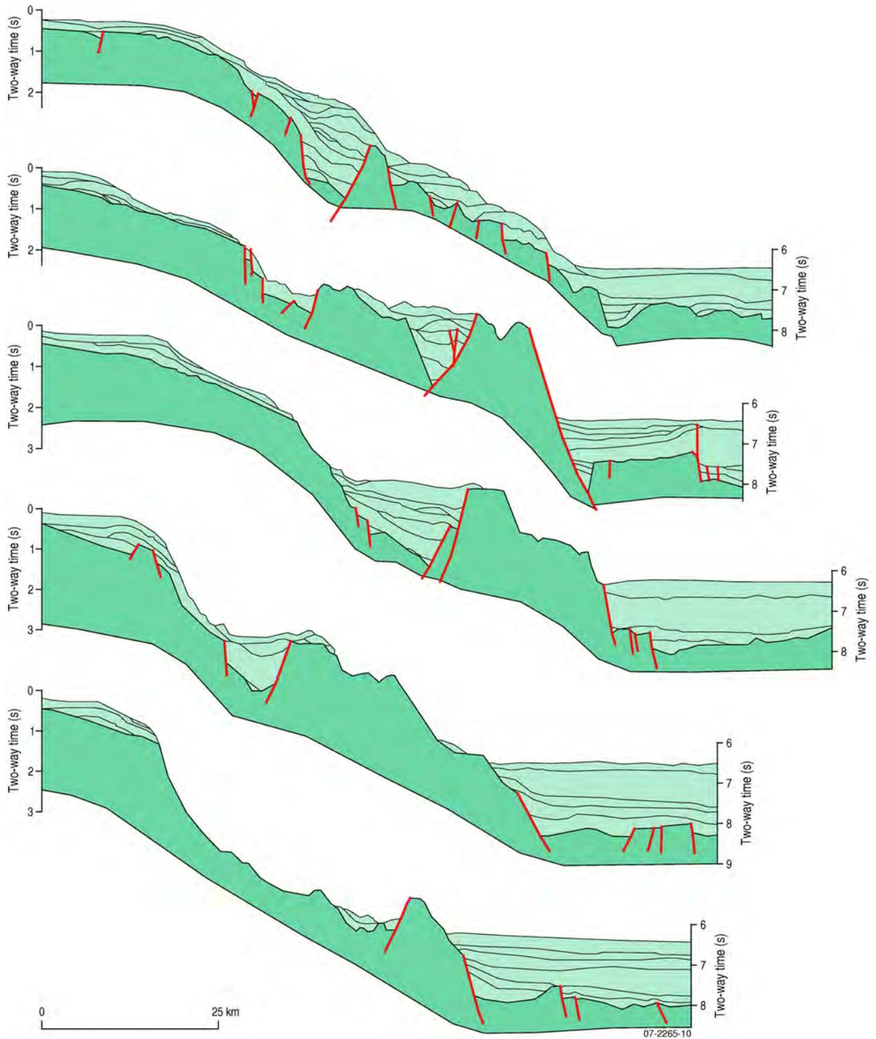
Figure 3.21. Line drawings of interpreted seismic profiles from the southern NSW slope and adjacent abyssal plain showing the relationship of sediments to basement. Note the convex upper slope with sediment wedge, concave mid-slope with erosion or sediments behind an outer ridge and a rugged and steep lower slope. BMR Survey 68, (Colwell et al., 1993).
