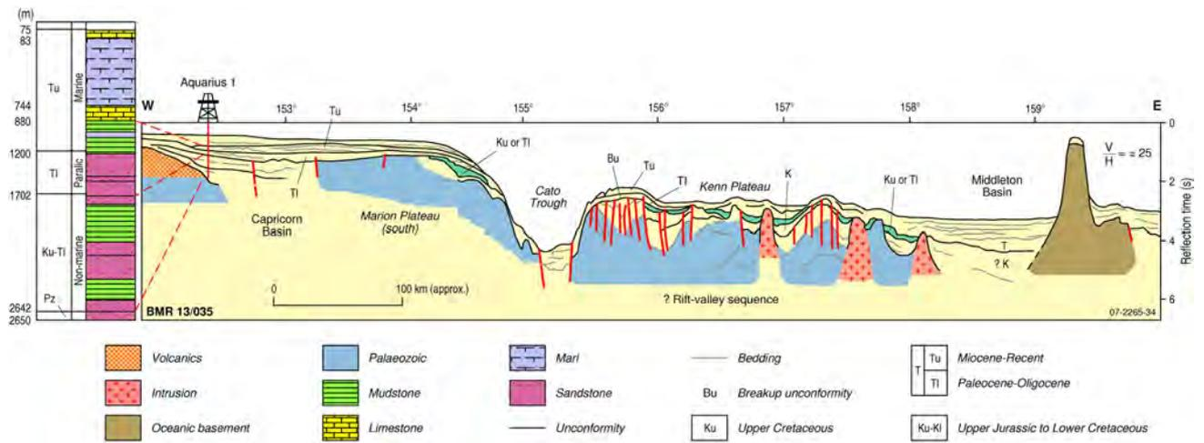
Figure 3.8. Geological and tectonic interpretation of an east-west seismic profile from the Marion Plateau to the Middleton Basin. Line BMR 13/035. Location in Figure 3.44. Willcox, (1981).
