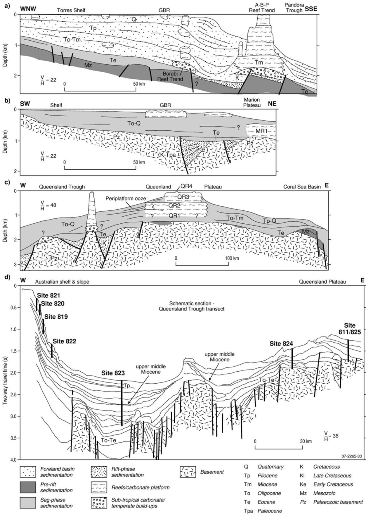
Figure 3.7. Profiles showing generalized basement structure and sedimentary sequences offshore of Queensland. Wellman et al., (1997).
