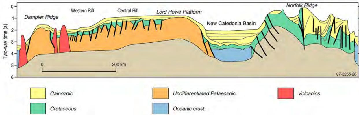
Figure 3.5. Interpreted seismic profile from the Tasman Basin across the Dampier Ridge, Lord Howe Rise, New Caledonia Basin and Norfolk Ridge showing how the tectonic elements of the rifted crust, oceanic crust and volcanics determine the geomorphic features. Note the relatively steep lower slopes, the thick sediment caps on highs and sediment fill in basins. (Alcock et al., 2006).
