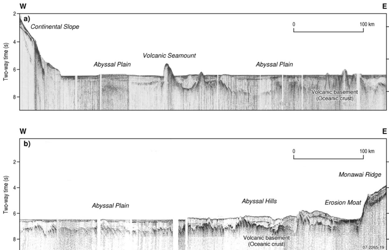
Figure 3.32. Seismic profile from the shelf off Newcastle across the Tasman Basin to the southern Lord Howe Rise. a) The seismic profile to the east of Newcastle shows the flat slightly convex-up abyssal plain. Note the broad moats at the base of the small seamounts of basement rock and b) Pelagic sediments in the eastern part of the basin show draping on underlying
