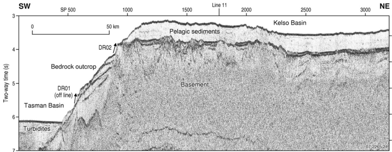
Figure 3.34. Seismic profile showing abyssal plain turbidites in sharp contact with the steep margin of the Kenn Plateau north Tasman Basin. Note the sediment blanket on the plateau. Location is on Figure 3.1. Line 270-7, Exon et al., (2005).
