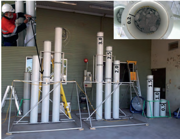
Figure 4.8 Set up of the radon columns at the Jabiru Field Station (photo: Safe Radiation 2013)
