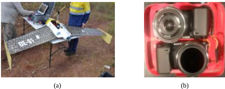
Figure 4.2 (a) The Swampfox preparing for flight, and (b) the RGB and NIR camera payload.
