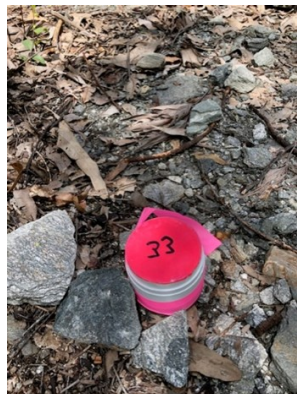
Images 8-9 (left to right): Image 8, Passive sampling device for radon exhalation; Image 9, measurement results to date
