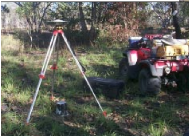
Figure 2 (above) Mobile rover dGPS receiver mounted on a 4WD quad bike; Figure 1 (left) Base station set up
