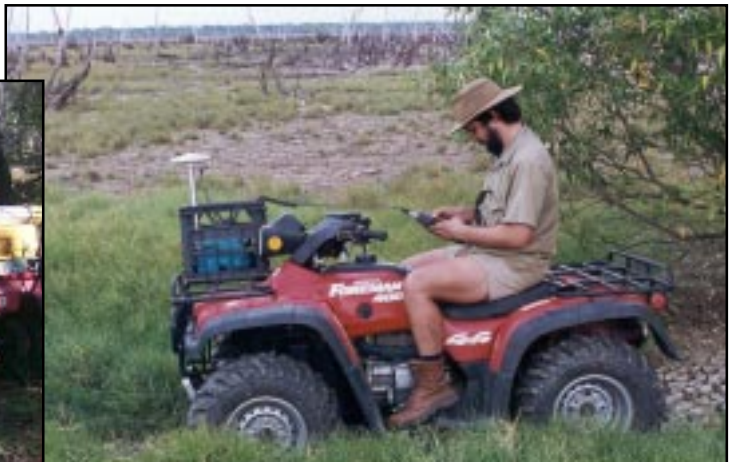
Figure 2 (above) Mobile rover dGPS receiver mounted on a 4WD quad bike; Figure 1 (left) Base station set up
