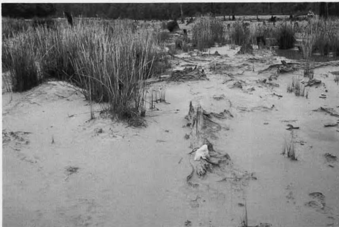
Plate 9 Fresh sulphidic tailings on the surface of Bank D overlying more oxidised sediment. Poned water on the bank indicates the occurrence of near-surface clay layers.
