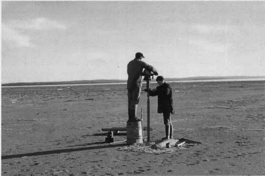
Plate 5 Hand-held sonic drilling equipment deployed on the north lobe of the delta for the installation of DEL-C1. The view is to the south-east towards Macquarie Harbour.
