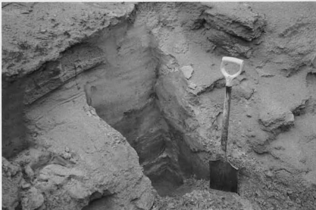
Plate 6 Vertical profile through part of the unsaturated zone in Bank H along the edge of the King River. The relatively unoxidised blue-green material is discontinuous in all directions. Oxidation was probably retarded by the local retention of perched groundwater above a clay-rich horizon.
