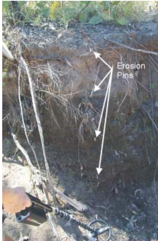
**Figure 3** Metal detector used to relocate buried pins. Tributary Central cross section TC6B during the dry season when the water table is at least 0.5 m below the river bed. Bank profile is vertical. Compare with wet season conditions in fig 4.
