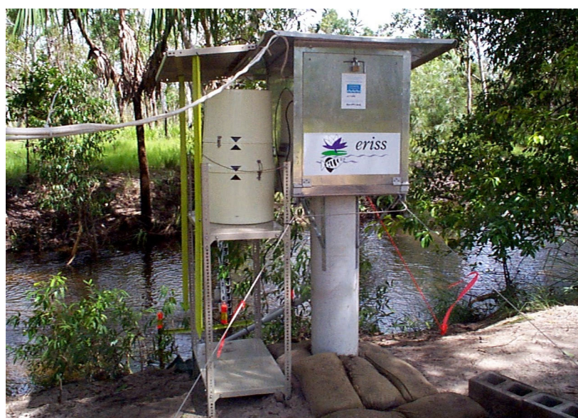
Figure 2 SC gauging station. A second APS is shown located outside the shelter.
