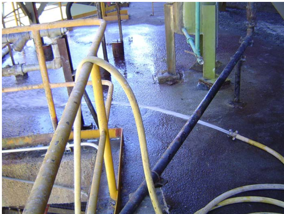
1" flattened hose when discharging Photograph 10
