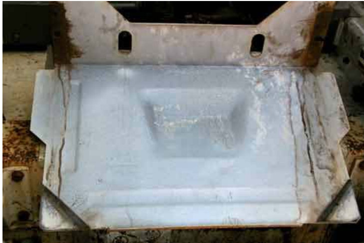
Figure 4 Close up of material deposited inside bobcat cabin
