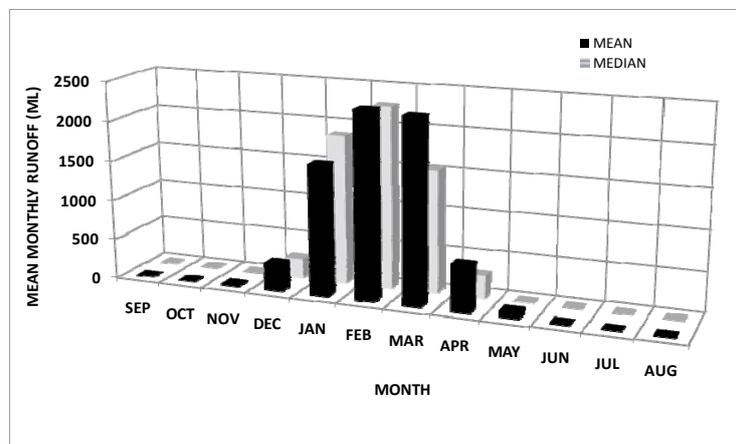
**Figure 6** Mean monthly runoff at the East Tributary gauge for the common period of record, 1998–2007. See Figure 1 for location of the site.
