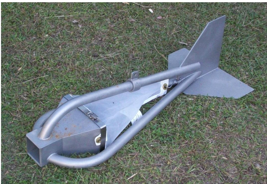
**Figure 2** Helley-Smith BLS 30 pressure difference bedload sampler designed for operation with a winch on a cableway (photo by Tony Walker)
