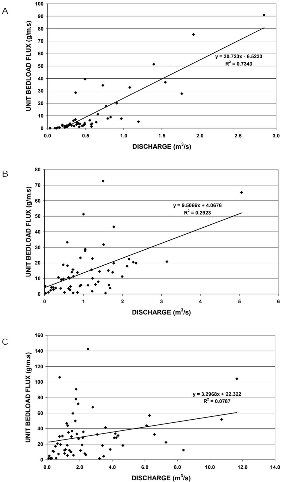
**Figure 11** Rating curves of bedload flux per unit bed width and unit time versus discharge at (A) East Tributary gauge, (B) Upper Swift Creek gauge and (C) Swift Creek gauge
