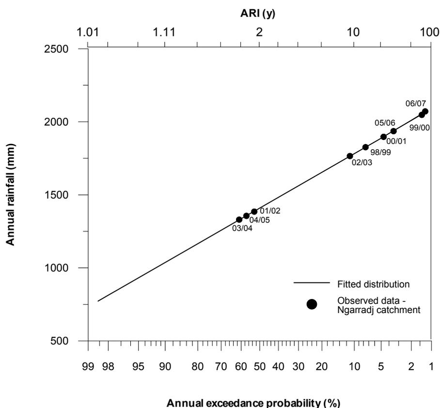
**Figure 4** Annual rainfall frequency curve for Oenpelli (from Moliere et al 2002a) showing the total annual Ngarradj catchment rainfall for the nine years of record, 1998–2007. ARI = average recurrence interval. See Fig 1 for location of Oenpelli and the Ngarradj catchment.
