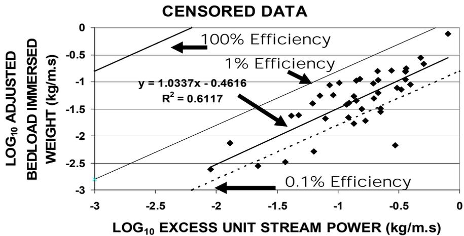
**Figure 18** Significant regressions on censored bedload data for Swift Creek gauge with an adjusted  $R^2 > 0.60$ . (A) Bedload flux versus discharge, (B)  $\text{Log}_{10}$ -transformed adjusted bedload immersed weight and unit stream power and (C)  $\text{Log}_{10}$ -transformed adjusted bedload immersed weight and excess unit stream power.
