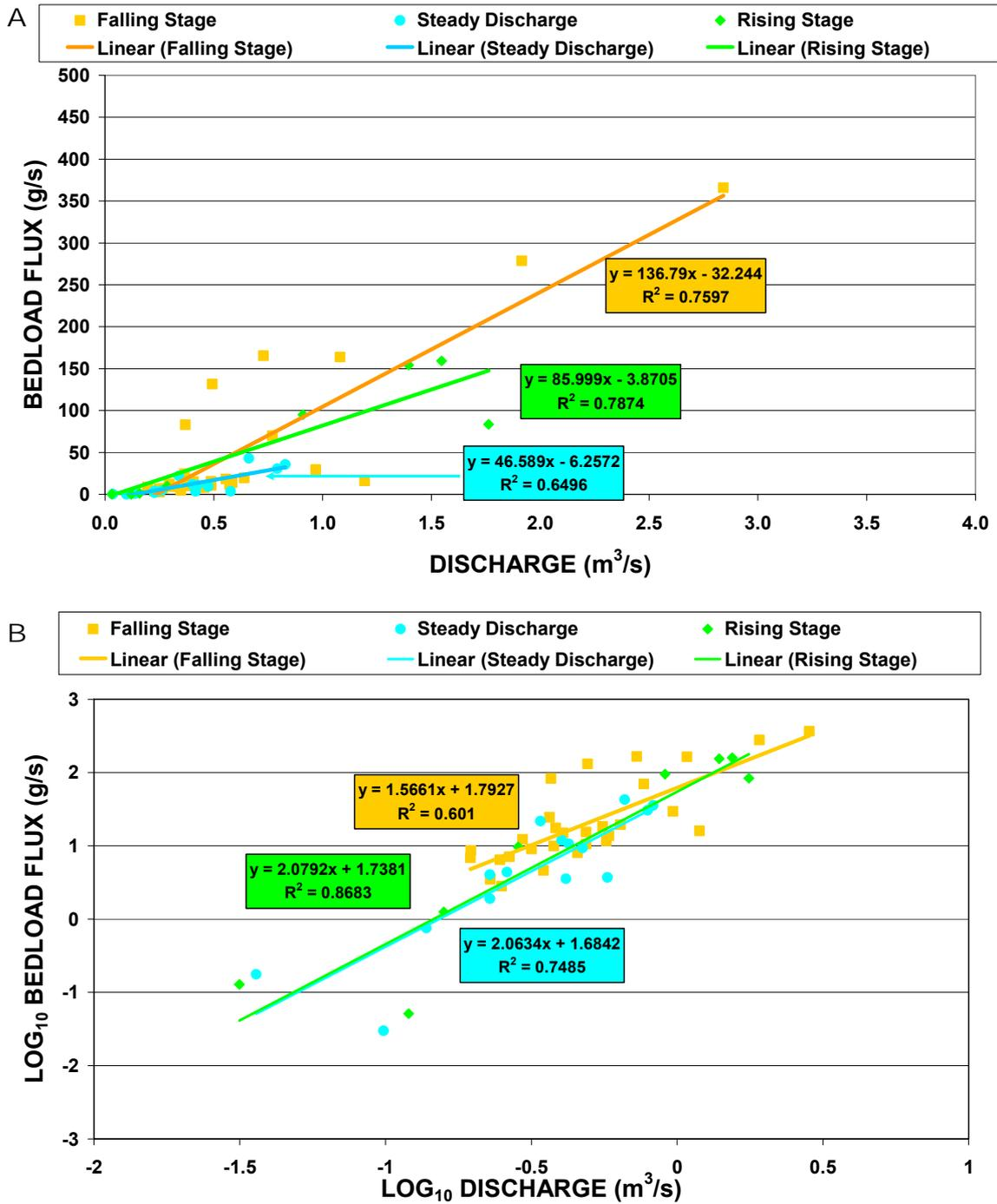
**Figure 12** Bedload ratings for (A) raw and (B)  $\log_{10}$ -transformed data for falling stage, steady discharge and rising stage at East Tributary
