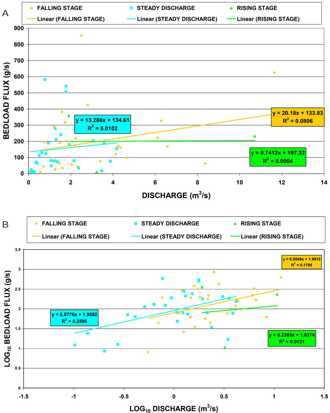
**Figure 14** Bedload ratings for (A) raw and (B)  $\log_{10}$ -transformed data for falling stage, steady discharge and rising stage at Swift Creek
