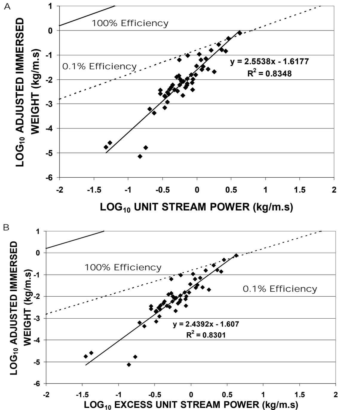
**Figure 16** Relationships between log<sub>10</sub> adjusted immersed weight and (A) log<sub>10</sub> unit stream power, and (B) log<sub>10</sub> excess unit stream power for the East Tributary gauge
