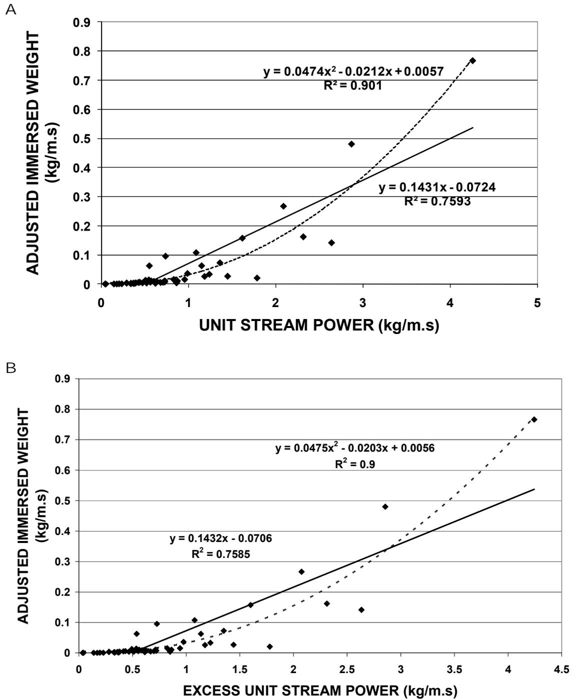
**Figure 15** Relationships between adjusted immersed weight and (A) unit stream power, and (B) excess unit stream power for the East Tributary gauge
