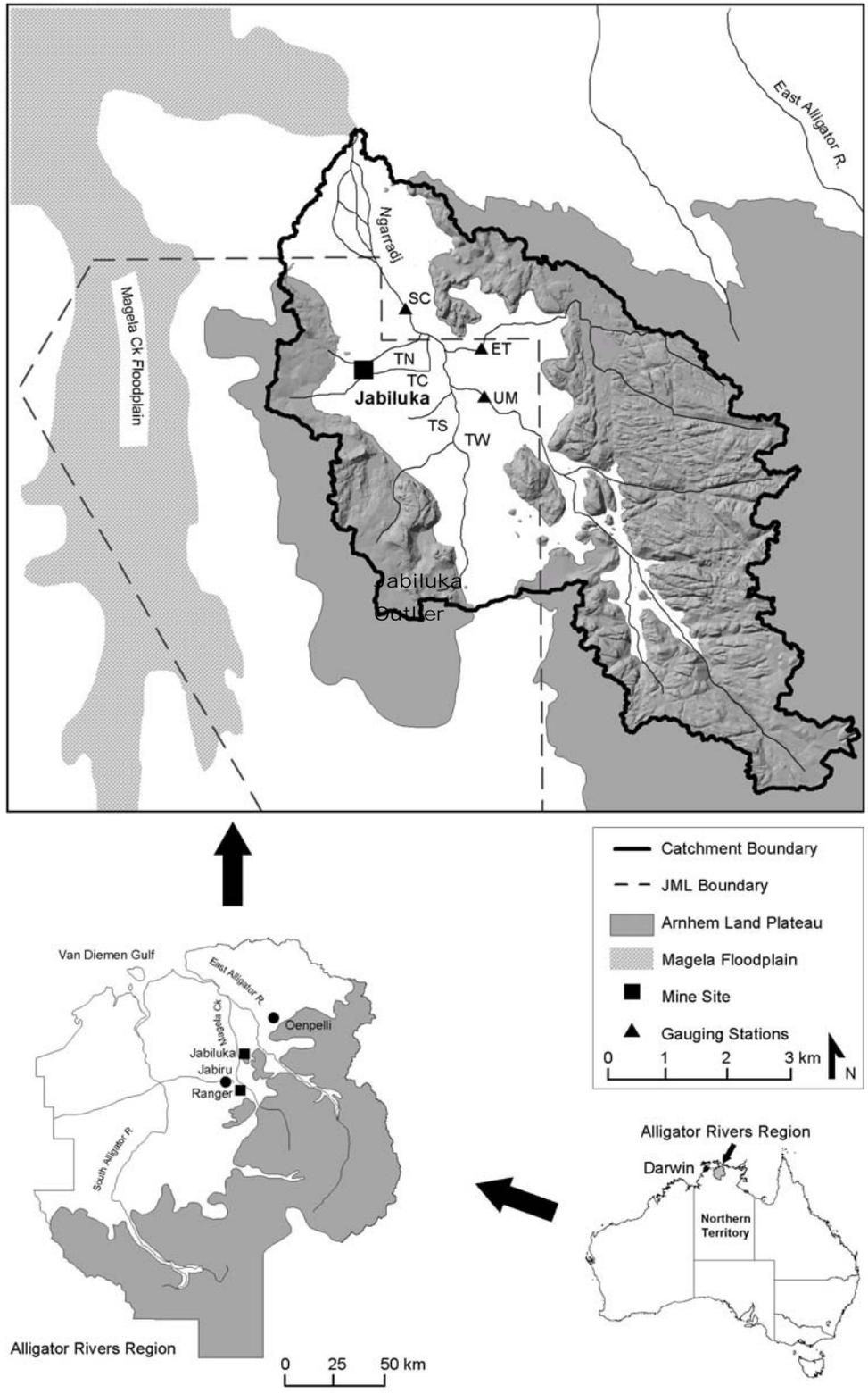
**Figure 1** Ngarradj Creek catchment at Jabiluka, Northern Territory, Australia. ET refers to the East Tributary gauge, UM the Upper Swift Creek gauge, SM the Swift Creek gauge, TN Tributary North, TC Tributary Central, TS Tributary South and TW Tributary West. JML refers to the Jabiluka Mineral Lease and the rest of the land to the west of the East Alligator River is Kakadu National Park.
