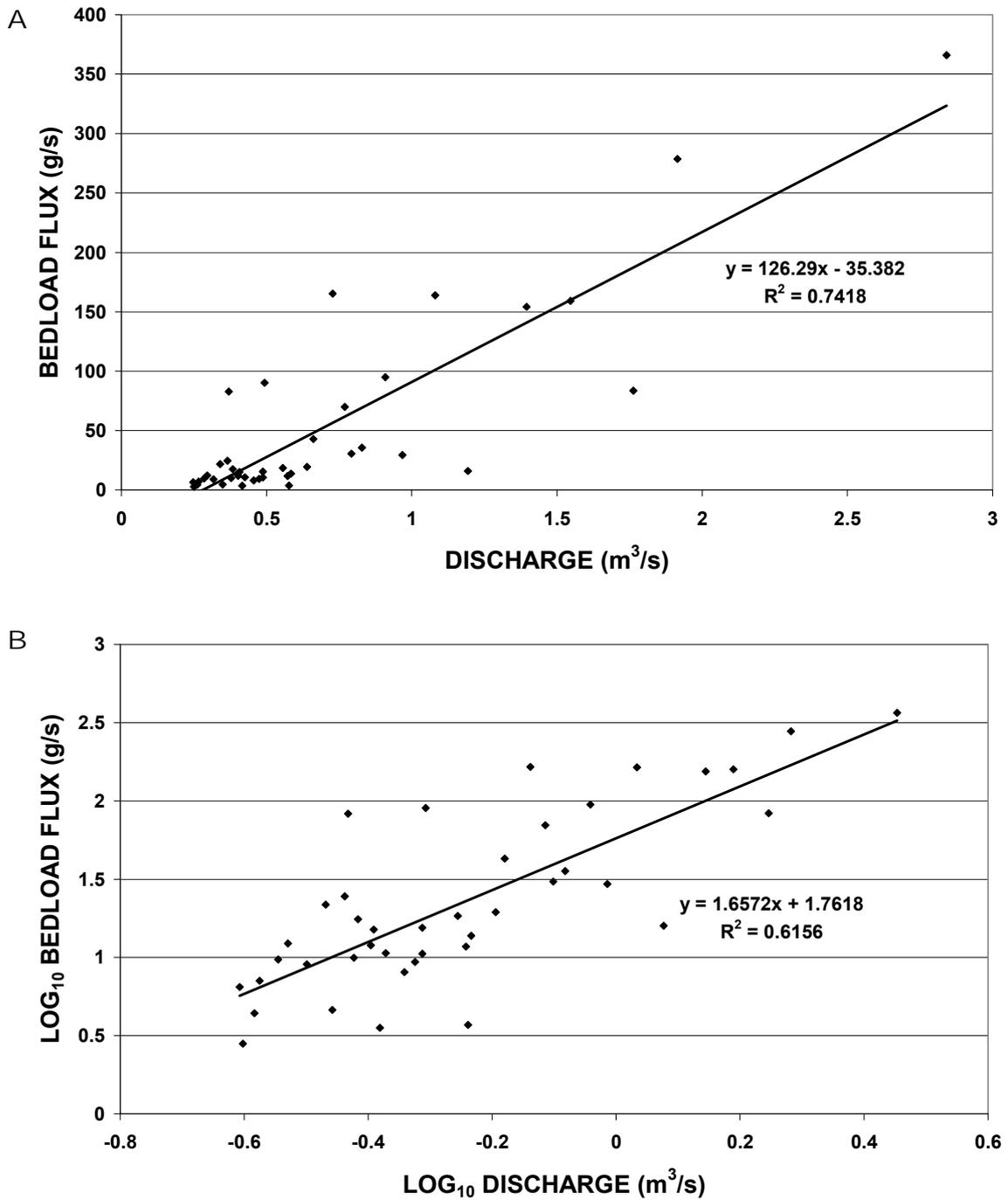
**Figure 10** Bedload ratings on (A) raw data and (B) log<sub>10</sub>-transformed data with values deleted below a discharge of 0.223 m<sup>3</sup>/s at East Tributary
