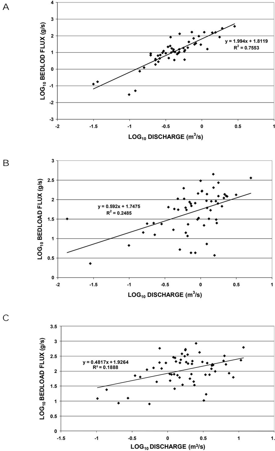
**Figure 9** Bedload rating curves on  $\text{log}_{10}$  data at (A) East Tributary gauge, (B) Upper Swift Creek gauge and (C) Swift Creek gauge
