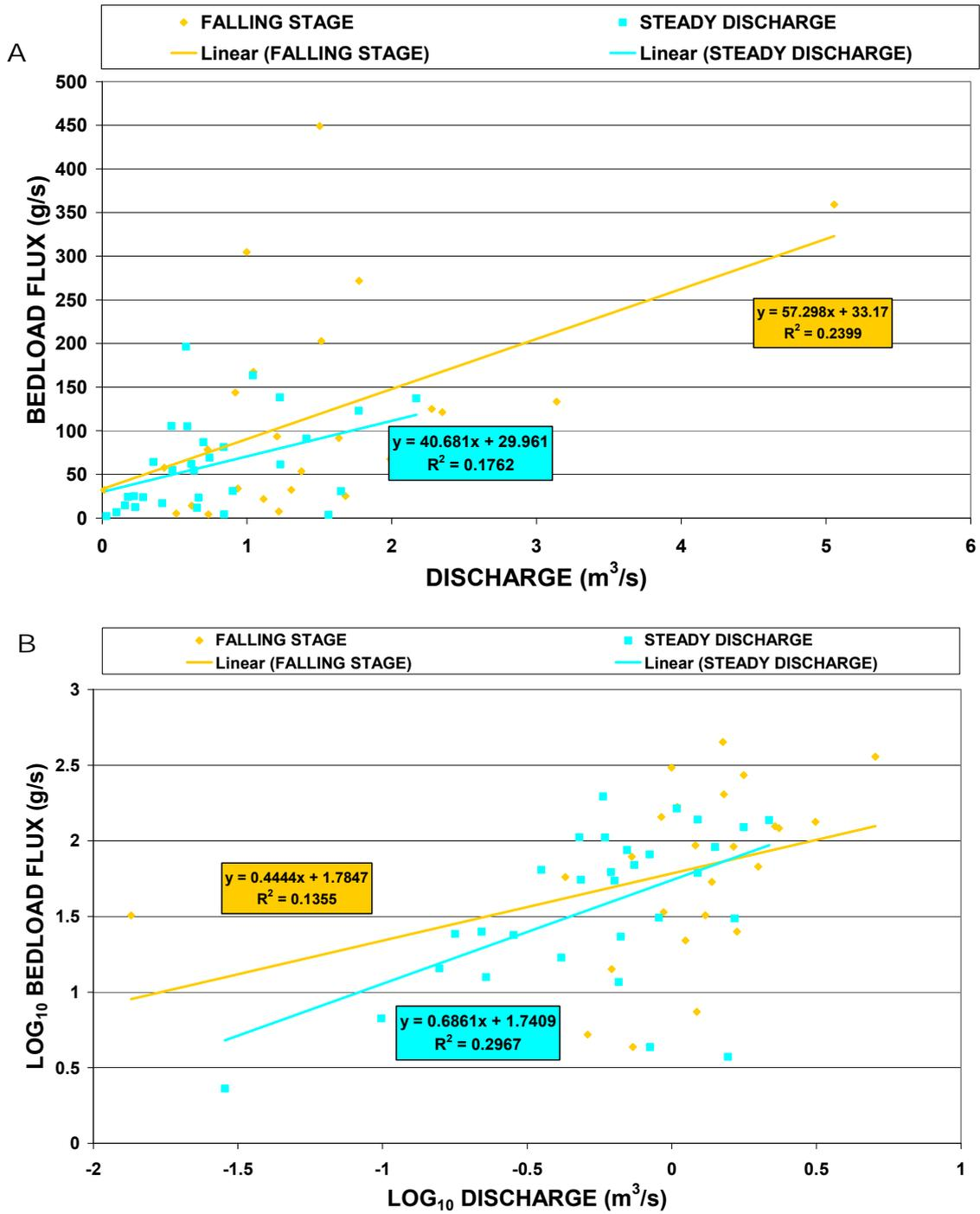
**Figure 13** Bedload ratings for (A) raw and (B) log<sub>10</sub>-transformed data for falling stage and steady discharge at Upper Swift Creek
