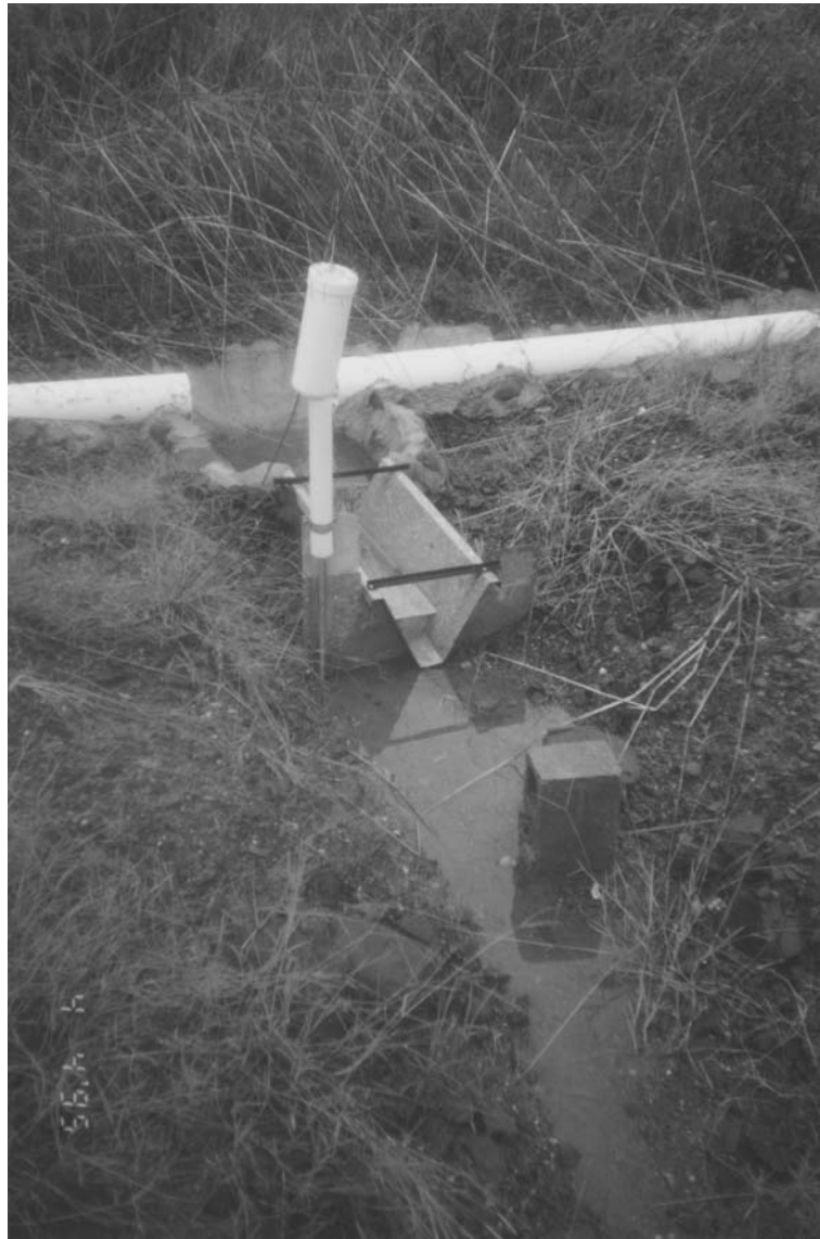
Figure 4 RBC flume on an earlier erosion plot at Ranger. In the plots on the demonstration land form the flume will be located at the left end of the plot near the edge of the landform.
