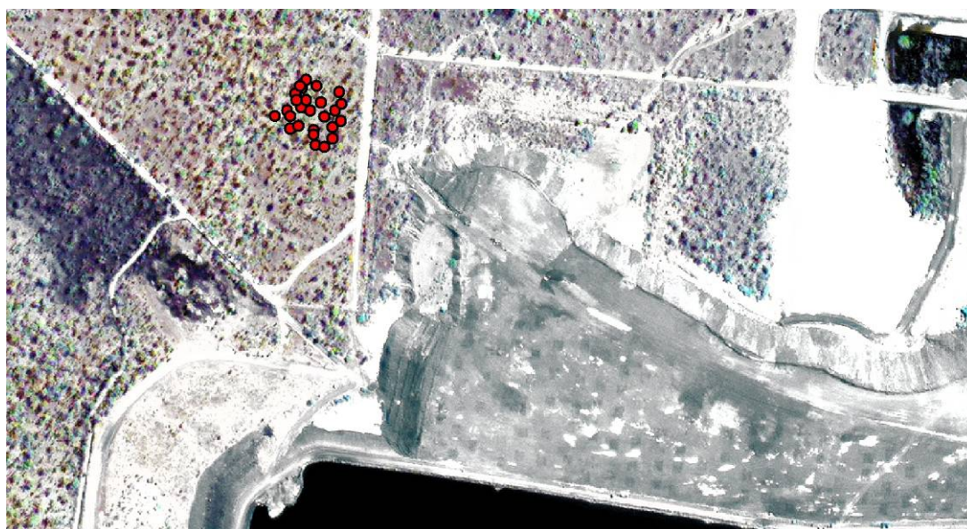
Figure 1 Location of the radon exhalation survey and individual charcoal cup locations. The north western corner of the tailings dam can be seen at the bottom of the picture.
