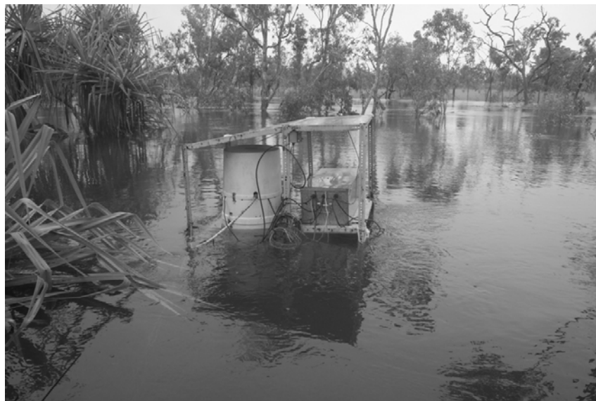
Figure 1 Gauging station at GCDS submerged by floodwaters during the March 2007 flood. This photo was taken several hours after the flood peak when waters were at least 0.5 m higher than that shown here.
