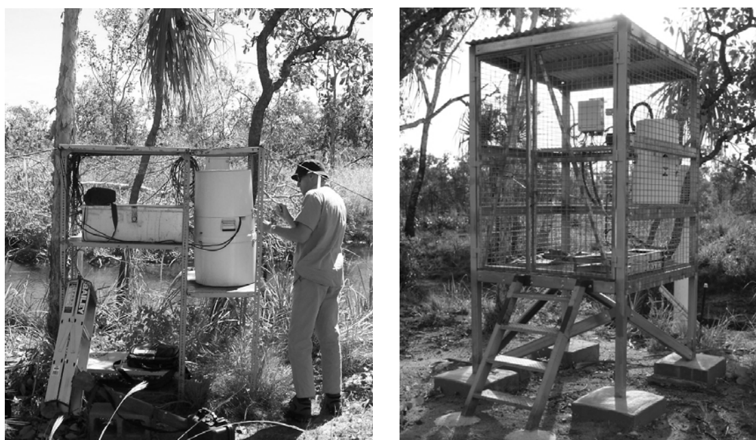
Figure 2 Original station at GCUS (left) and the new permanent gauging station constructed late in the 2007 dry season (right)
