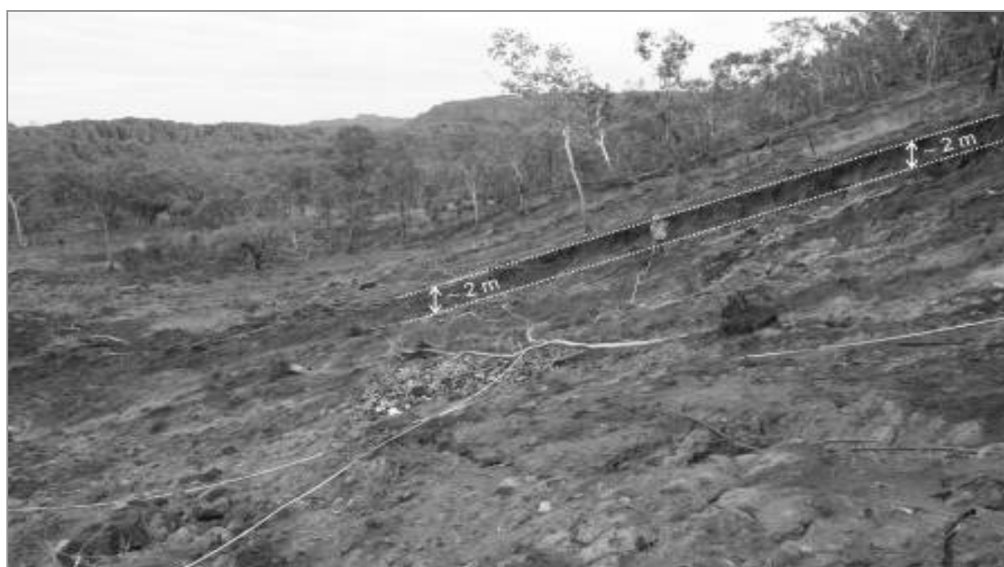
Figure 2 Field measurement of the one of the landslips in the Upper Magela Catchment. The approximate depth of the landslide at 2 m is illustrated.
