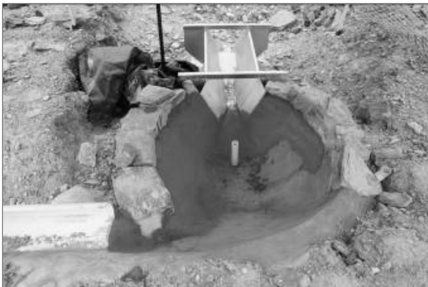
Figure 4 Reservoir and flume at the outlet of the erosion plot
