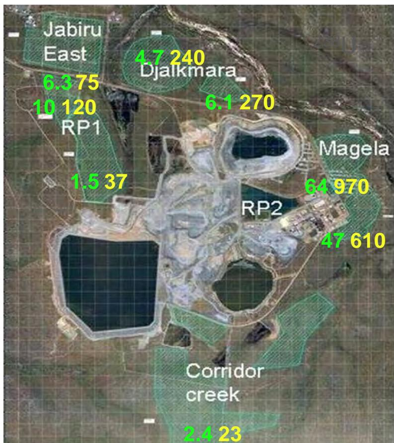
**Figure 1**  $^{238}\text{U}$  (yellow – white in printed copy) and  $^{226}\text{Ra}$  (green – grey in printed copy) aerial activity densities ( $\text{kBq}\cdot\text{m}^{-2}$ ) calculated from historical radionuclide inventories in RP2 water and irrigation rates provided by ERA (from Akber et al 2010)
