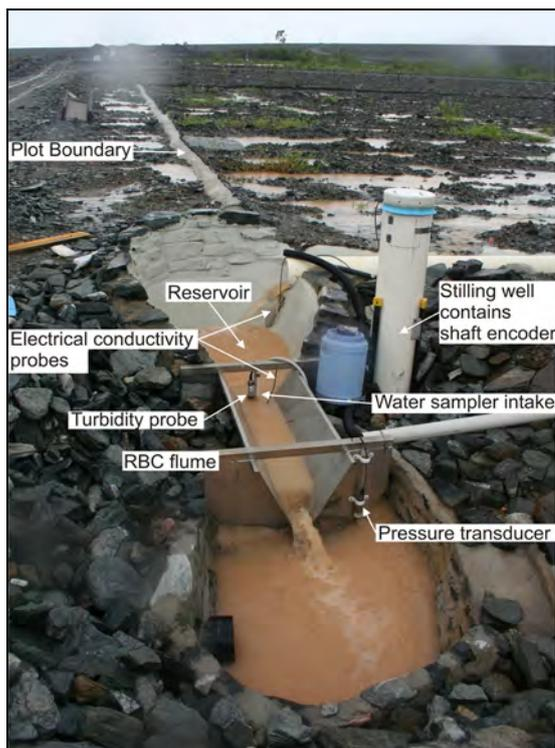
**Figure 3** Runoff through flume on trial landform erosion plot 3 during a storm event
