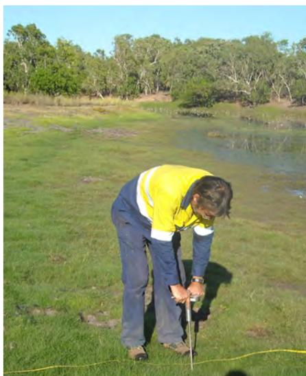
**Figure 2** Penetrometer being used in Malabanbandju Billabong
