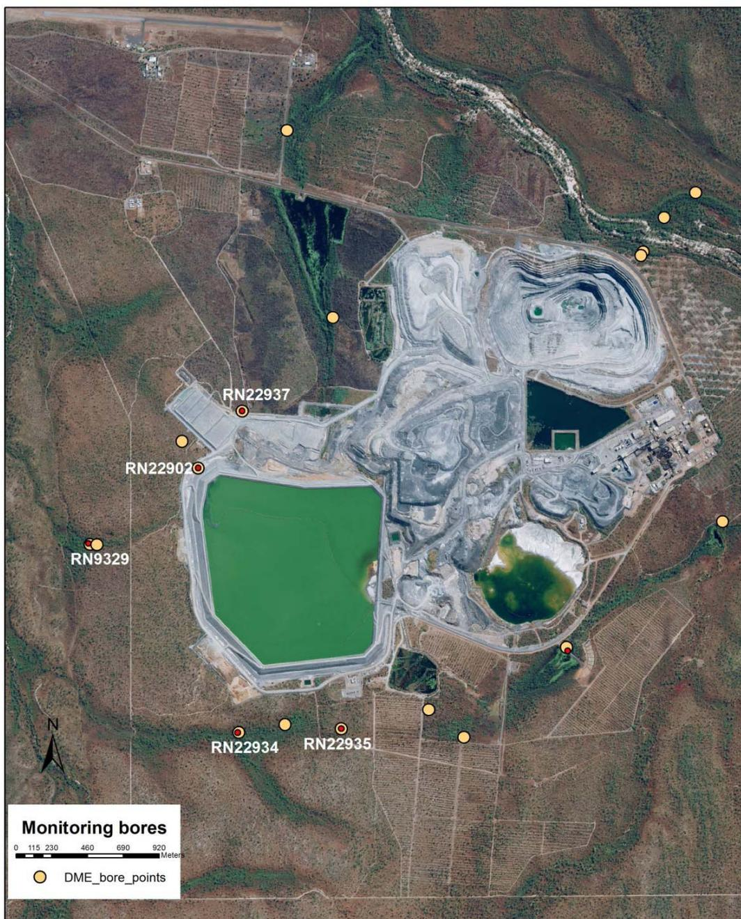
**Figure 1** Aerial photograph of Ranger mine with monitoring bore locations sampled by DME
