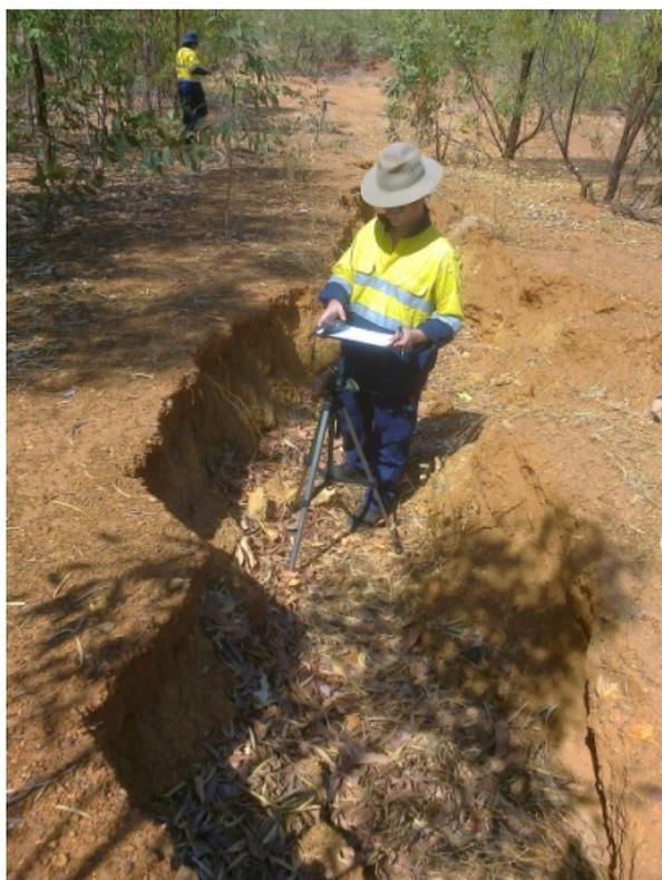
**Figure 5** Measurement of the gamma dose rate in an erosion gully at the containment
