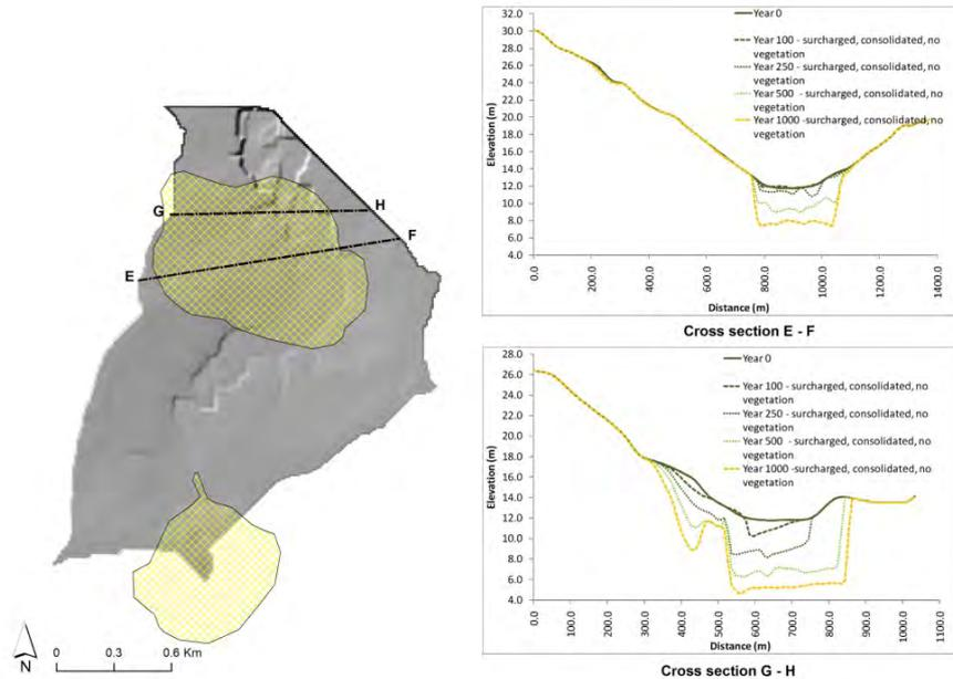
**Figure 3** Unvegetated ('worst case') 1000 year surface of Djalkmara Creek catchment. Hatched areas represent current extent of Pit 1 (lower) and Pit 3 (upper).
