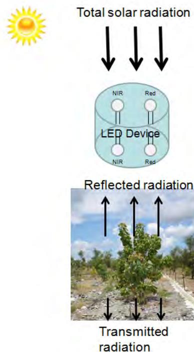
**Figure 4** Illustration of how the LED device is able to measure both incident and reflected radiation
