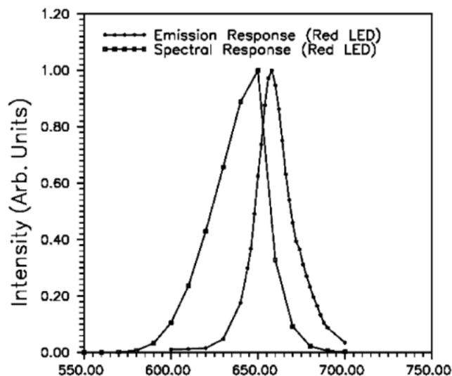
**Figure 1** Emission and spectral sensitivity response for a typical LED
