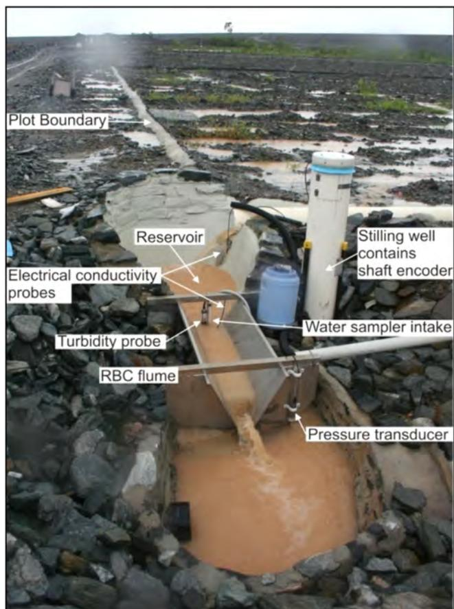
**Figure 2** Runoff through the flume on the trial landform erosion Plot 3 during a storm event
