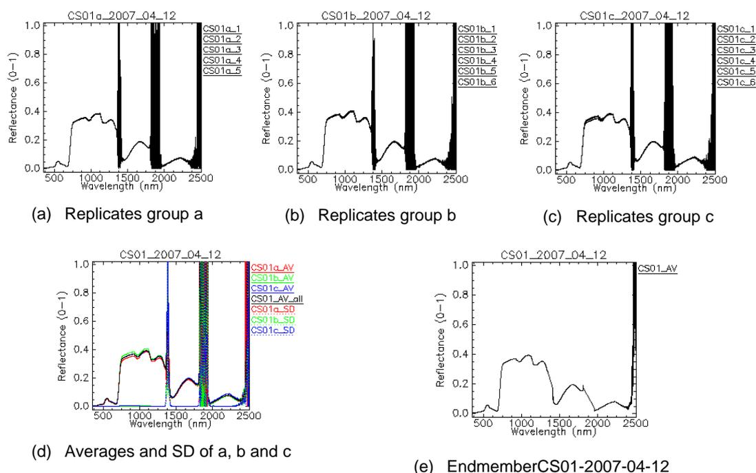
**Figure 2** The processing of spectra for one species of one date.
