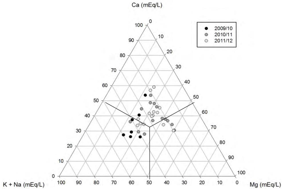
**Figure 6** Ternary plot showing cation (mEq/L) composition of surface water runoff over the 2009–10 (black), 2010–11 (dark grey) and 2011–12 (light grey) wet seasons
