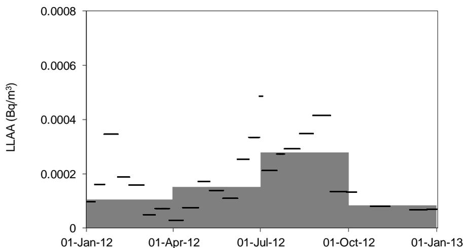
**Figure 4** Measured (black lines) and quarterly average (grey columns) concentrations of dust-bound LLAA radionuclides in air at Jabiru town in 2012
