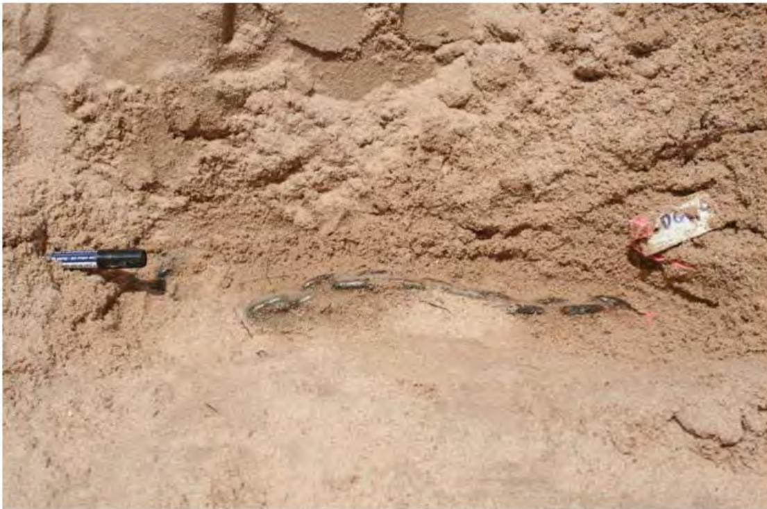
**Figure 7** Excavated scour chain 1 at cross section DG11 on 12 December 2007. Flow direction is from left to right.
