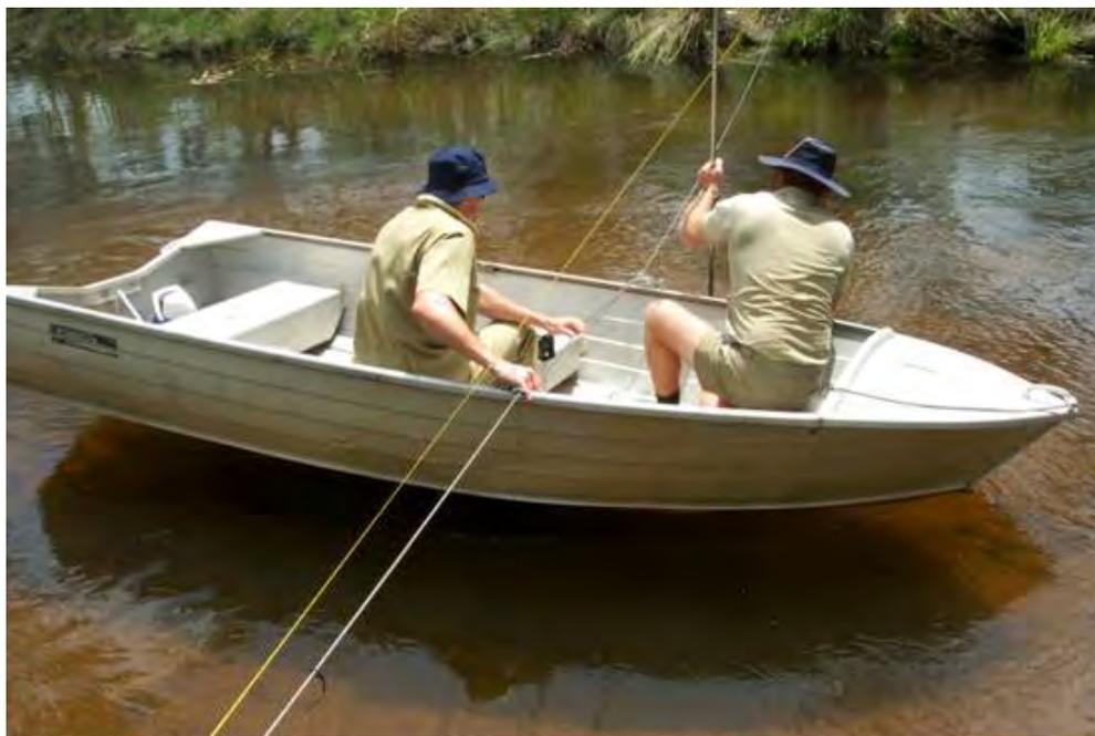
**Figure 1** Velocity-area gauging using a current meter and wading rod out of a boat at the gauging wire at G8210012 on 8 February 2005. A number of gaugings are needed to construct a rating curve (water surface elevation or stage on the gauge board versus discharge) to convert the stage record to discharge.
