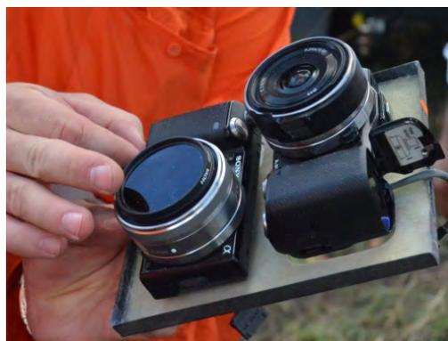
**Figure 3** The modified digital cameras carried onboard Swampfox.
