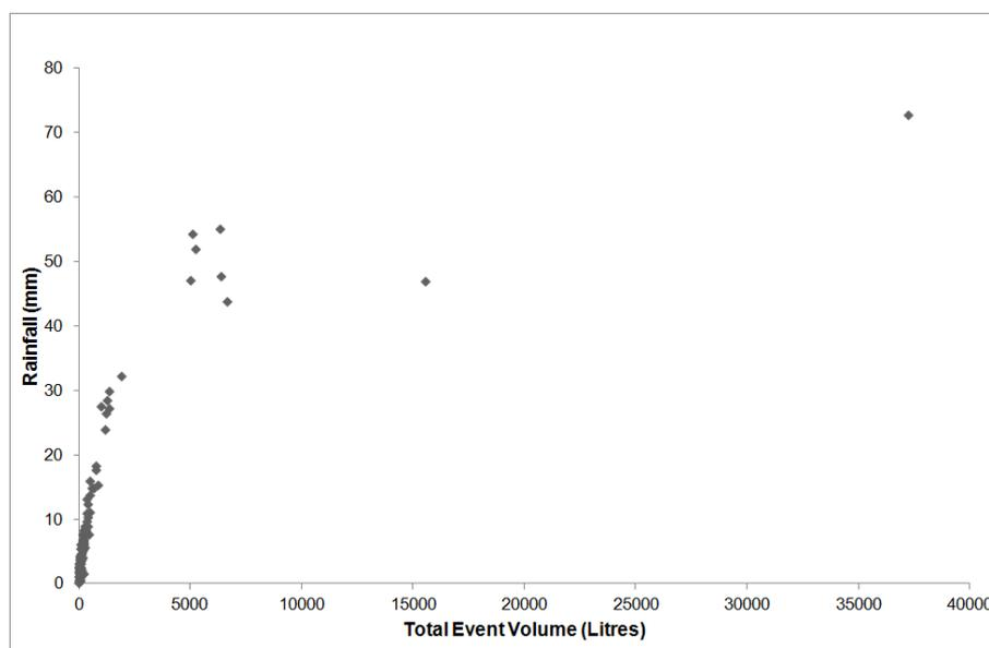
**Figure 3** Relationship between total event rainfall and runoff for Plot 1 for every runoff event in the 2012–13 water year
