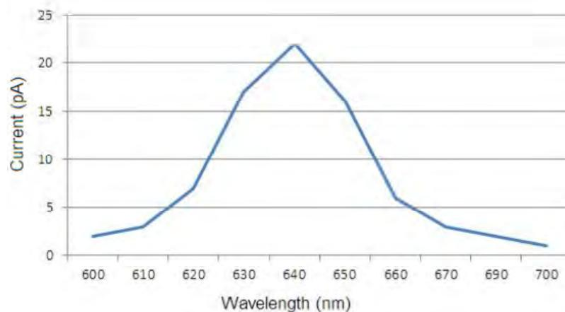
**Figure 3** LED sensitivity curve
