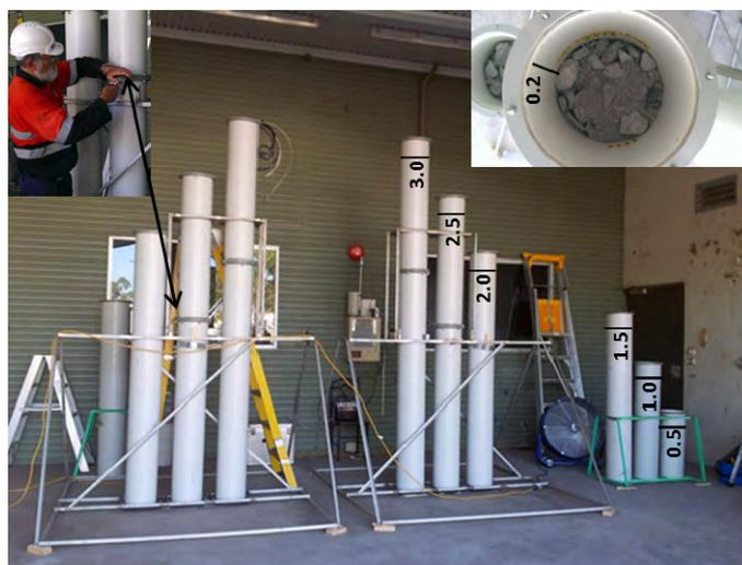
**Figure 1** Set up of radon column experiment at Jabiru Field Station, April 2013 (photo from SafeRadiation (2013)).
