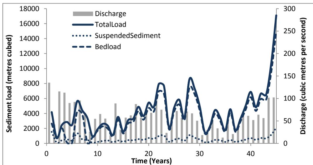
**Figure 4** Variation in bedload and suspended load in the unvegetated Djalkmara catchment over the 45 year period. The largest historical storm occurred in year 45.
