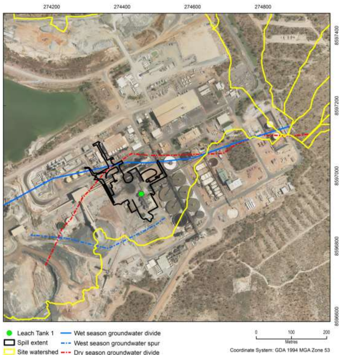
Figure 14. Site watershed (data provided by SSD) compared to wet and dry season groundwater divides (Alarcon Leon et al., 2007a). Note that the location of the surface watershed implies that all surface flow from the plant area exposed to spill material will flow to RP2, while the groundwater divides sit directly under the spill-affected area
