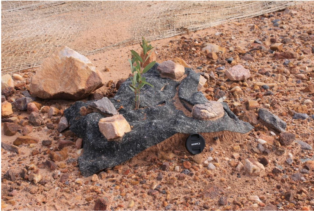
Figure 6 Protective matting has prevented the erosion of sediment underneath it, whilst surrounding sediment has been transported away. Image taken 20-2-2014
