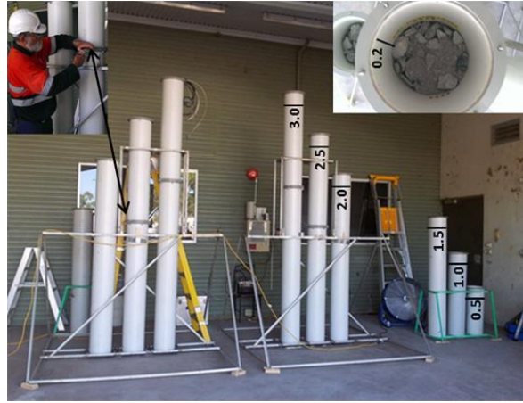
Figure 1 Set up of the radon columns at the Jabiru Field Station (photo: Safe Radation 2013).
