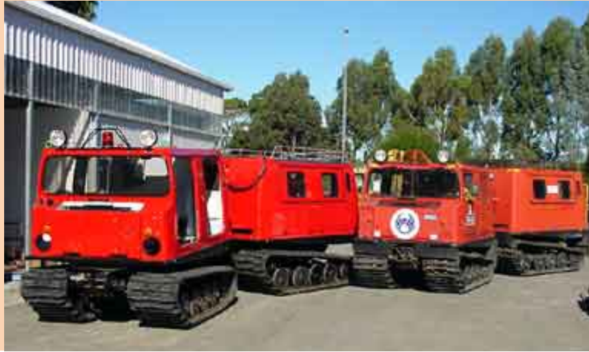
Hagglunds at Kingston: the old (right) and the 'reborn' during a total overhaul known as a 're-life' (left). (Photograph by M. Filipowski)
