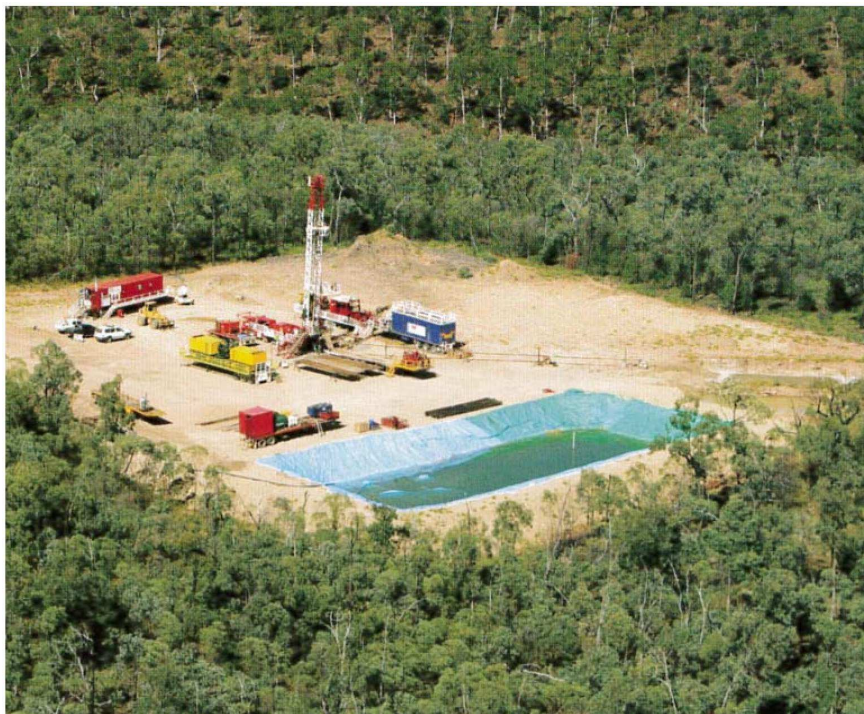
Figure 2.4 Origin lease site showing a drilling rig and temporary water storage in an excavated ground pit
