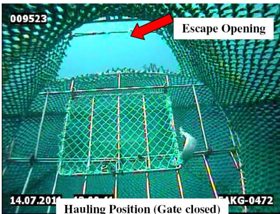
Figure 2: Acoustic-release gate in open and closed positions. The gate is held open by the acoustic actuator while the net is towed through the school of fish, allowing the fish to pass into the codend. Once the boat has finished towing through the school of fish, the gate is released (triggered from the boat) before the net is hauled (through seal diving range depths) and brought onboard.
