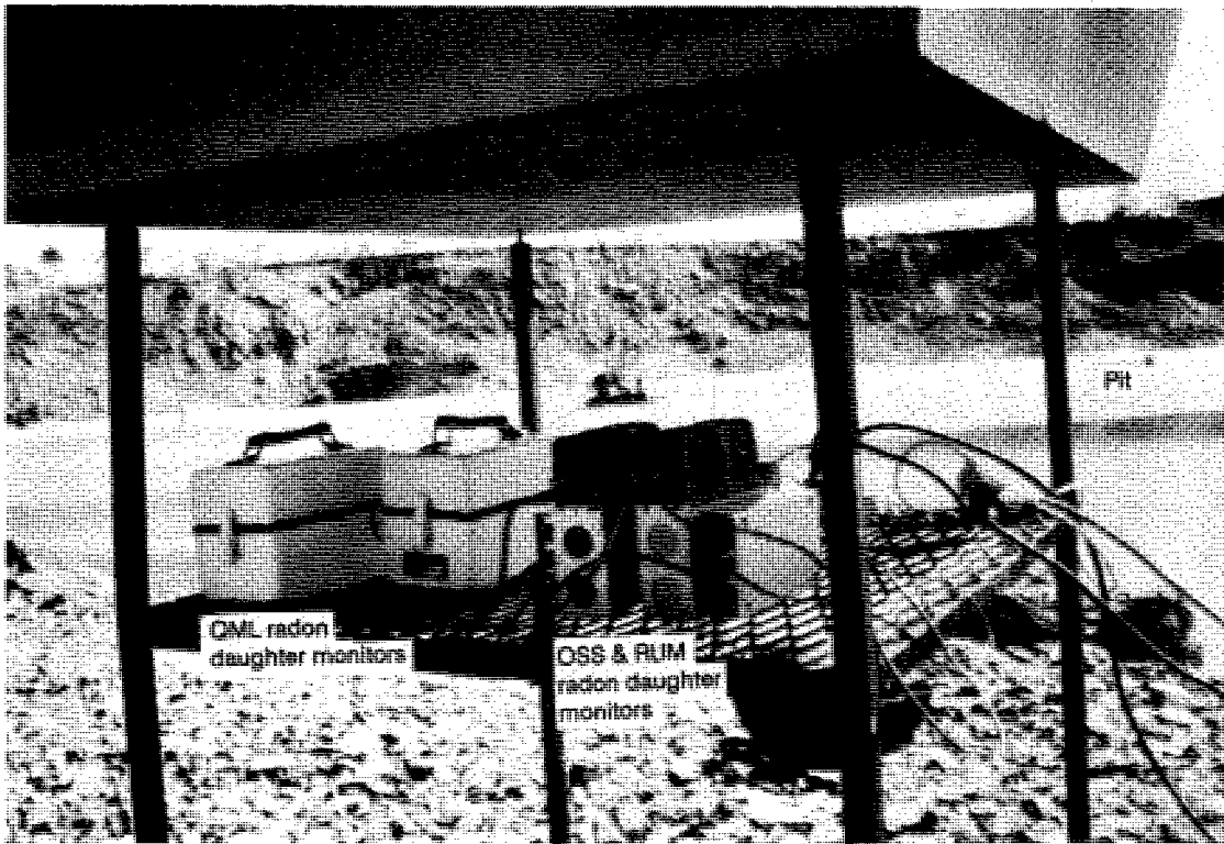
Plate 1. Equipment used in the radon/radon daughter monitor intercomparison, September 1986
