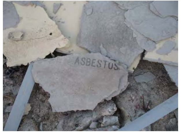
Figure 85. Asbestos sheeting near water at West Island transfer station Jan 2010
