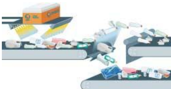
Figure 13 Diagram showing how an optical sorting unit scans and separates materials
