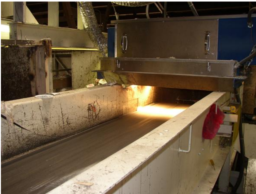
Figure 12 An optical sorting unit above a conveyor 91
