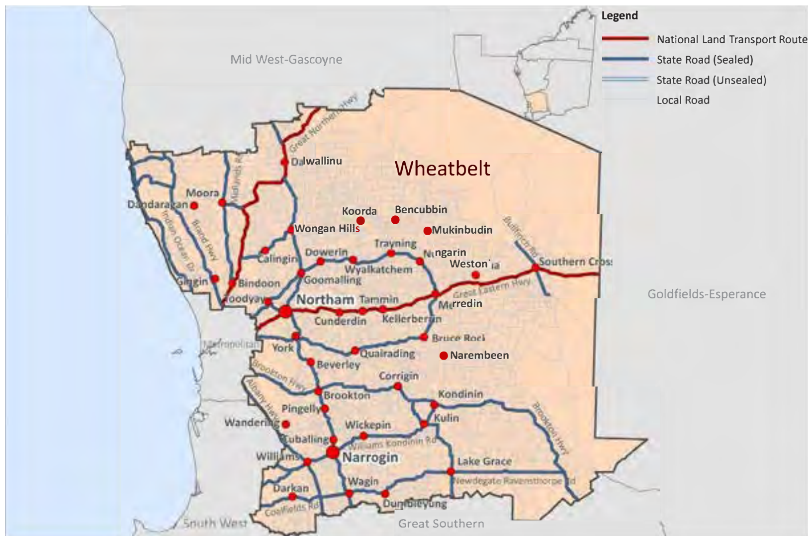
FIGURE 6 National, state and local road network in the Wheatbelt. The region's 42 local government authorities are responsible for maintaining 90% of the network (about 37,000 km).
