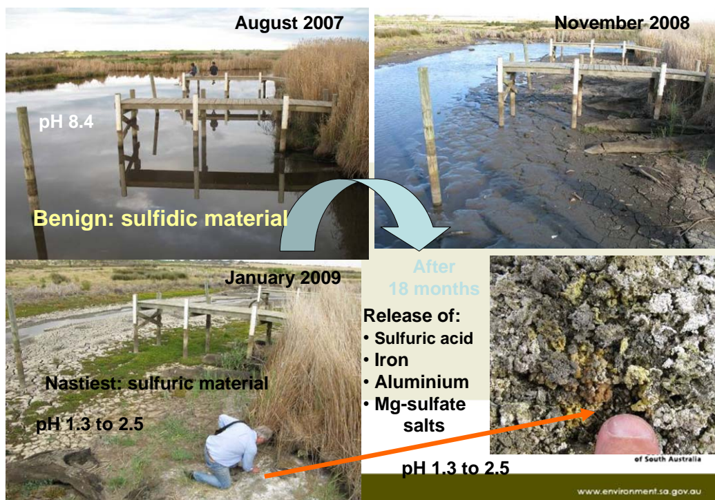
Progression of acid sulfate soils in Lower Lakes (Source: Russell Seaman, DEH SA).
