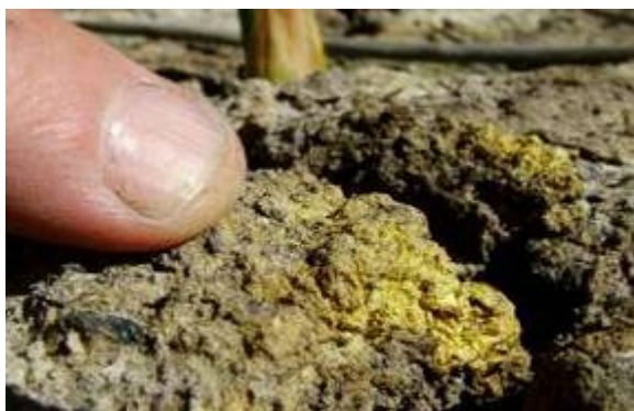
ASS with accumulation of white & yellow Na-Mg-Fe-Al-sulfate-rich minerals; pH 2.5 (Source: CSIRO).
